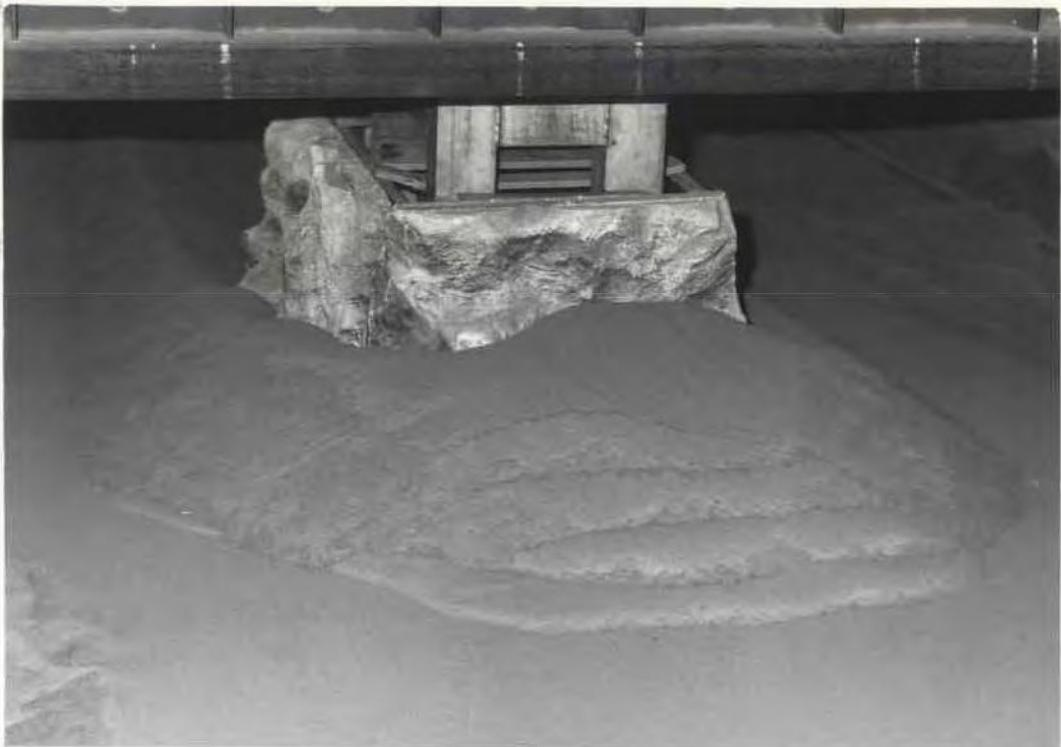
FIGURE 28I MODEL WITH A RANDOM SHAPE (NOTE THE FAILURE WEDGES, SIMILAR TO THOSE FOR THE RECTANGULAR SHAPE)
