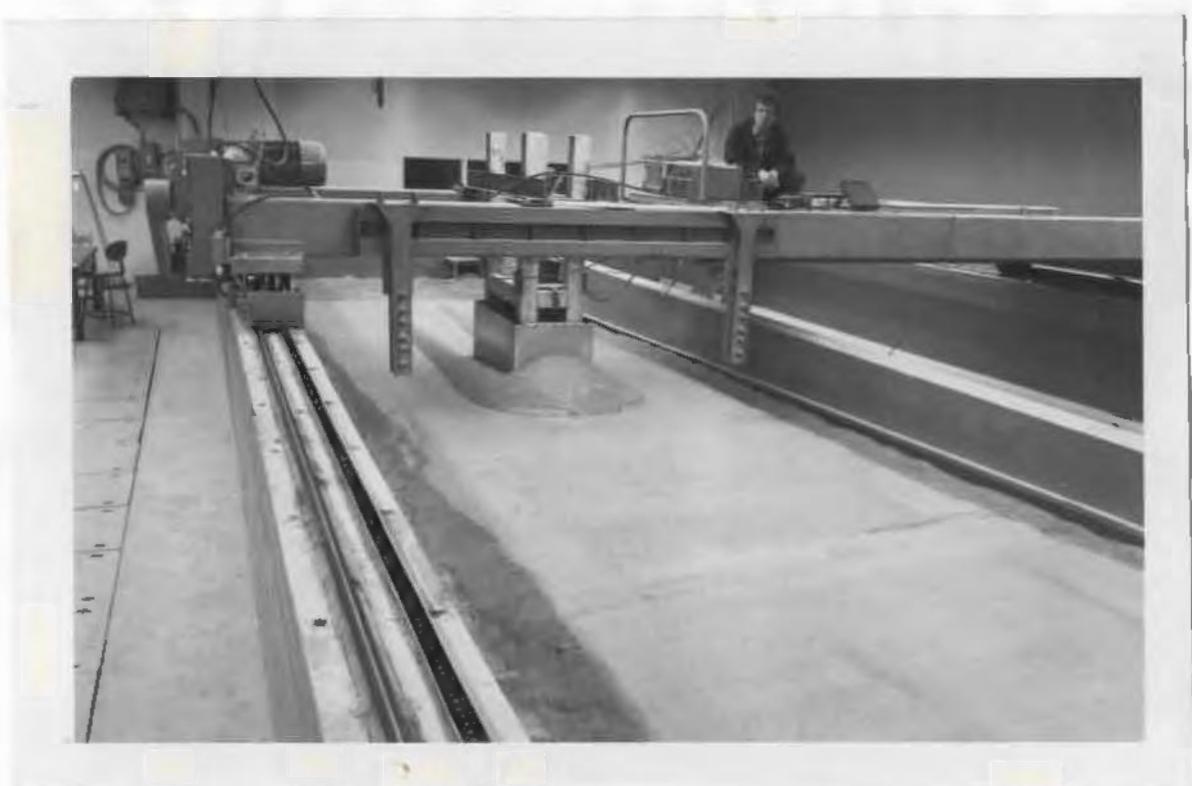
FIGURE 26 A GENERAL VIEW OF THE TOWING TANK, CARRIAGE AND MODEL
