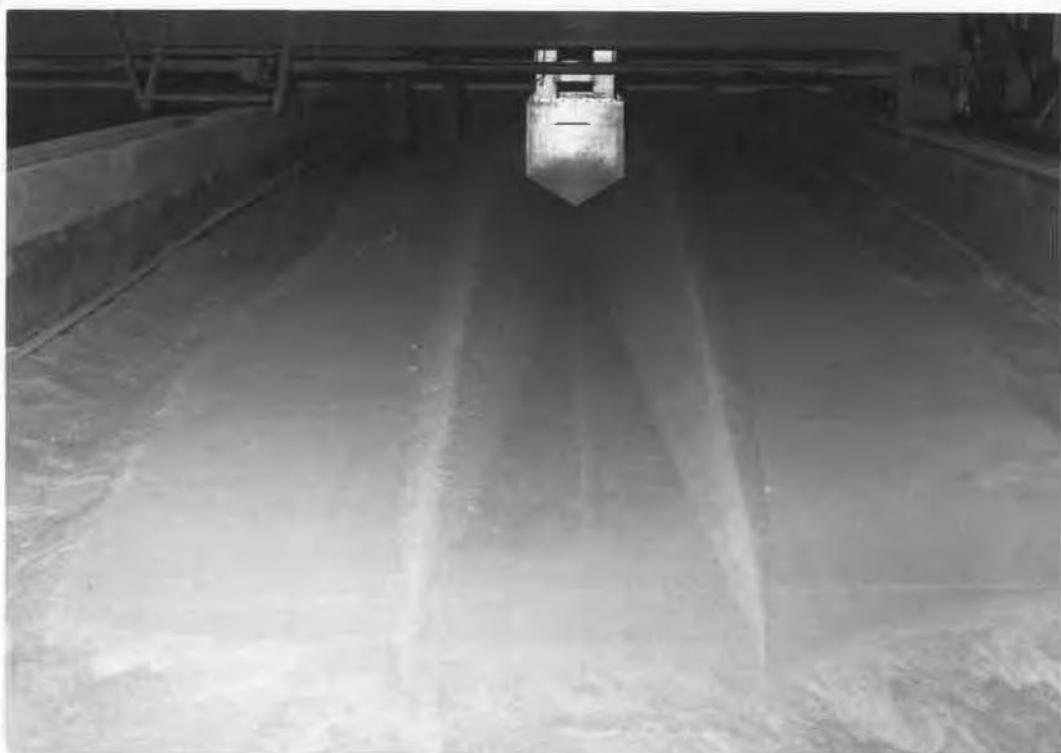
FIGURE 28J SHAPE OF THE SCOUR TRENCH AND RAISED SHOULDERS
