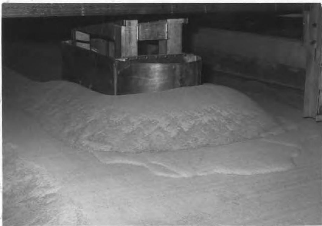
FIGURE 28F MODEL WITH A CYCLINDRICAL SHAPE DURING SCOURING
