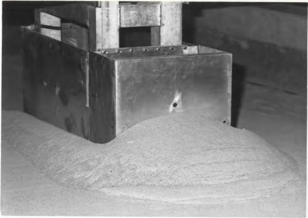
FIGURE 28E MODEL WITH A CURVED KEEL DURING SCOURING
