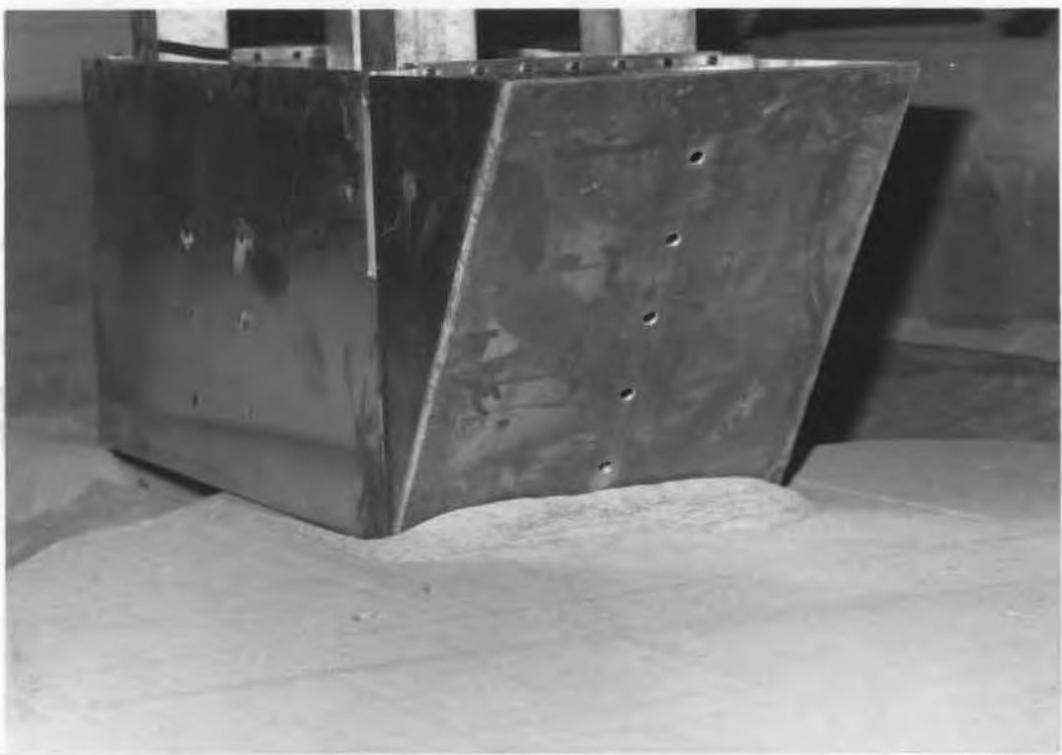
FIGURE 28B MODEL WITH A KEEL SLOPING AT 30°
