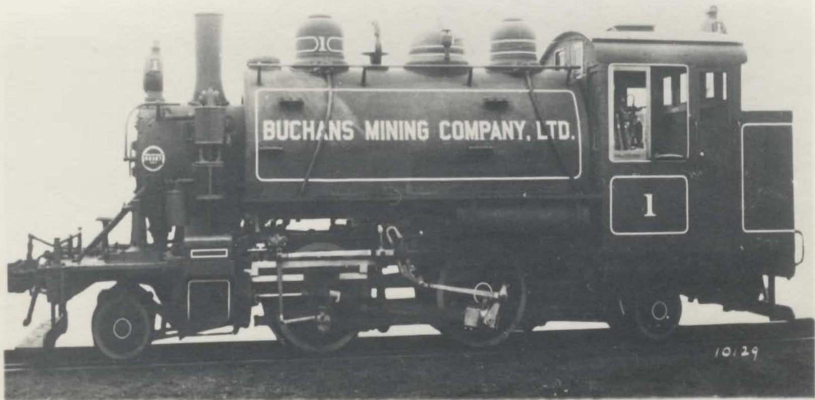
Figure 53. 2-4-2 Buchans Mining Company, Ltd. steam locomotive, No. 1. This locomotive hauled trains of short ore hopper cars to Millertown Junction on the main line from which the ore was taken to the coast for export by ship. The Buchans Mining Company also owned another steam locomotive, No. 2, which was used on the Buchans Railway until 1953 when it was taken to Grand Falls and retirement. In 1949 and in 1952 the Buchans Mining Company bought two diesel-electric locomotives at about the same time the C.N.R. was converting to diesel-electric locomotives. These two diesels were still in operation in the late 1970's.
