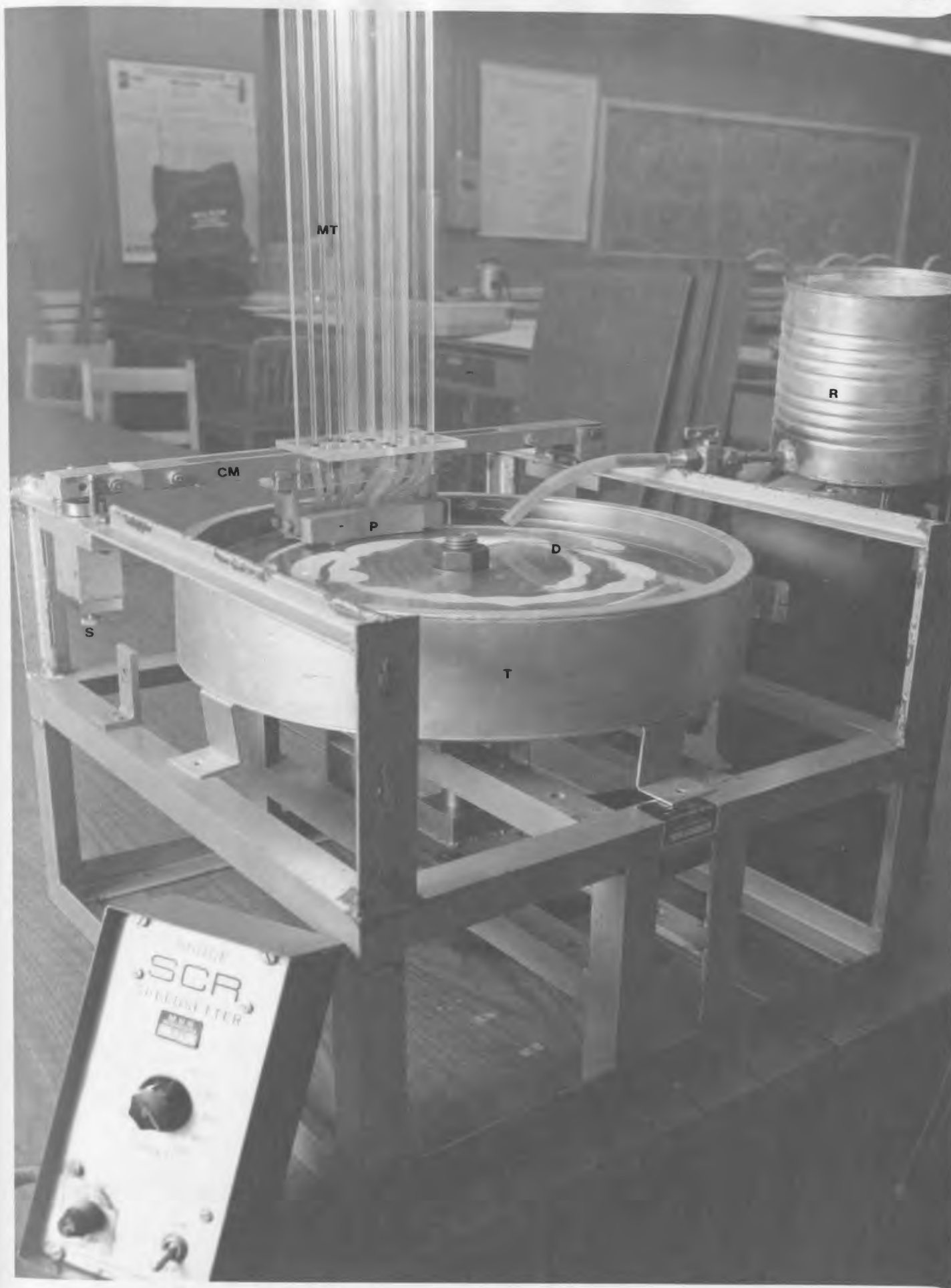
Figure 16 Hydrodynamic Lubrication Rig - Pad Bearing
