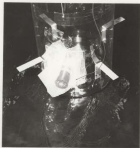
Figure 3.25: The flow pattern around the cylinder before attaching the device
