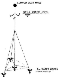
Figure 6.2: The finite element model of the structure
