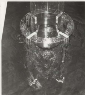
Figure 3.26: The flow pattern around the cylinder after attaching the device
