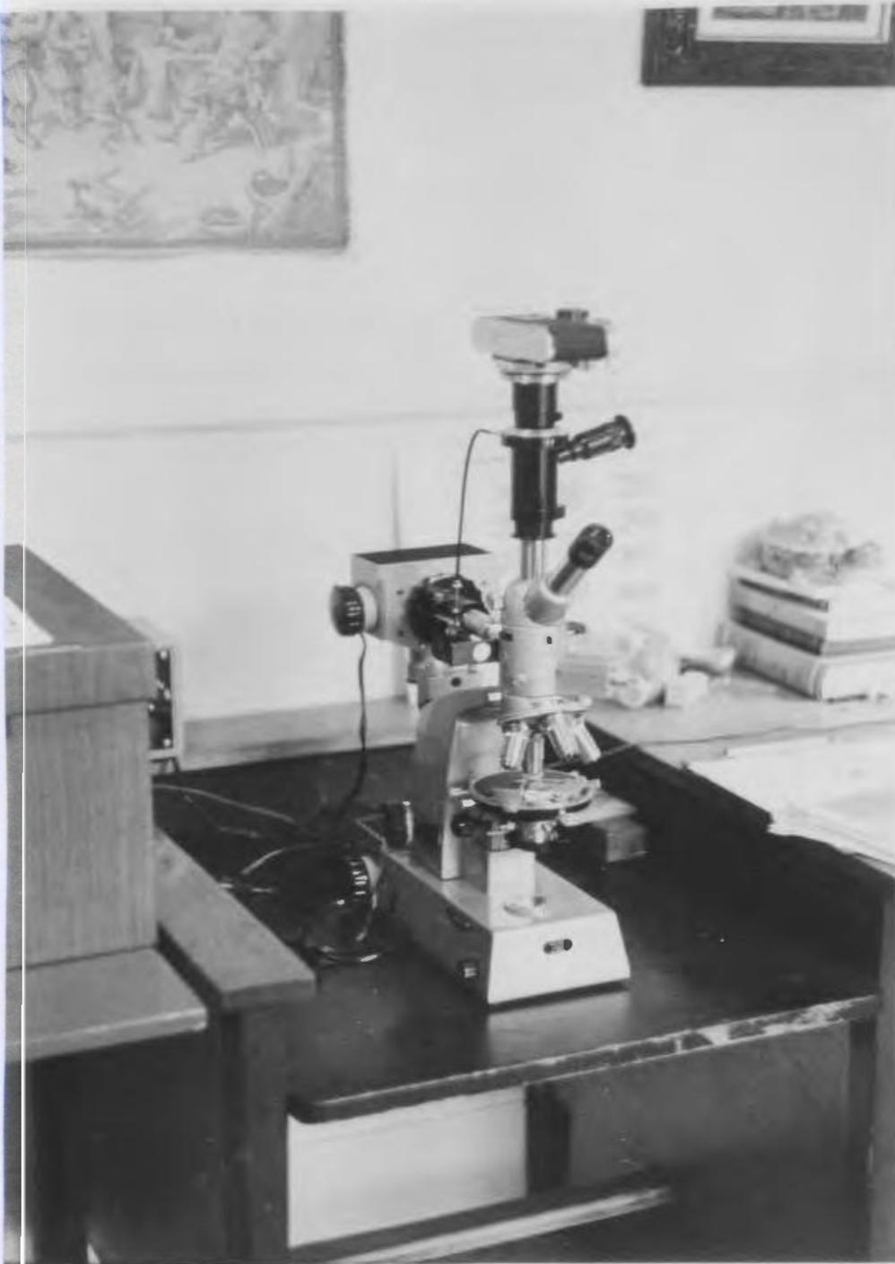
Fig. 6: Reichert microscope fitted with reflected-light interference contrast and photographic attachments.
