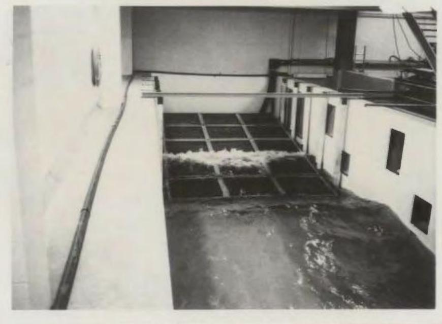
Fig. 5: Wave Absorbing Beach (Slope 1:6.2)
