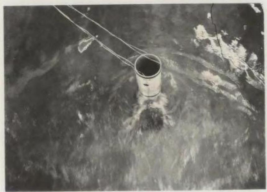
Fig. 17: Vortex Shedding in the Wake of the Circular Cylinder
