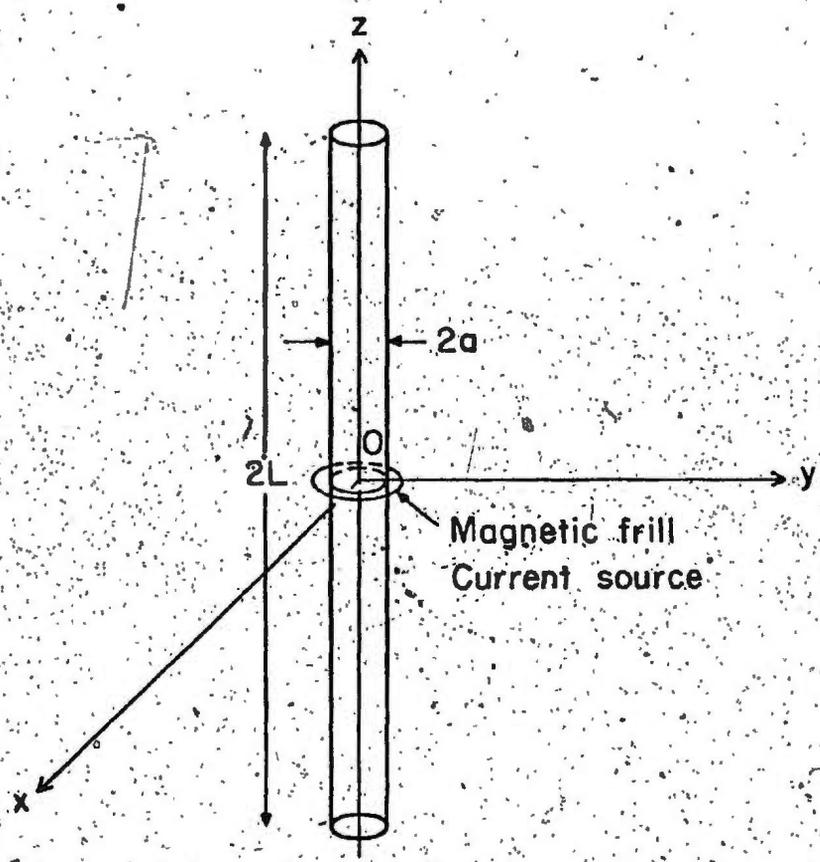
Figure 3.1. Geometry of a symmetrical center-fed linear cylindrical dipole.
