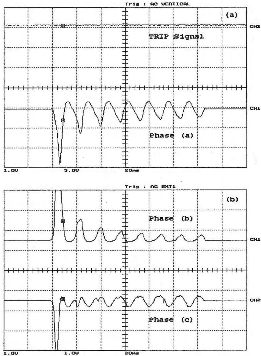
Figure B.3: Magnetizing inrush current for unbalanced resistive load of  $Z_a=20$ ,  $Z_b=\infty$  and  $Z_c=35 \Omega$ , (a) the WPT response and phase (a) differential current, (b) phase (b) and phase (c) differential currents. Y-scale is 1 Div. = 11.67 A
