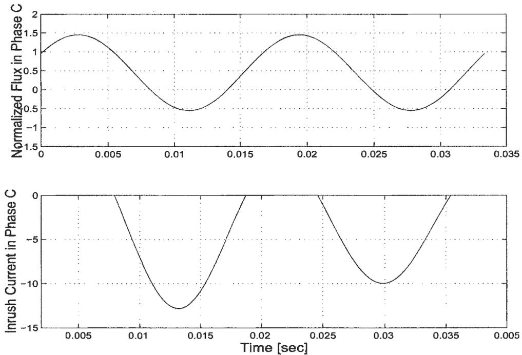
Figure 2.6: Magnetic Flux and Exciting in Phase (c)
