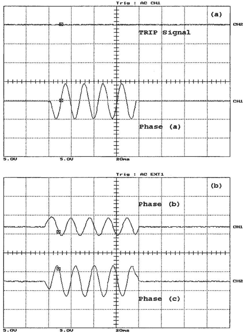
Figure A.4: Magnetizing inrush current for inductive unbalanced load of  $Z_a=j11.9129$ ,  $Z_b= 20+j11.9129 \Omega$  and  $Z_c=20 \Omega/\text{phase}$ , (a) the WPT response and phase (a) differential current, (b) phase (b) and phase (c) differential currents. Y-scale is 1 Div. = 11.67 A
