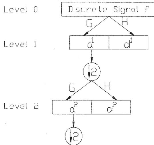
Figure 3.4: Decomposition of The signal  $f[n]$  by DWT
