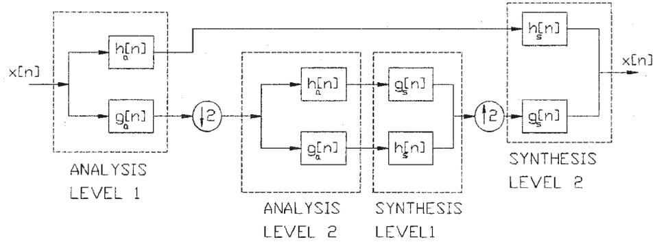
Figure 3.6: Two Level Typical Analysis-Synthesis Quadrature Mirror Filter Bank
