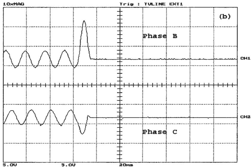
Figure 5.25: Unbalanced loaded phase B to phase C fault, occurred after energization on the secondary side, (a) the WPT response and phase A differential current, (b) phase B and phase C differential currents. Y-scale is 1 Div. = 11.67 A
