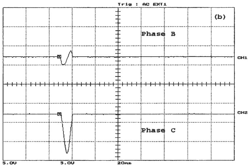
Figure 6.20: Unloaded three-phase to ground fault, occurred before energization on the primary side, (a) the WPT response and phase A differential current, (b) phase B and phase C differential currents. Y-scale is 1 Div. = 11.67 A
