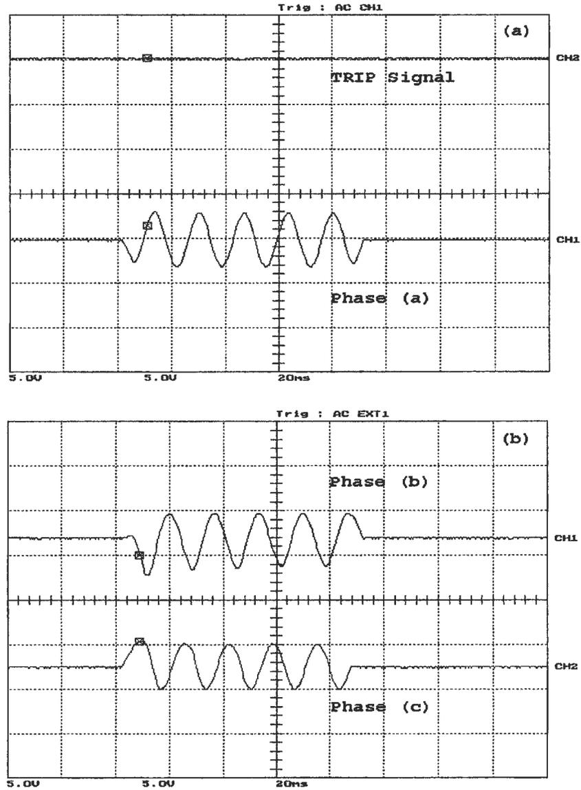
Figure A.3: Magnetizing inrush current for inductive balanced load of  $Z=20+j11.9129 \Omega/\text{phase}$ , (a) the WPT response and phase (a) differential current, (b) phase (b) and phase (c) differential currents. Y-scale is 1 Div. = 11.67 A
