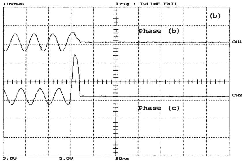
Figure A.33: Loaded phase (a) to phase C fault, occurred after energization on the primary side, (a) the WPT response and phase (a) differential current , (b) phase (b) and phase (c) differential currents. Y-scale is 1 Div. = 11.67 A
