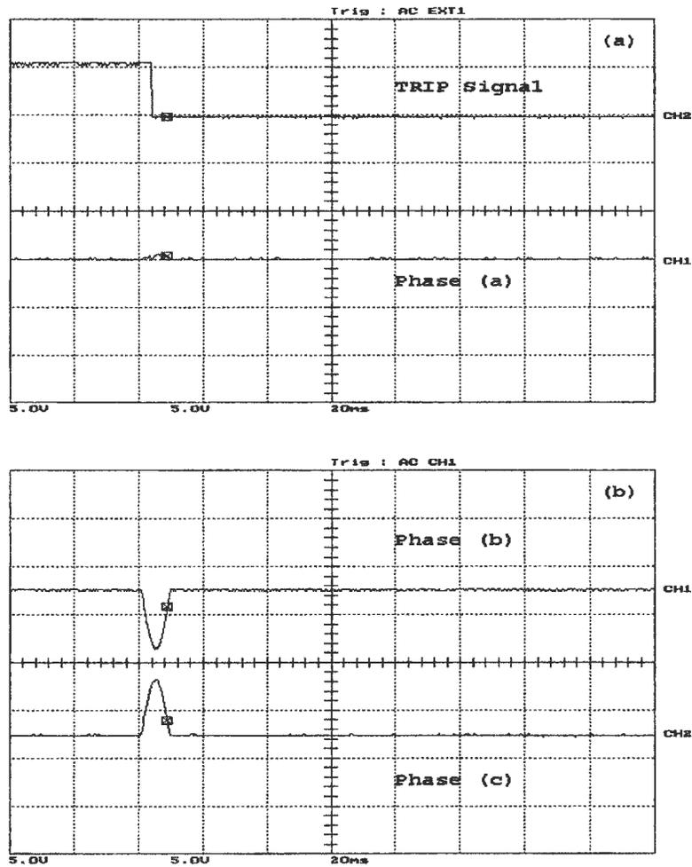
Figure A.37: Unloaded three-phase to ground fault, occurred before energization on the secondary side, (a) the WPT response and phase (a) differential current , (b) phase (b) and phase (c) differential currents. Y-scale is 1 Div. = 11.67 A
