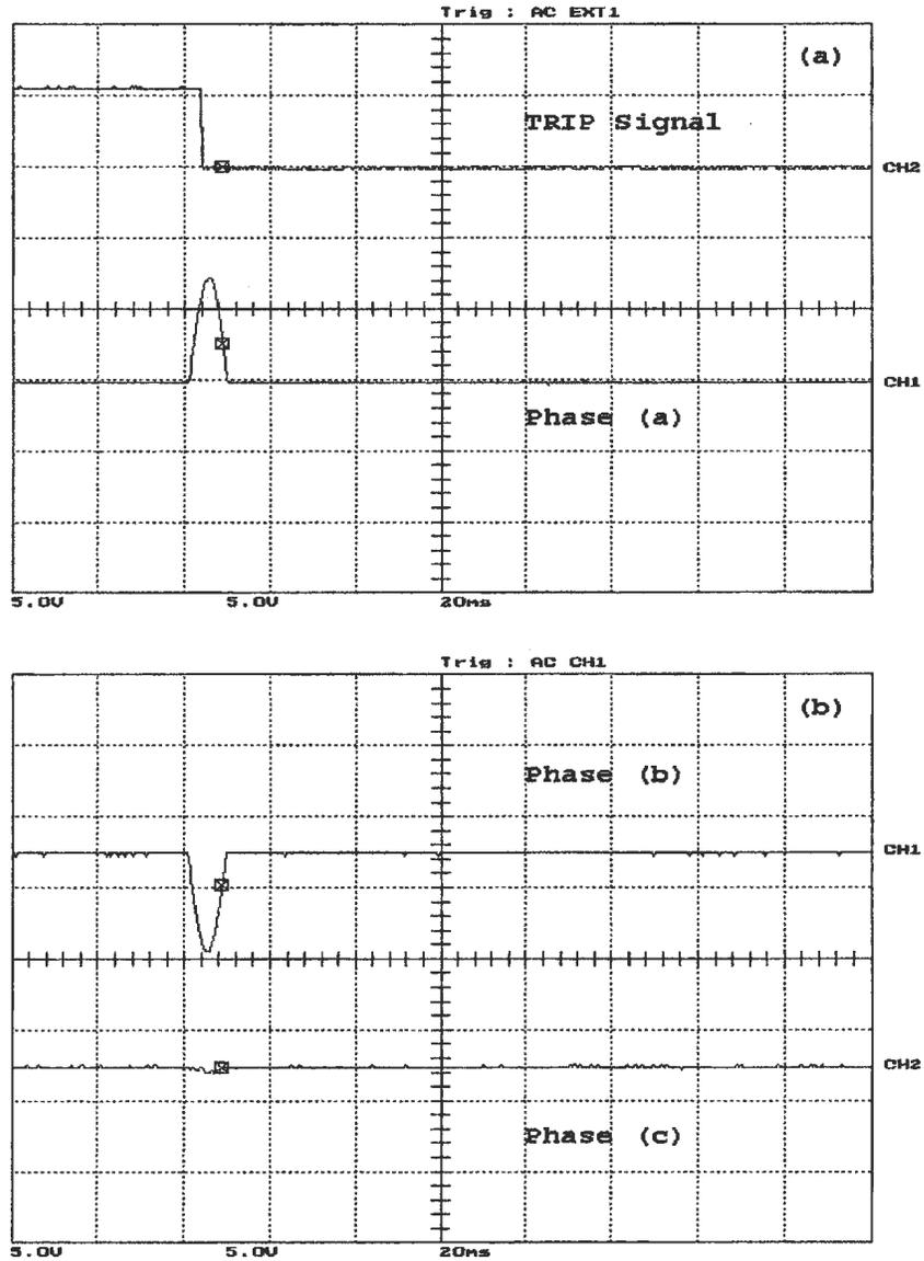
Figure A.40: Loaded three-phase fault, occurred before energization on the secondary side, (a) the WPT response and phase (a) differential current , (b) phase (b) and phase (c) differential currents. Y-scale is 1 Div. = 11.67 A
