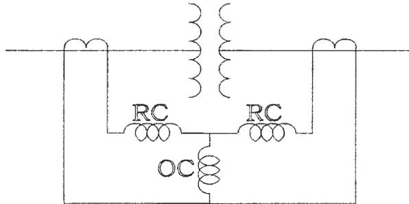
Figure 2.8: A percentage Differential Relay with Restraining Coils
