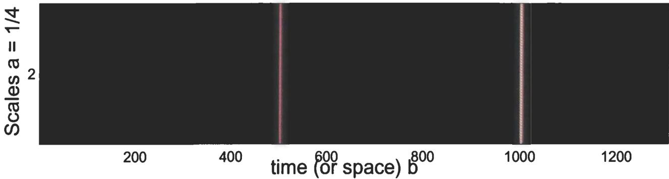
Figure 4.7: Two Level Evaluation of the Wavelet Packet Coefficients for the Secondary Side Loaded Phase to Phase Fault Current (Resistive Load) Using (*db4*) Mother Wavelet
