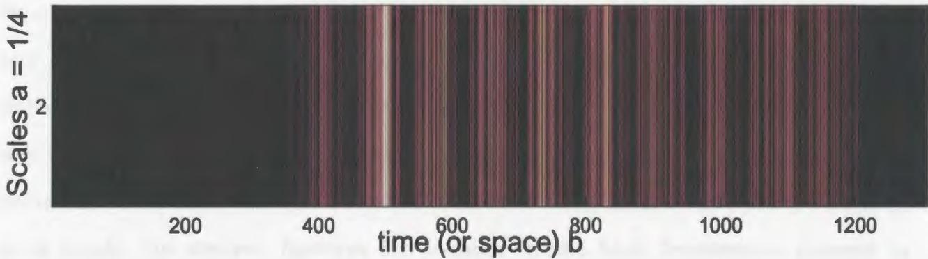
Figure 4.8: Two Level Evaluation of the Wavelet Packet Coefficients for the Primary Side Unloaded Three-Phase to Ground Fault Current Using ( $db4$ ) Mother Wavelet
