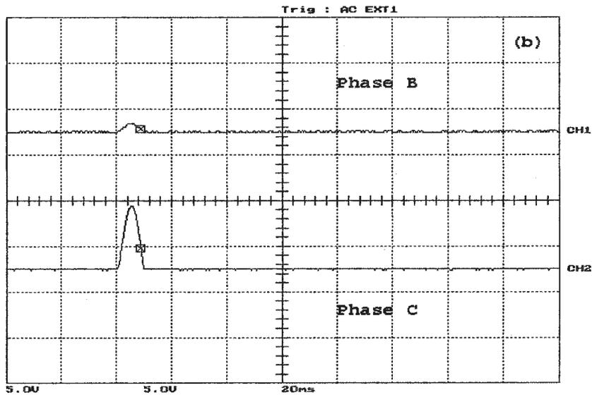
Figure 5.12: Loaded phase A to ground fault, occurred before energization on the secondary side, (a) the WPT response and phase A differential current, (b) phase B and phase C differential currents. Y-scale is 1 Div. = 11.67 A
