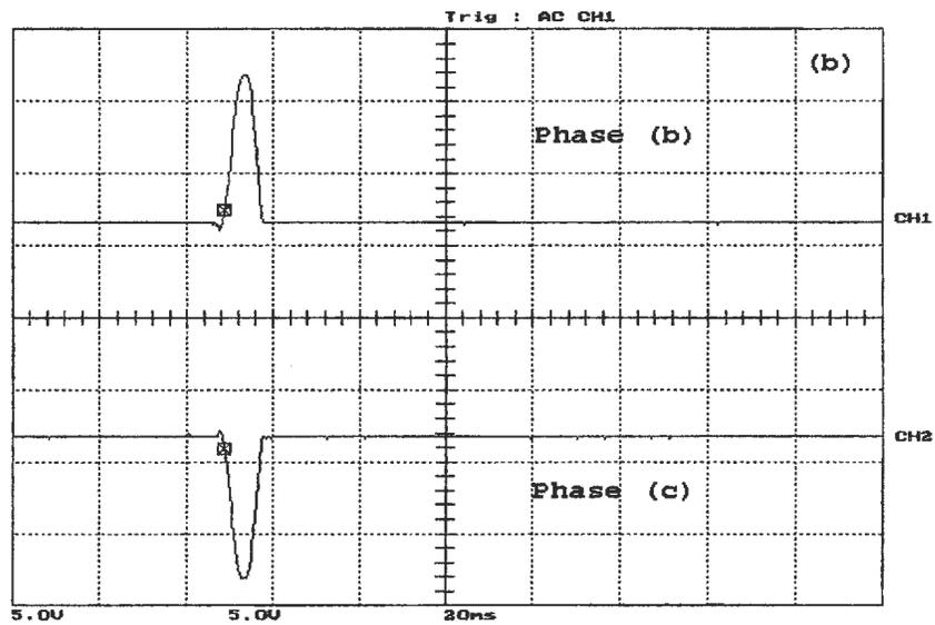
Figure B.26: Unloaded phase (b) to to phase C fault, occurred after energization on the primary side, (a) the WPT response and phase (a) differential current , (b) phase (b) and phase (c) differential currents. Y-scale is 1 Div. = 11.67 A
