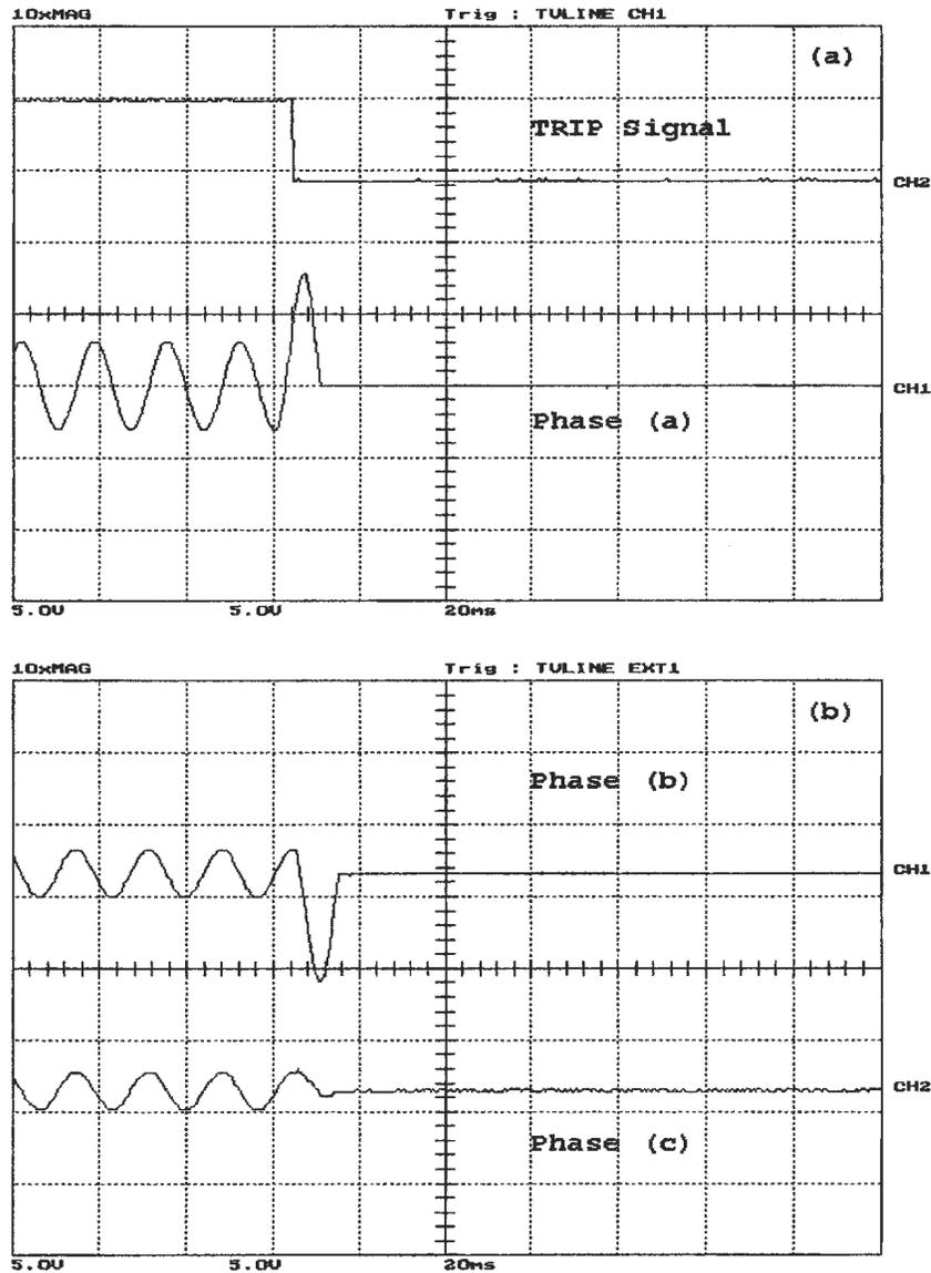
Figure A.47: phase (b) to ground fault, occurred after energization with  $Z_a = 20 + j11.9129$ ,  $Z_b = 11.9129$ ,  $Z_c = \infty \Omega$  on the secondary side, (a) the WPT response and phase (a) differential current, (b) phase (b) and phase (c) differential currents. Y-scale is 1 Div. = 11.67 A
