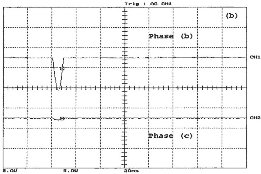
Figure A.14: Loaded phase (b) to ground fault, occurred before energization on the secondary side, (a) the WPT response and phase (a) differential current, (b) phase (b) and phase (c) differential currents. Y-scale is 1 Div. = 11.67 A
