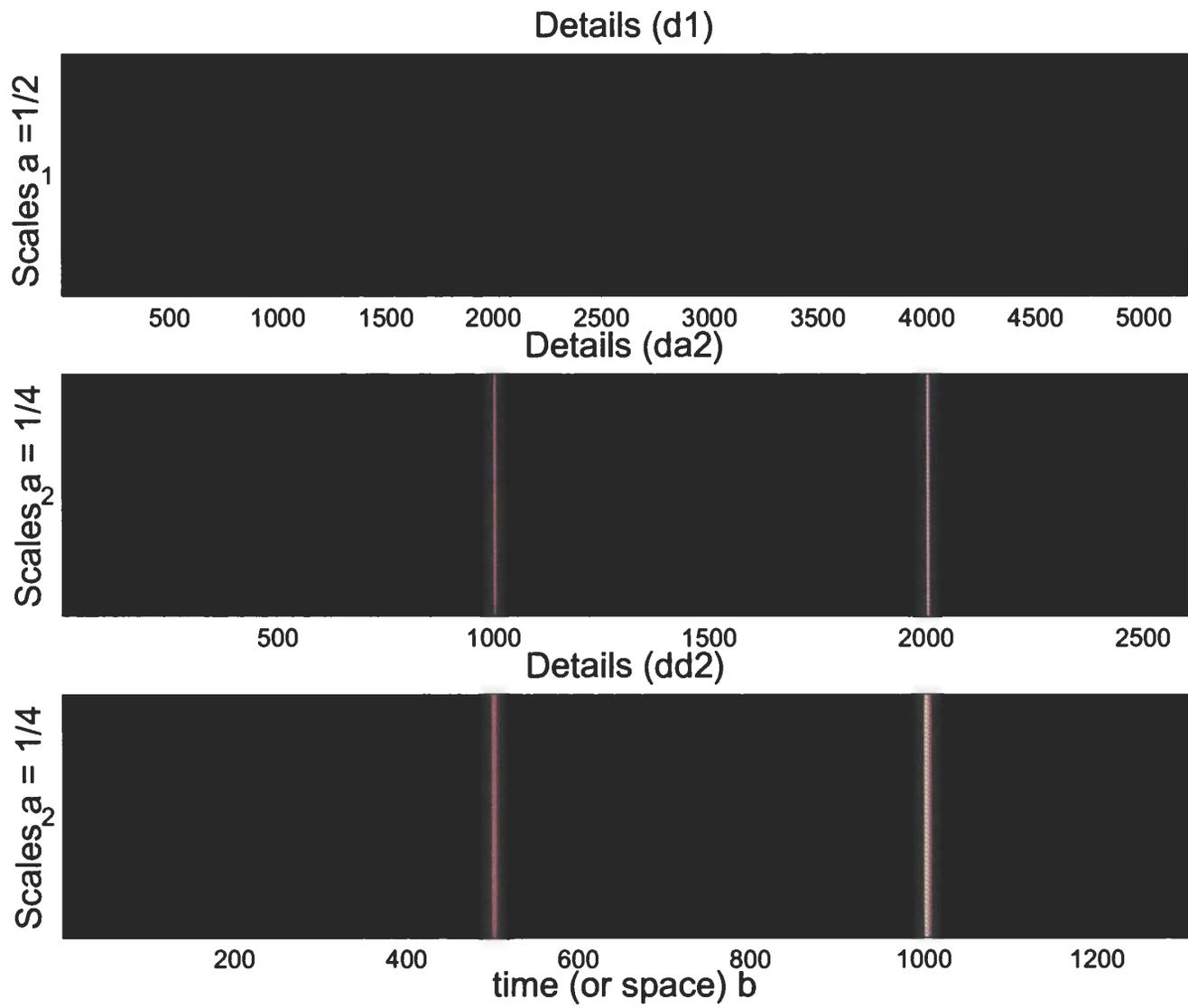
Figure 4.6: Two Level Evaluation of the Wavelet Packet Coefficients for the Primary Side Phase to Phase Fault Current Using (*db4*) Mother Wavelet
