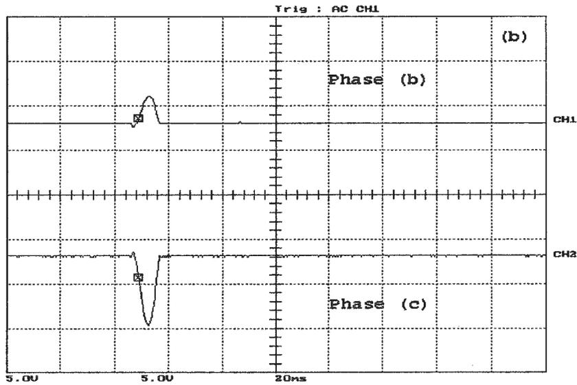
Figure A.15: Loaded phase C to ground fault, occurred before energization on the primary side, (a) the WPT response and phase (a) differential current , (b) phase (b) and phase (c) differential currents. Y-scale is 1 Div. = 11.67 A
