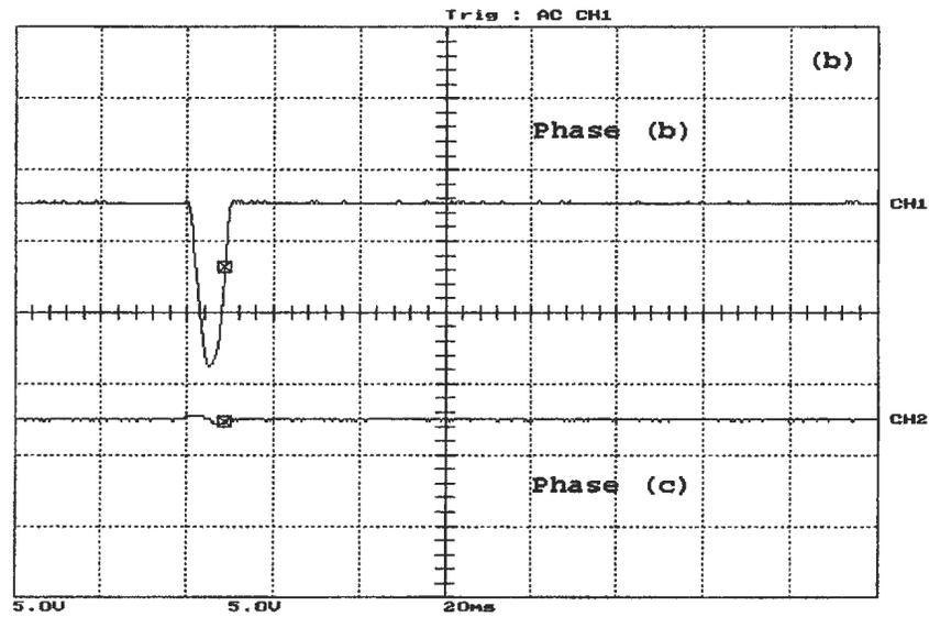
Figure B.28: Loaded phase (a) to phase (b) fault, occurred before energization on the primary side, (a) the WPT response and phase (a) differential current , (b) phase (b) and phase (c) differential currents. Y-scale is 1 Div. = 11.67 A
