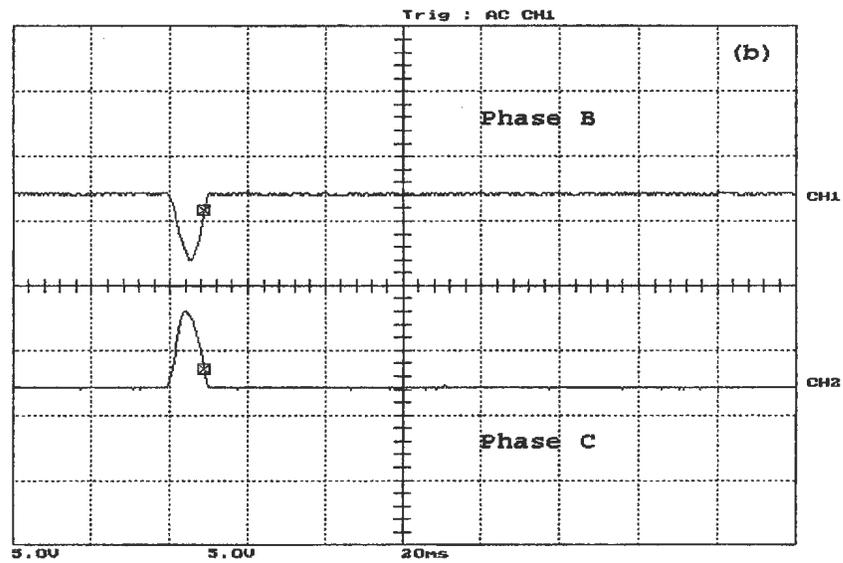
Figure 6.10: Unloaded phase B to ground fault, occurred before energization on the secondary side, (a) the WPT response and phase A differential current, (b) phase B and phase C differential currents. Y-scale is 1 Div. = 11.67 A
