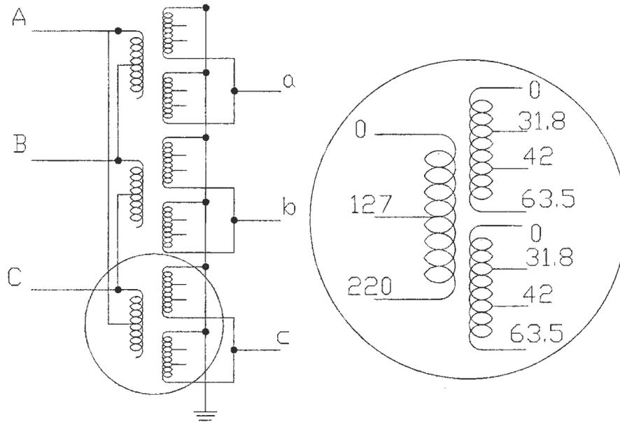
Figure 6.1: The configuration of the step down,  $\Delta$ -Y, 2kVA, 127-220/31.8-42-63.5 V, 50Hz, multi-tap three-phase power transformer
