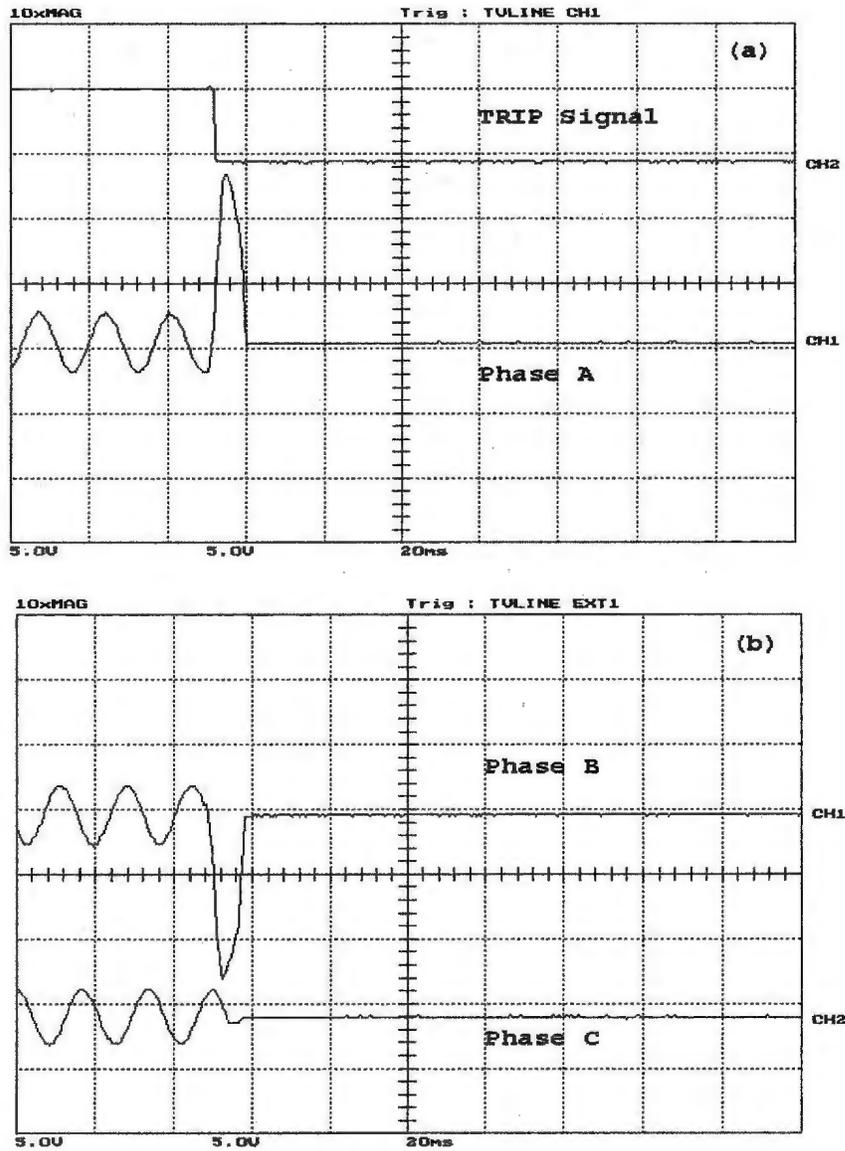
Figure 5.17: Loaded phase A to phase B fault, occurred after energization on the primary side, (a) the WPT response and phase A differential current,(b) phase B and phase C differential currents. Y-scale is 1 Div. = 11.67 A
