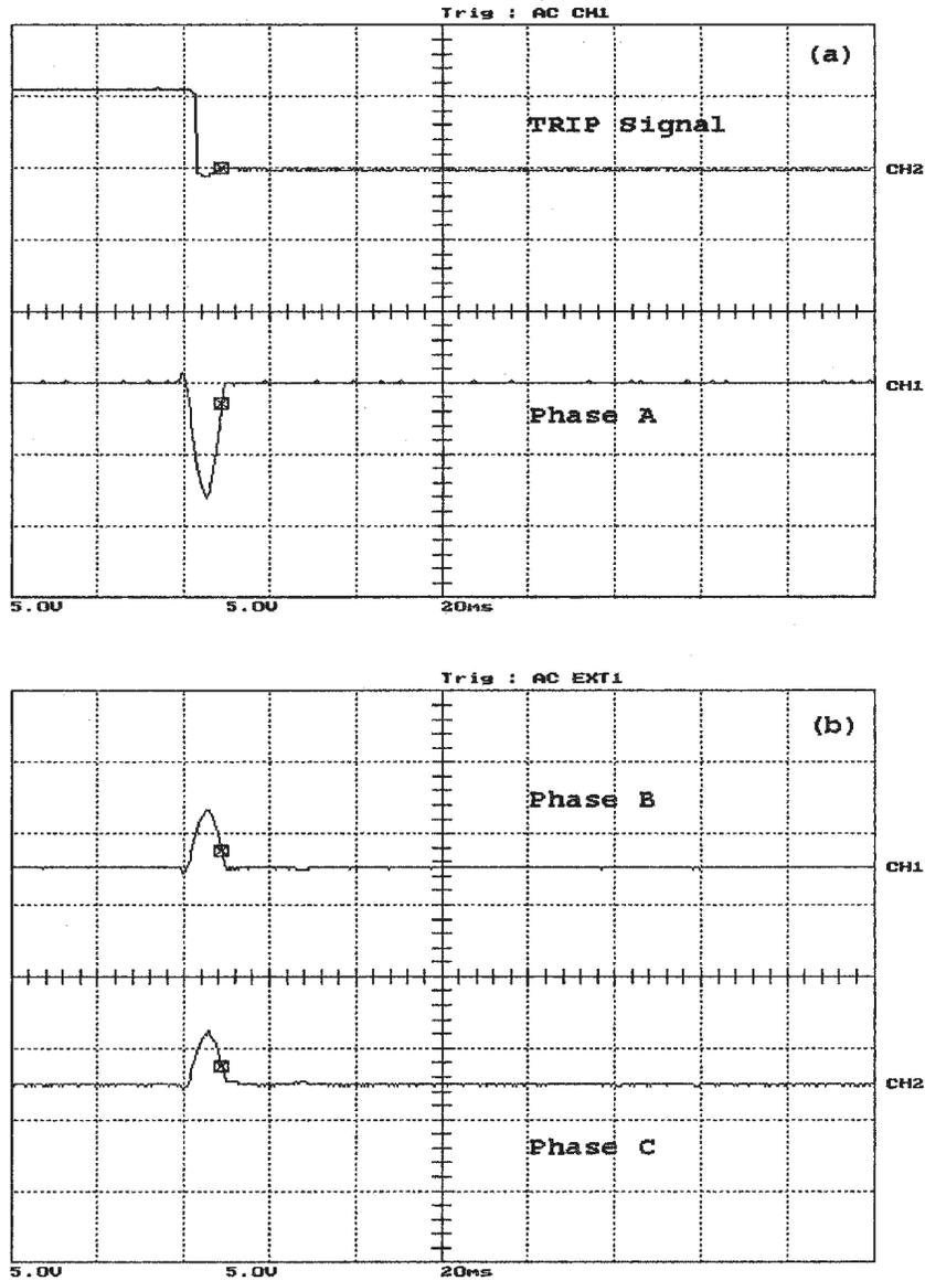
Figure 5.6: Unloaded phase A to ground fault, occurred before energization on the primary side, (a) the WPT response and phase A differential current,(b) phase B and phase C differential currents. Y-scale is 1 Div. = 11.67 A.
