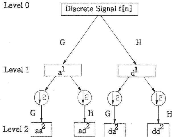
Figure 3.5: Decomposition of the signal  $f[n]$  by WPT
