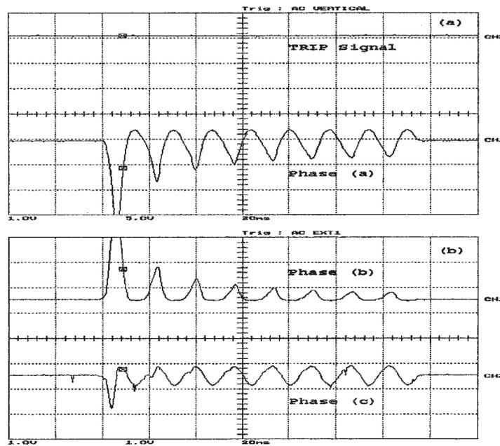
Figure B.1: Magnetizing inrush current for unbalanced inductive load of  $Z_a=20+j11.9129$ ,  $Z_b= j11.9129$  and  $Z_c=20 \Omega$ , (a) the WPT response and phase (a) differential current , (b) phase (b) and phase (c) differential currents. Y-scale is 1 Div. = 11.67 A
