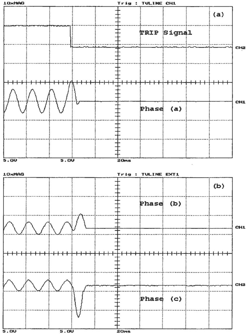
Figure A.46: phase (a) phase C fault, occurred after energization with  $Z_a = 20 + j11.9129$ ,  $Z_b = 11.9129$ ,  $Z_c = \infty \Omega$  on the secondary side, (a) the WPT response and phase (a) differential current, (b) phase (b) and phase (c) differential currents. Y-scale is 1 Div. = 11.67 A
