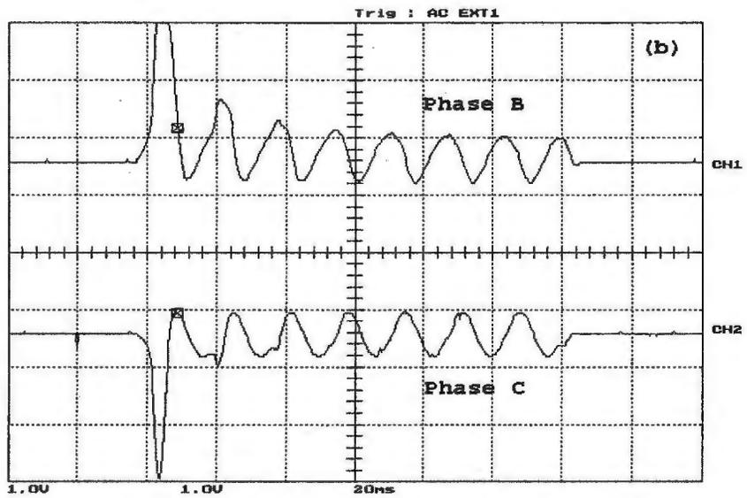
Figure 6.5: Loaded magnetizing inrush current, (a) the WPT response and phase A differential current, (b) phase B and phase C differential currents. Y-scale is 1 Div. = 11.67 A
