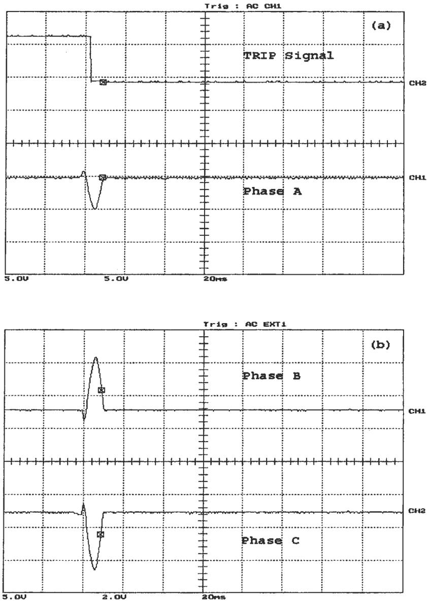
Figure 6.8: Loaded phase B to ground fault, occurred before energization on the primary side, (a) the WPT response and phase A differential current, (b) phase B and phase C differential currents. Y-scale is 1 Div. = 11.67 A
