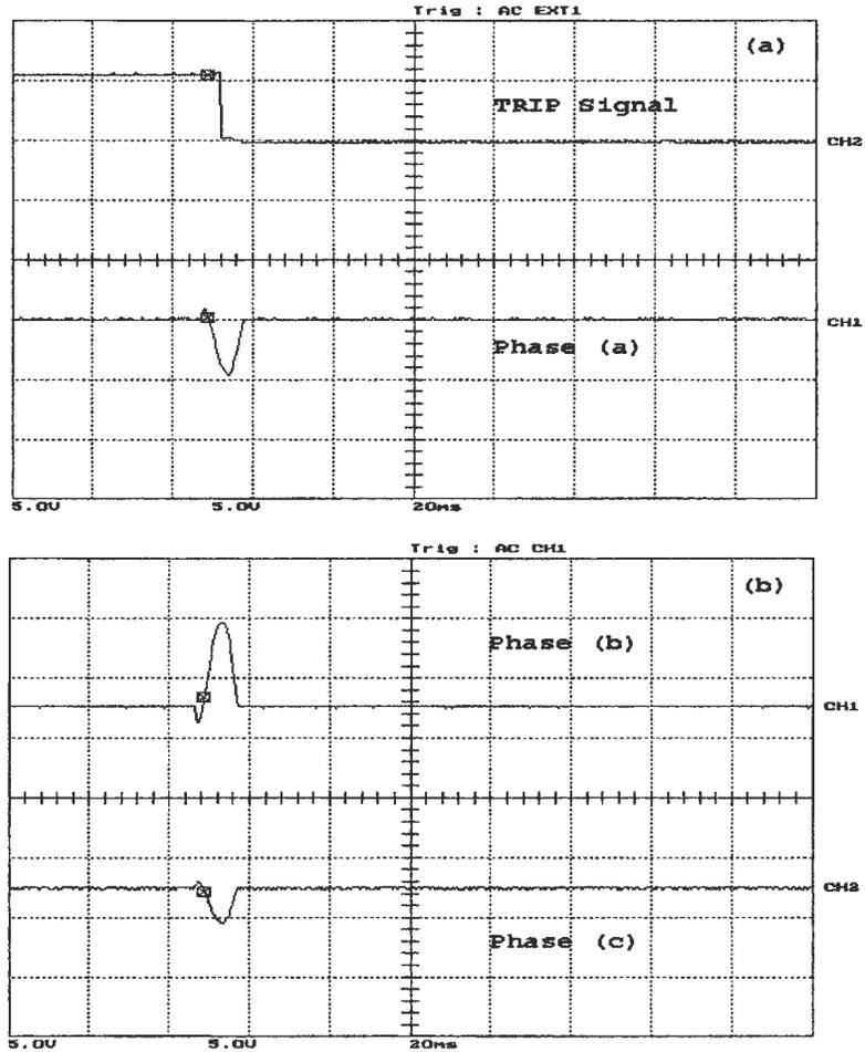
Figure A.5: Unloaded phase (b) to ground fault, occurred before energization on the primary side, (a) the WPT response and phase (a) differential current, (b) phase (b) and phase (c) differential currents. Y-scale is 1 Div. = 11.67 A
