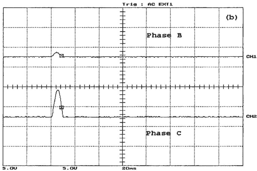
Figure 5.10: Unloaded phase A to ground fault, occurred before energization on the secondary side, (a) the WPT response and phase A differential current,(b) phase B and phase C differential currents. Y-scale is 1 Div. = 11.67 A
