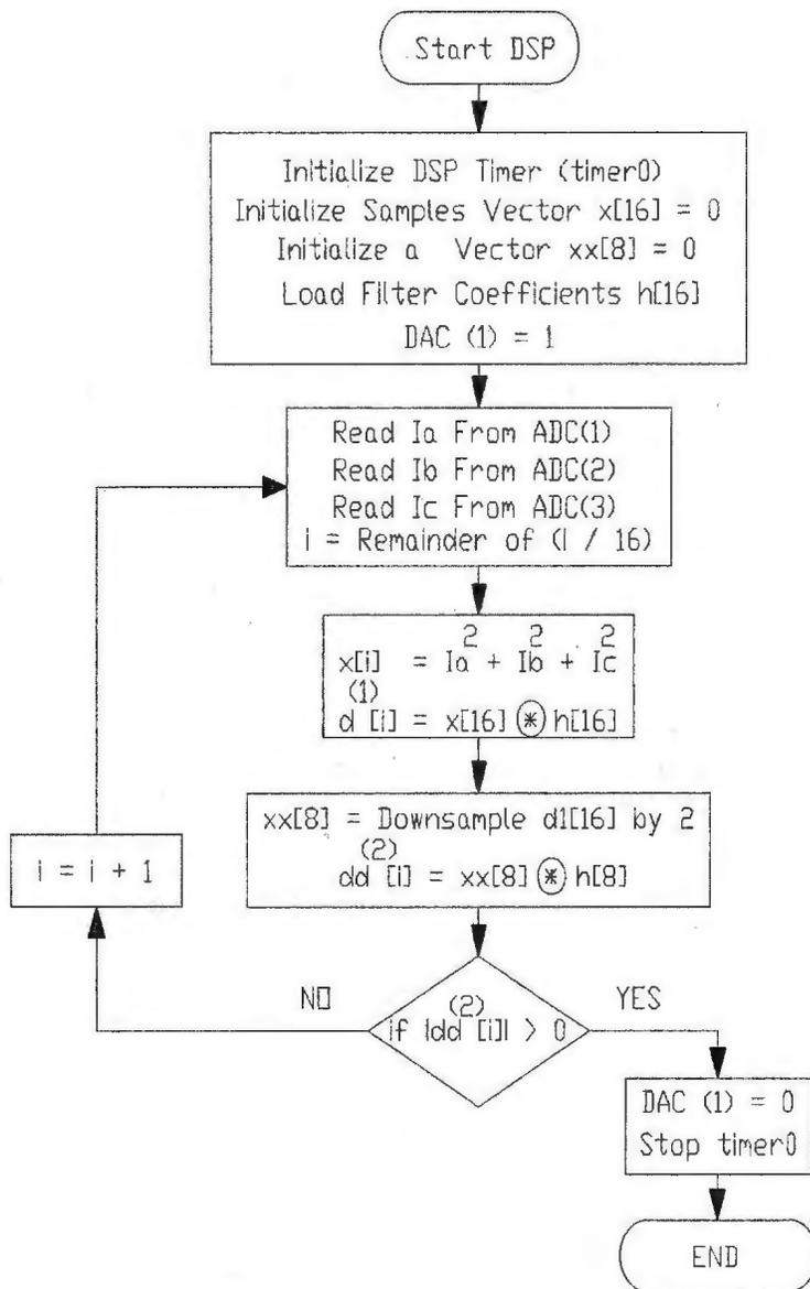
Figure 5.3: Flowchart of Implementing the Wavelet Packet-Based Algorithm
