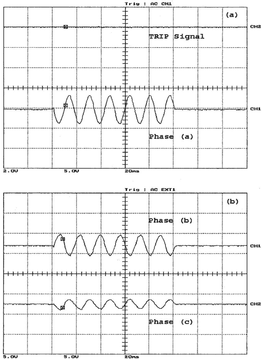
Figure A.2: Magnetizing inrush current for resistive unbalanced load of  $Z_a=\infty$ ,  $Z_b= 20 \Omega$  and  $Z_c=35 \Omega$ /phase, (a) the WPT response and phase (a) differential current , (b) phase (b) and phase (c) differential currents. Y-scale is 1 Div. = 11.67 A
