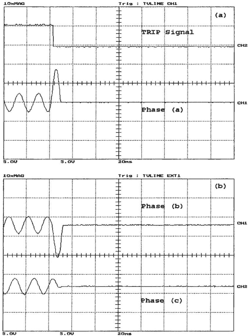
Figure A.18: Loaded phase (b) to ground fault, occurred after energization on the secondary side, (a) the WPT response and phase (a) differential current , (b) phase (b) and phase (c) differential currents. Y-scale is 1 Div. = 11.67 A
