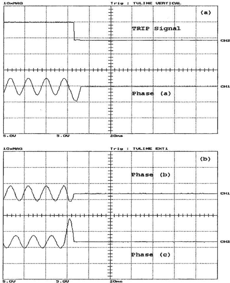
Figure A.43: Phase C to ground fault, occurred after energization with  $Z_a = 20 + j11.9129$ ,  $Z_b = 20 + j0$ ,  $Z_c = 35 + j7.012$   $\Omega$  on the primary side, (a) the WPT response and phase (a) differential current, (b) phase (b) and phase (c) differential currents. Y-scale is 1 Div. = 11.67 A
