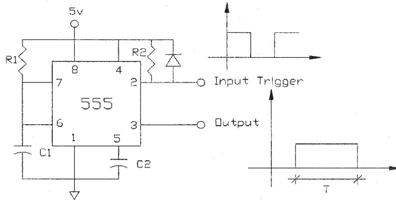
Figure 4.2: The Triggering Circuit Connection,  $R1= 100\text{ k}\Omega$ ,  $C1= 1\ \mu\text{F}$ ,  $R2=10\text{k}\Omega$ ,  $C2=0.01\ \mu\text{F}$  and  $T=1.1R1C1= 0.1\text{ sec}$
