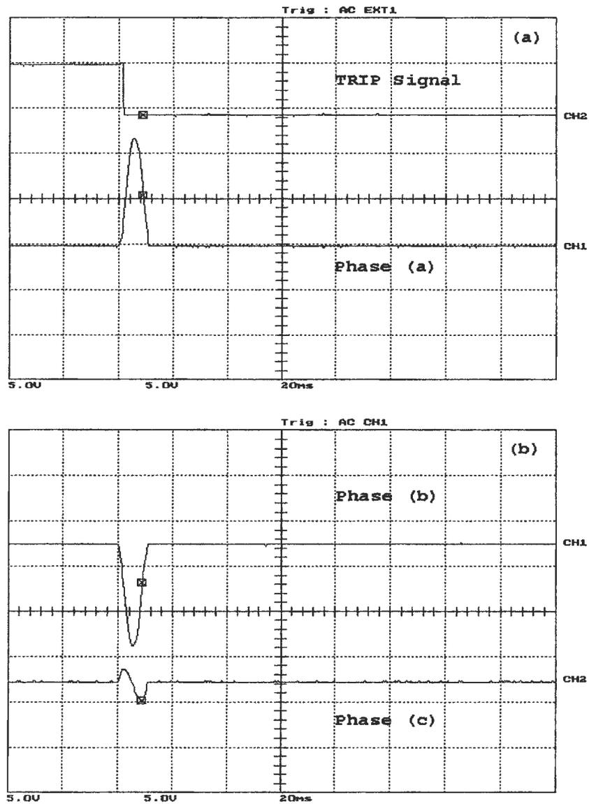
Figure B.38: Loaded three-phase fault, occurred before energization on the primary side, (a) the WPT response and phase (a) differential current, (b) phase (b) and phase (c) differential currents. Y-scale is 1 Div. = 11.67 A
