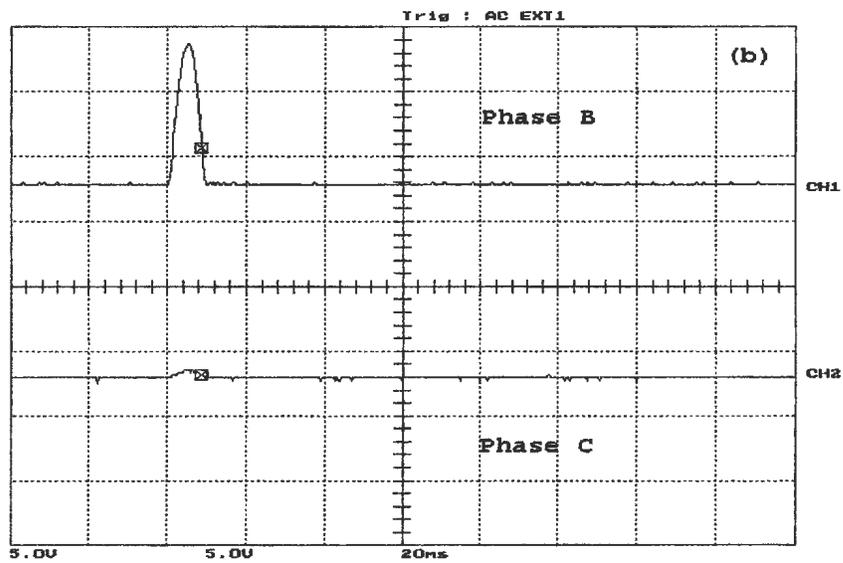
Figure 5.16: Loaded phase A to phase B fault, occurred before energization on the primary side, (a) the WPT response and phase A differential current,(b) phase B and phase C differential currents. Y-scale is 1 Div. = 11.67 A
