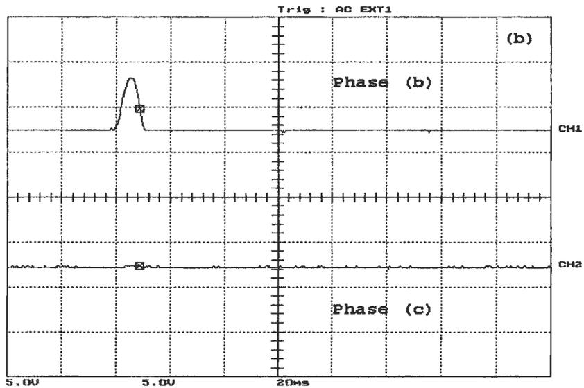
Figure B.13: Loaded phase (a) to ground fault, occurred before energization on the secondary side, (a) the WPT response and phase (a) differential current , (b) phase (b) and phase (c) differential currents. Y-scale is 1 Div. = 11.67 A
