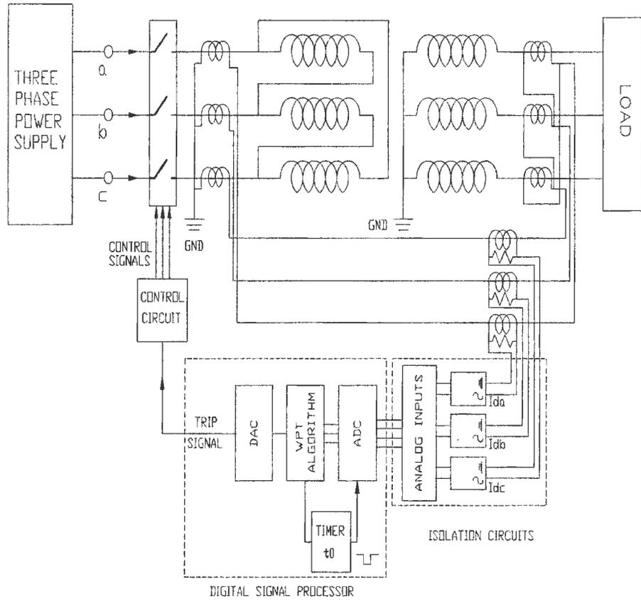
Figure 5.2: Experimental setup for on-line testing on the core type power transformer
