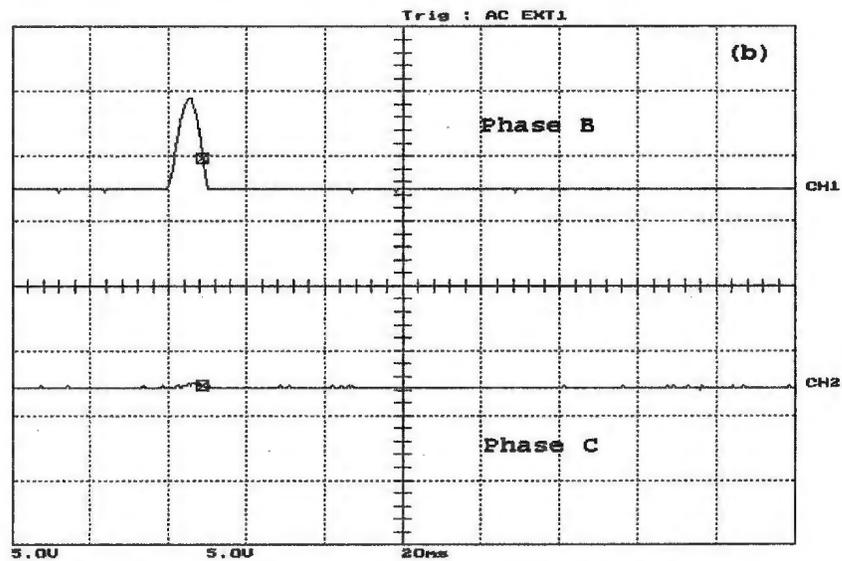
Figure 6.21: Loaded three-phase to ground fault, occurred before energization on the secondary side, (a) the WPT response and phase A differential current, (b) phase B and phase C differential currents. Y-scale is 1 Div. = 11.67 A
