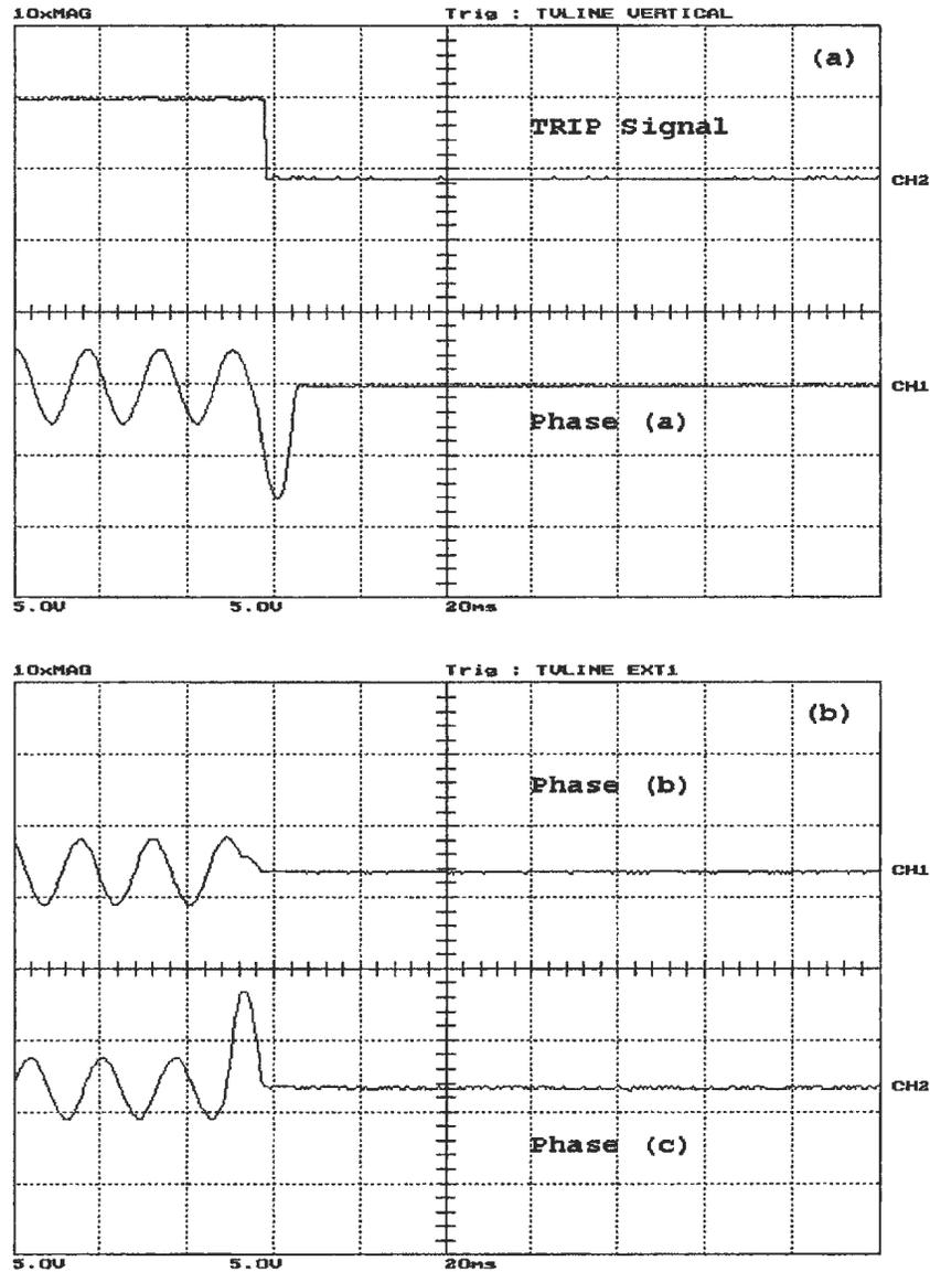
Figure A.44: phase (a) to ground fault, occurred after energization with  $Z_a = 20 + j11.9129$ ,  $Z_b = 20 + j0$ ,  $Z_c = 35 + j7.012$   $\Omega$  on the secondary side, (a) the WPT response and phase (a) differential current, (b) phase (b) and phase (c) differential currents. Y-scale is 1 Div. = 11.67 A
