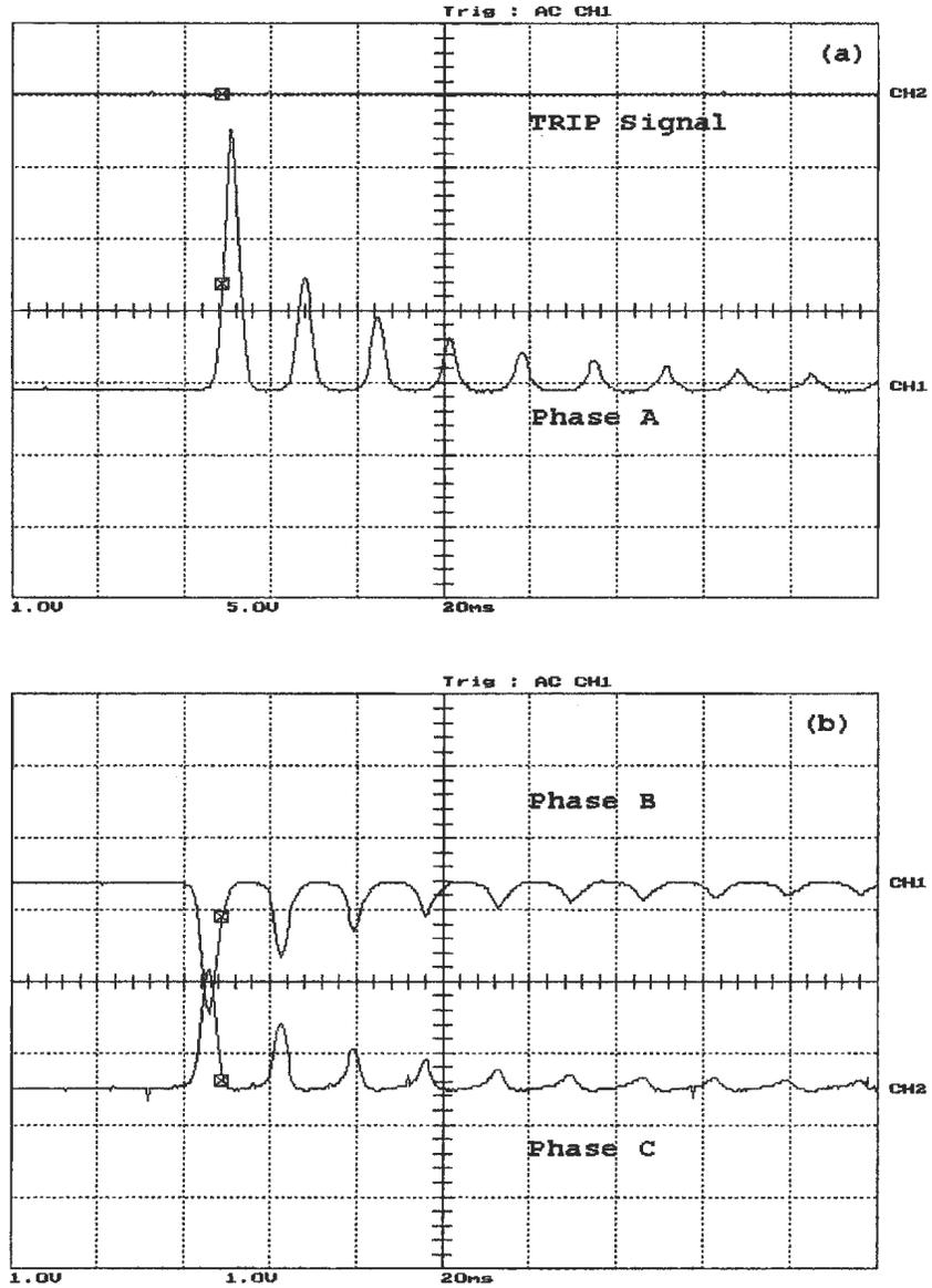
Figure 5.5: Unloaded magnetizing inrush current, (a) the WPT response and phase A differential current, (b) phase B and phase C differential currents. Y-scale is 1 Div. = 11.67 A
