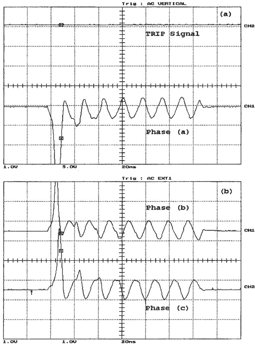
Figure B.2: Magnetizing inrush current for balanced resistive load of  $Z=20 \Omega/\text{phase}$ , (a) the WPT response and phase (a) differential current, (b) phase (b) and phase (c) differential currents. Y-scale is 1 Div. = 11.67 A
