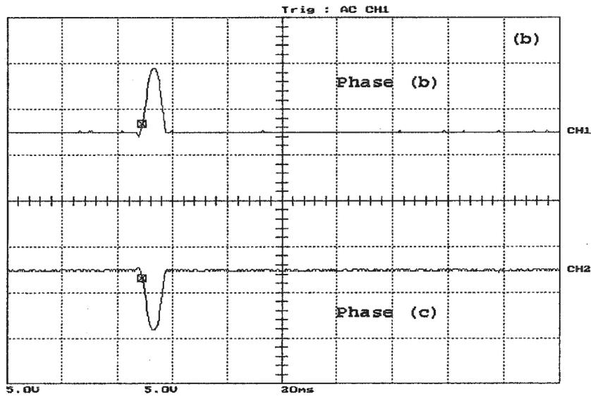
Figure A.16: Loaded phase C to ground fault, occurred before energization on the secondary side, (a) the WPT response and phase (a) differential current , (b) phase (b) and phase (c) differential currents. Y-scale is 1 Div. = 11.67 A
