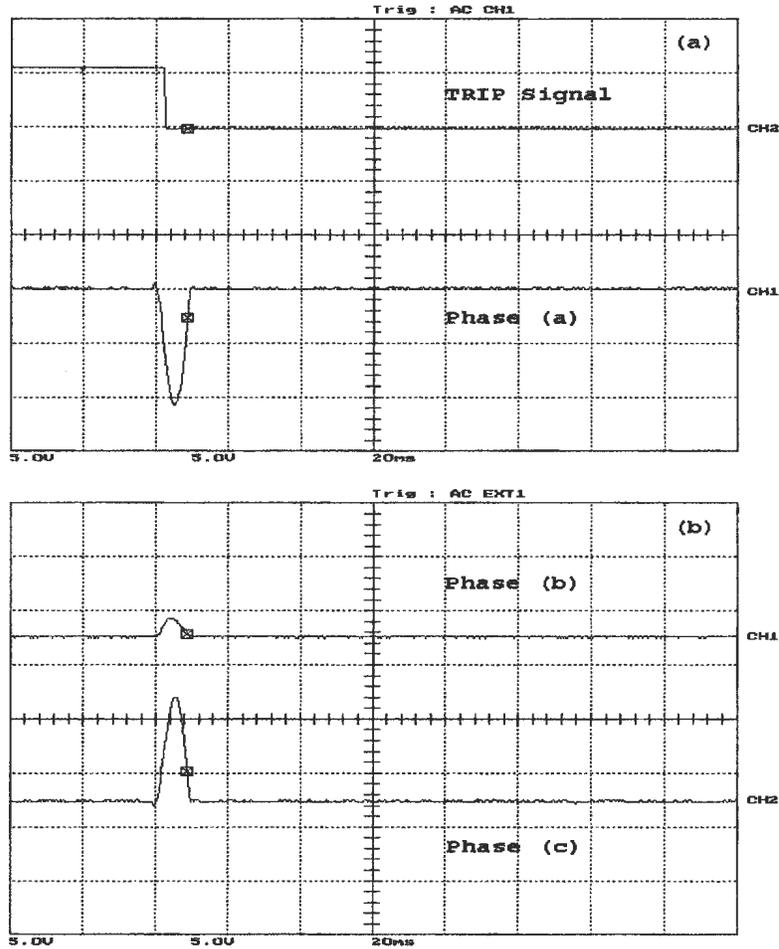
Figure A.21: Unloaded phase (a) to phase C fault, occurred before energization on the primary side, (a) the WPT response and phase (a) differential current, (b) phase (b) and phase (c) differential currents. Y-scale is 1 Div. = 11.67 A
