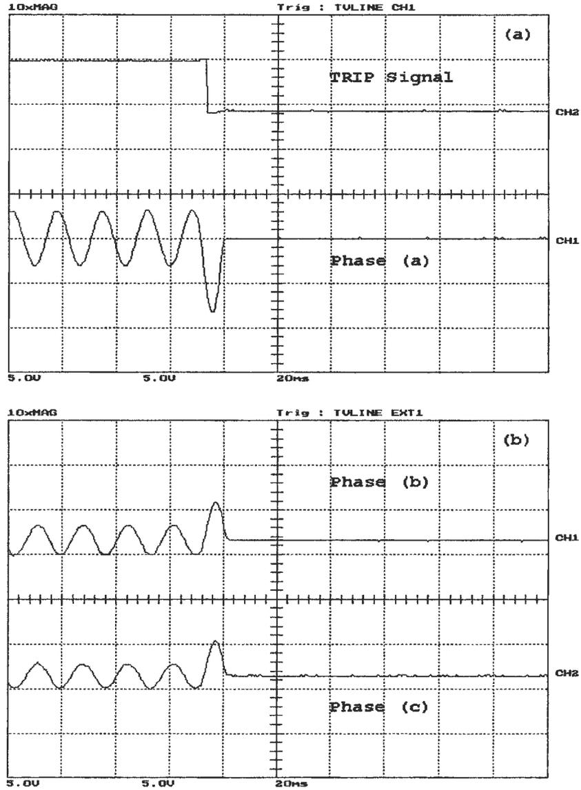
Figure A.45: phase (a) to ground fault, occurred after energization with  $Z_a = 20 + j11.9129$ ,  $Z_b = 11.9129$ ,  $Z_c = \infty \Omega$  on the primary side, (a) the WPT response and phase (a) differential current, (b) phase (b) and phase (c) differential currents. Y-scale is 1 Div. = 11.67 A
