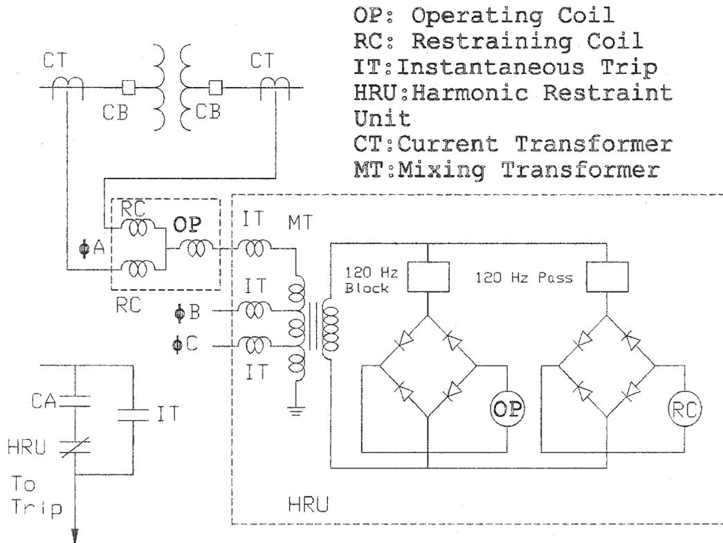
Figure 2.9: Typical Harmonic Restrained Percentage Differential relay [1]
