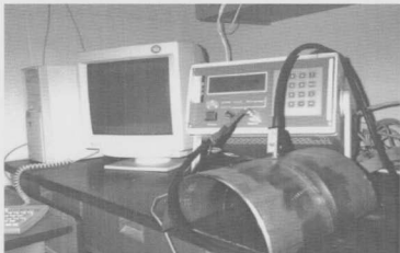
Figure 3.3. The U9b ACFM crack microgauge connected to the external computer.
