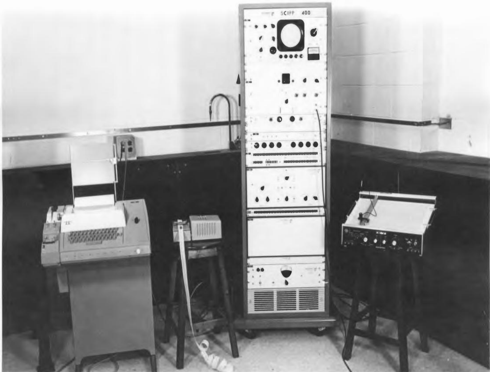
Fig. 3.5 Multi-Channel Pulse-Height Analyzer and its Accessories
