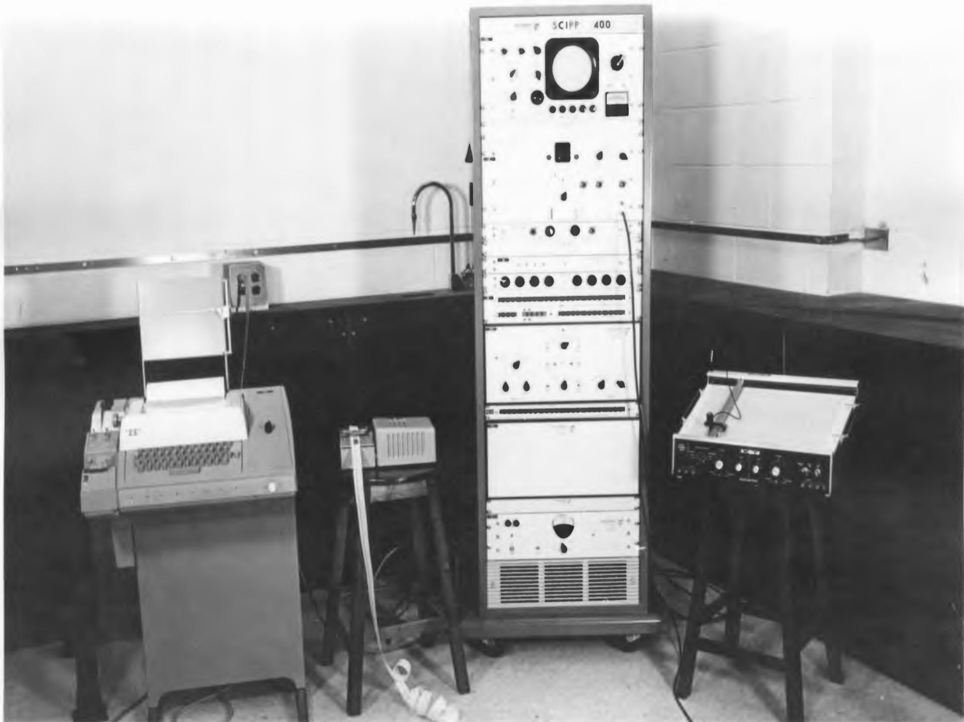
Fig. 3.5 Multi-Channel Pulse-Height Analyzer and its Accessories
