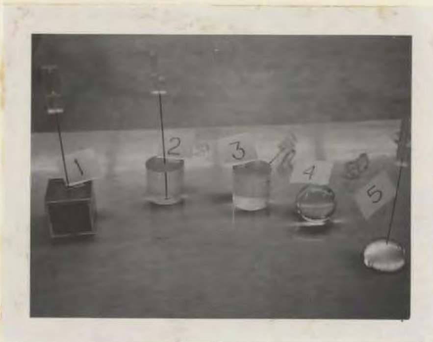
Fig. 12 PHOTOGRAPH SHOWING PLEXIGLAS MODELS USED FOR FULLY EMBEDDED BREAKOUT TESTS: (1) CUBE, (2) RIGHT CIRCULAR CYLINDER (AXIS VERTICAL), (3) RIGHT CIRCULAR CYLINDER (LONGITUDINAL AXIS IN HORIZONTAL ATTITUDE), (4) SPHERE AND (5) HEMISPHERE
