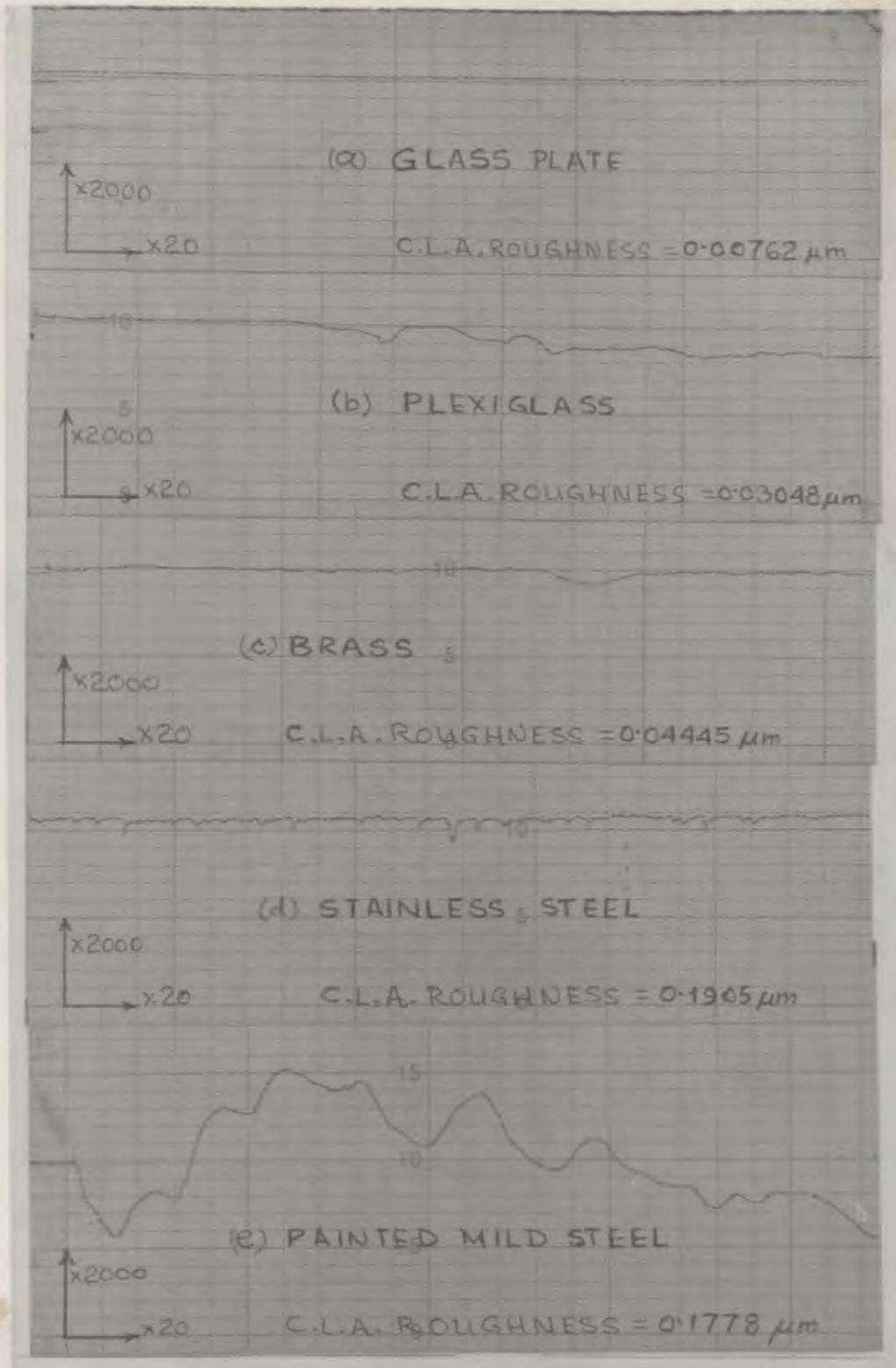
Fig. 18 SURFACE ROUGHNESS OF (a) GLASS PLATE, (b) PLEXIGLAS,
