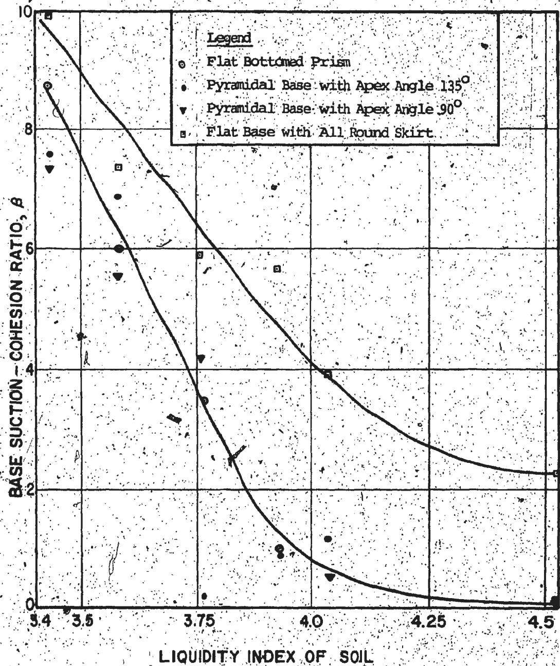
Fig. 31 VARIATION OF BASE SUCTION-COHESION RATIO WITH LIQUIDITY INDEX OF SOIL
