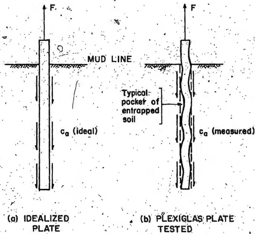
Fig. 20 CONCEPTUAL DIAGRAM SHOWING THE EFFECT OF SURFACE UNDULATIONS IN PLEXIGLAS PLATE MODEL
