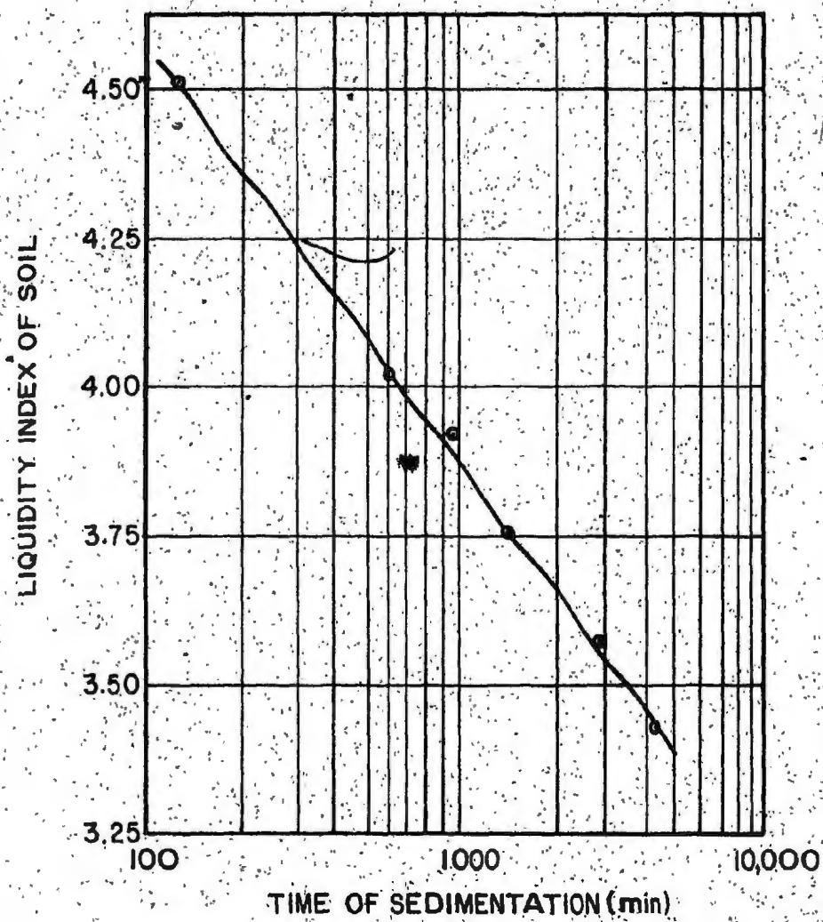
Fig. 15. LIQUIDITY INDEX VARIATION WITH TIME OF SEDIMENTATION
