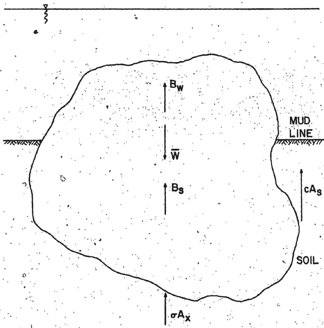
Fig. 2 CONCEPTUAL DIAGRAM SHOWING THE FORCES ON A SINKING OBJECT
