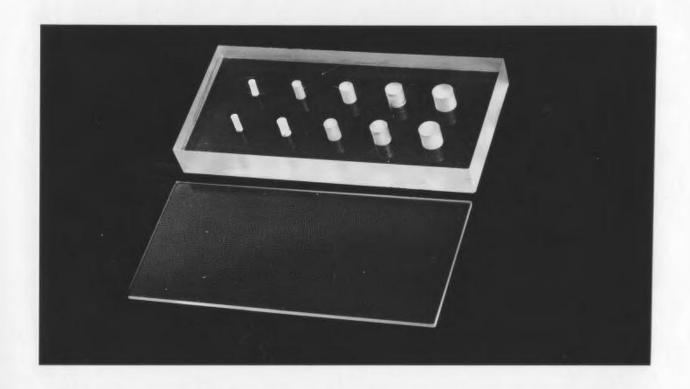
Figure 2. A drilled perspex plate of 3 mm. thickness.
