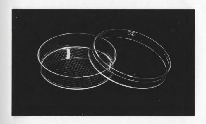
Figure 5. Integrid Petri dish with lid.
