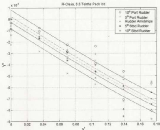
Figure E. 7 Nondimensional sway force as a function of nondimensional sway velocity for all rudder angles for the R-Class model in pack ice.
