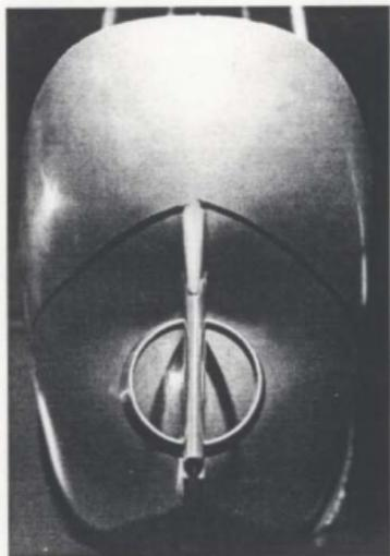
Figure A. 4 Stern view of M.V. Arctic, clearly showing the stern shape and propeller nozzle.
