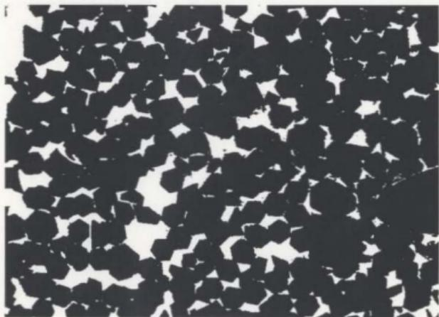
Figure C. 4 Water area threshold overlay (white portion measured).
