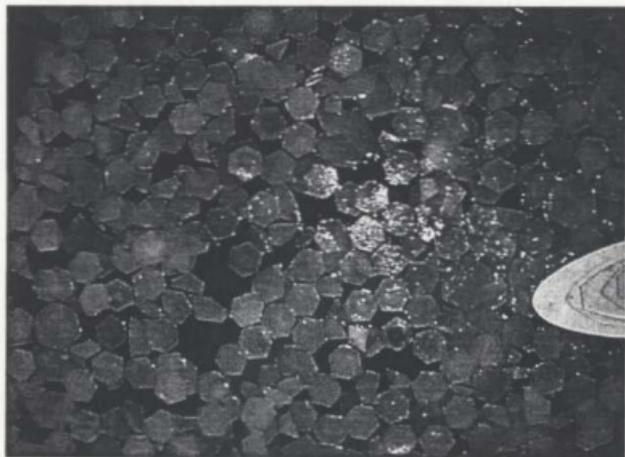
Figure 4.17 Photograph of typical wax-covered area of tank.
