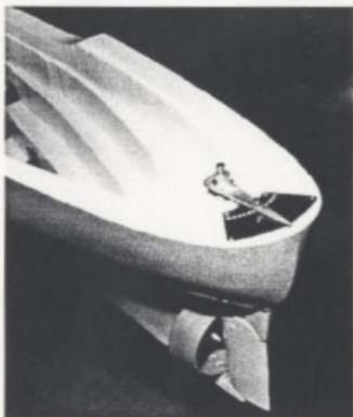
Figure 4.2 Stern view of M.V. Arctic model showing the nozzle, rudder, and rudder angle set device.
