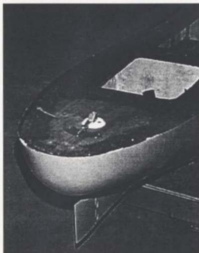
Figure 4.4 Stern view of R-Class model showing the rudder, and rudder angle set device.
