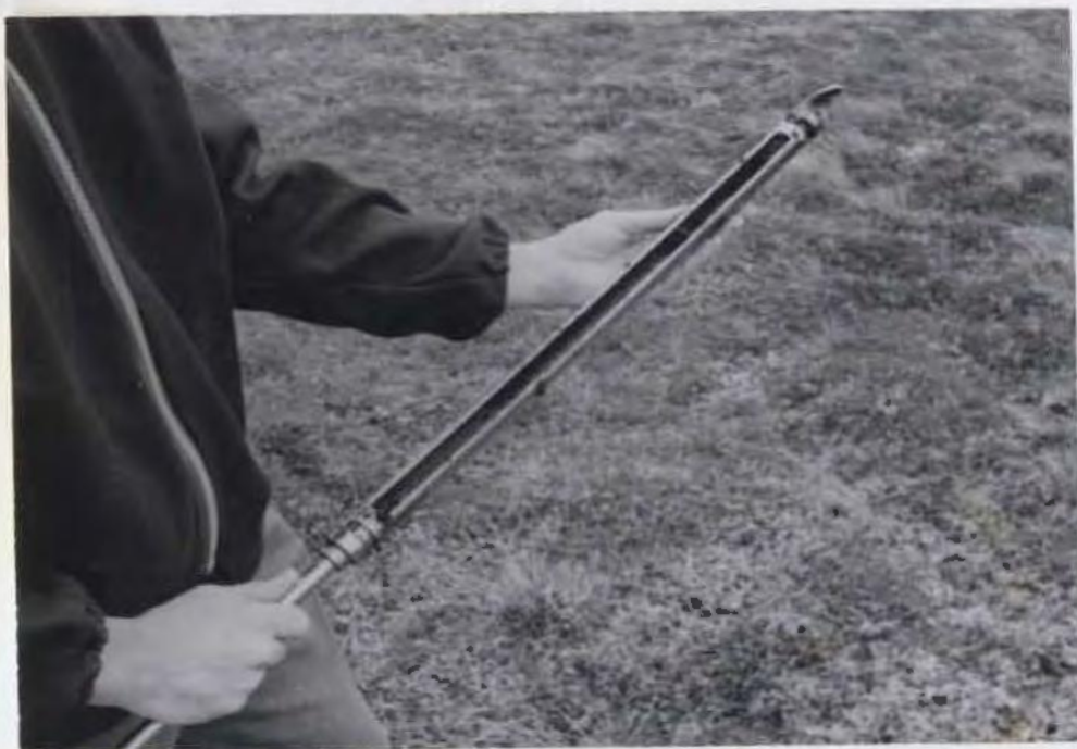
Figure 2. Swedish sampler showing cylinder, handle, and extension rod. Photo taken on Elliston Bog (108).
