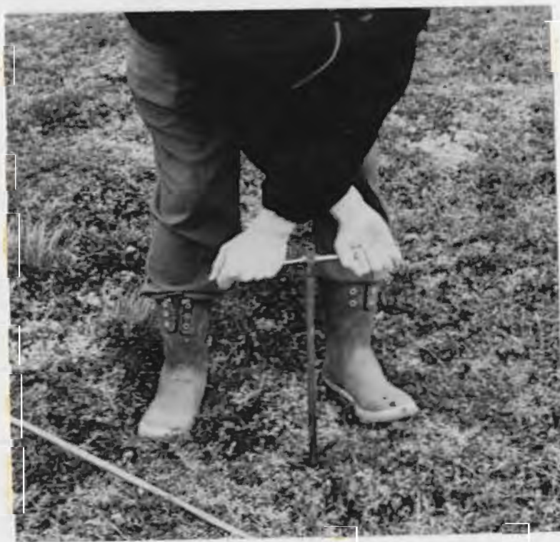
Figure 4. The sampler is first turned clockwise opening the cylinder.
