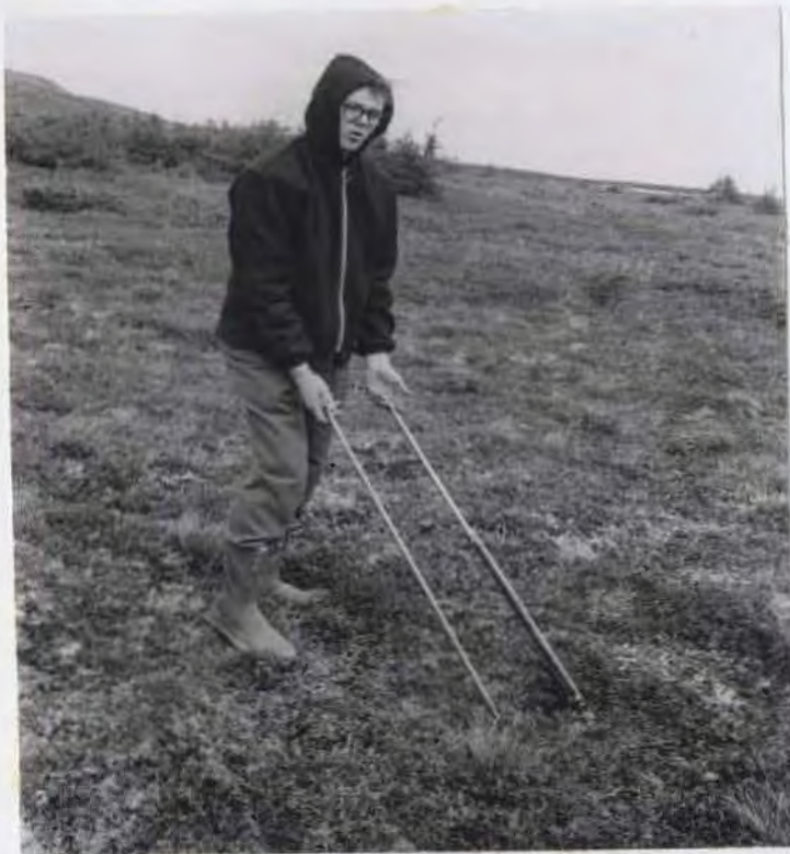
Figure 2. Swedish sampler showing cylinder, handle, and extension rod. Photo taken on Elliston Bog (108).
