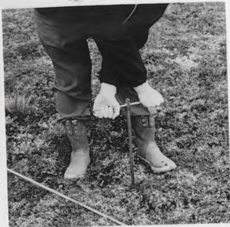
Figure 4. The sampler is first turned clockwise opening the cylinder.
