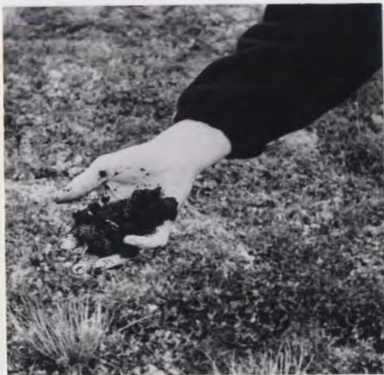
Figure 7. Peat moss is taken into the hand and squeezed to determine the degree of humification (Table 1.)
