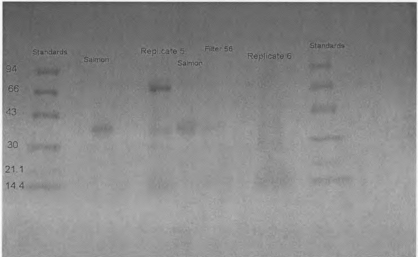
Figure C4: Coomassie blue stained electrophoresis gel used for peptide mass fingerprinting (Replicate 5 and 6 are snow crab condensate samples; filter 56 is an air filter replicate and salmon is the standard salmon tropomyosin).
