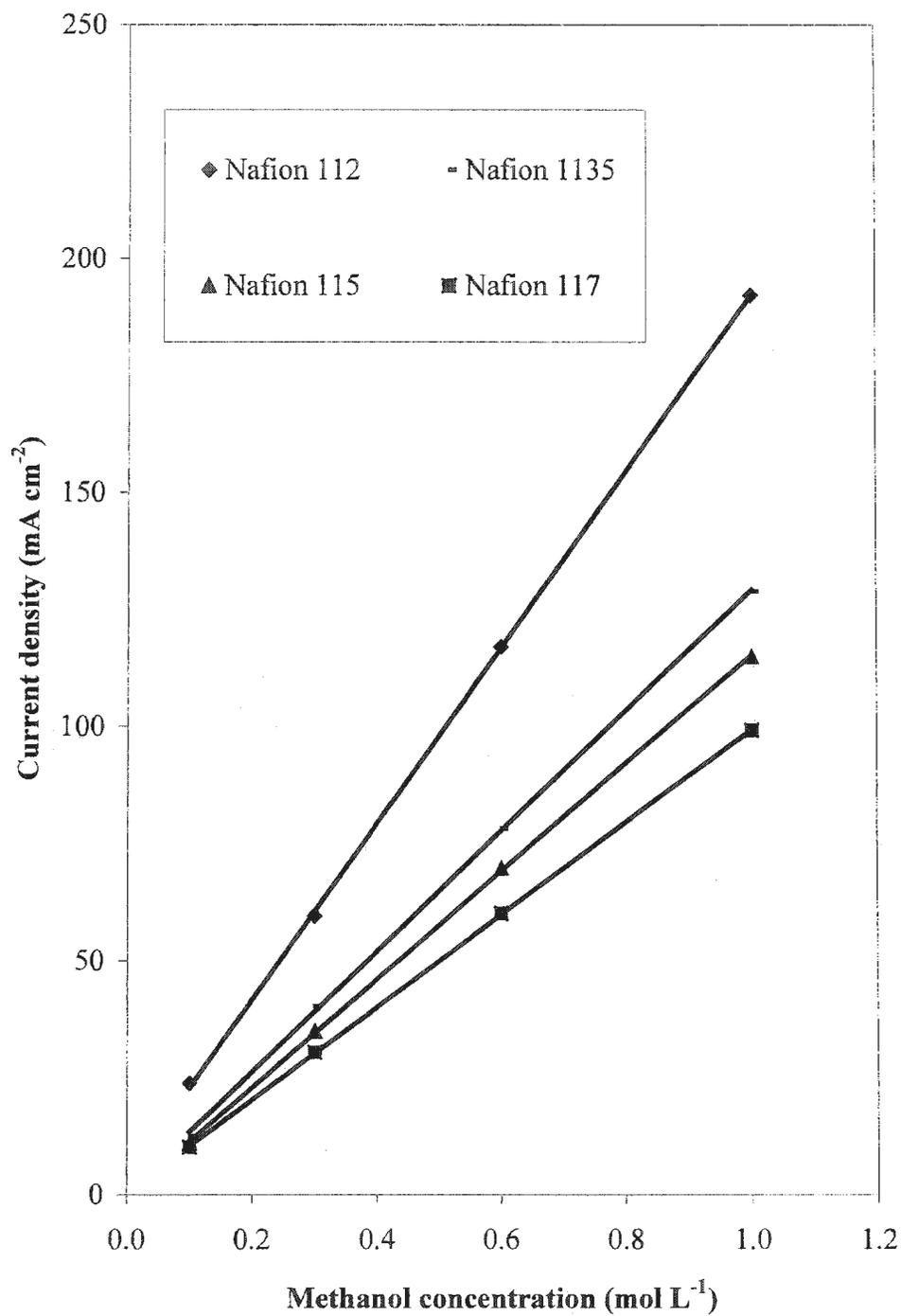
**Figure 3.6.** Concentration dependency of methanol crossover for a series of Nafion<sup>®</sup> membranes at 60 °C.
