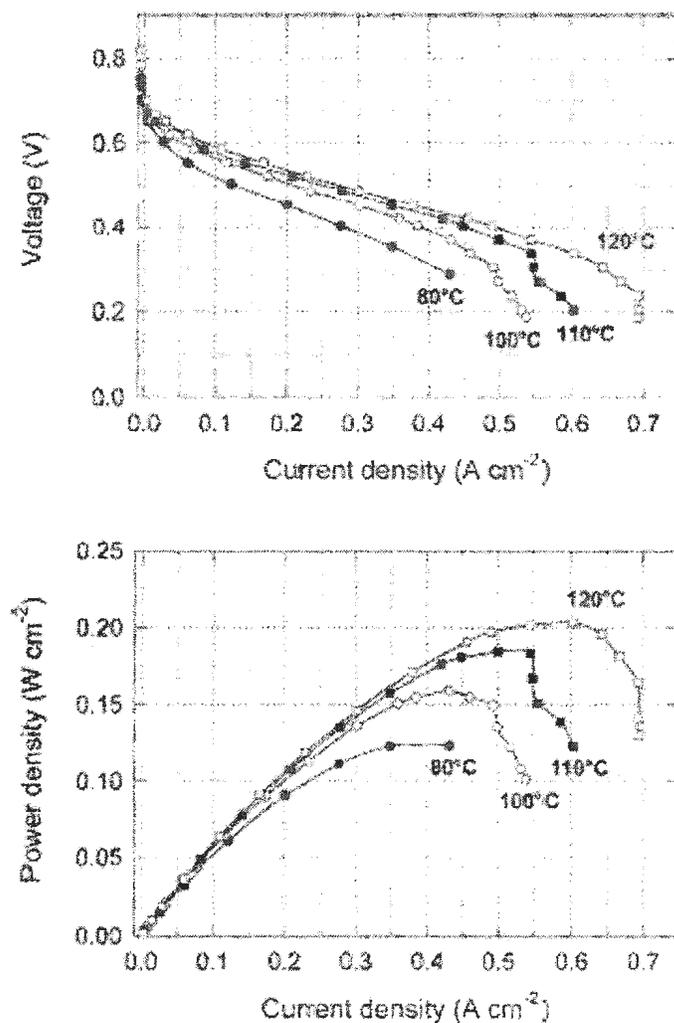
**Figure 1.4.** Voltage (top) and power density (bottom) as a function of current density for a DMFC with the total Pt loading limited to  $2.6 \text{ mg cm}^{-2}$ ; air cathode at  $2.0 \text{ atm}$  back pressure and high flow stoichiometry;  $C_{\text{MeOH}} = 0.5 \text{ M}$ ,  $f_{\text{MeOH}} = 2.0 \text{ mL min}^{-1}$ .
