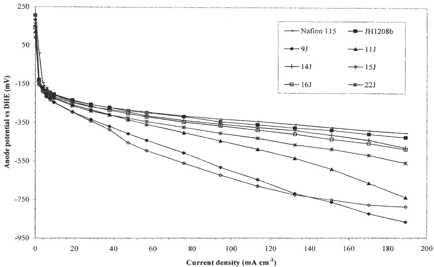
**Figure 5.2.** DMFC anode performances for unmodified and modified Nafion 115 membranes treated with  $\text{Fe}^{3+}$  at 60 °C and at ambient pressure.  $f_{\text{Nitrogen}} = 25.6 \text{ mL min}^{-1}$ ,  $C_{\text{MeOH}} = 1 \text{ mol L}^{-1}$ .
