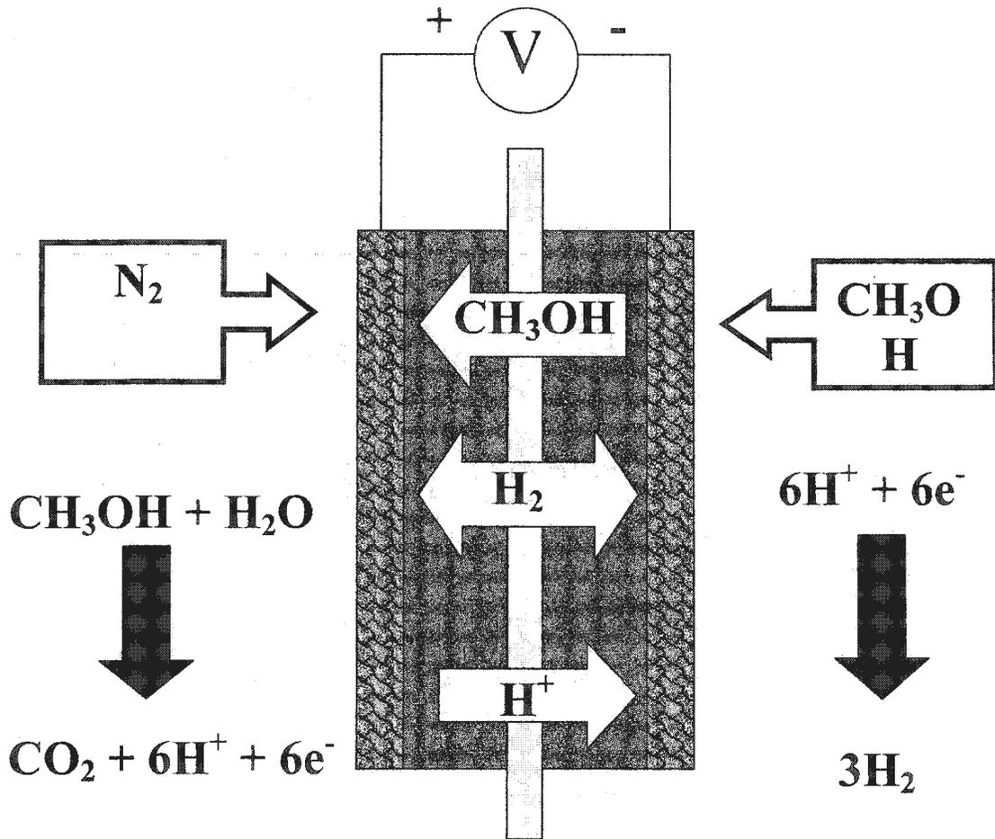
**Figure 3.1.** A schematic diagram showing the methanol permeation process and the electrode reactions involved in the electrochemical measurement of crossover.
