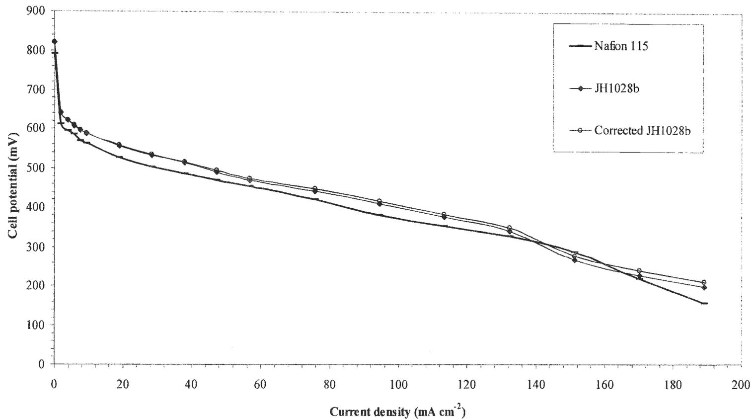
**Figure 4.4.** DMFC performances of Nafion 115 and JH1028b membranes running with air at 60 °C and at ambient pressure,  $f_{air} = 73.1 \text{ mL min}^{-1}$ ,  $C_{MeOH} = 1 \text{ mol L}^{-1}$ . The corrected JH1028b data has been adjusted to the same cell resistance as unmodified Nafion 115 ( $0.16 \Omega \text{ cm}^2$ ).
