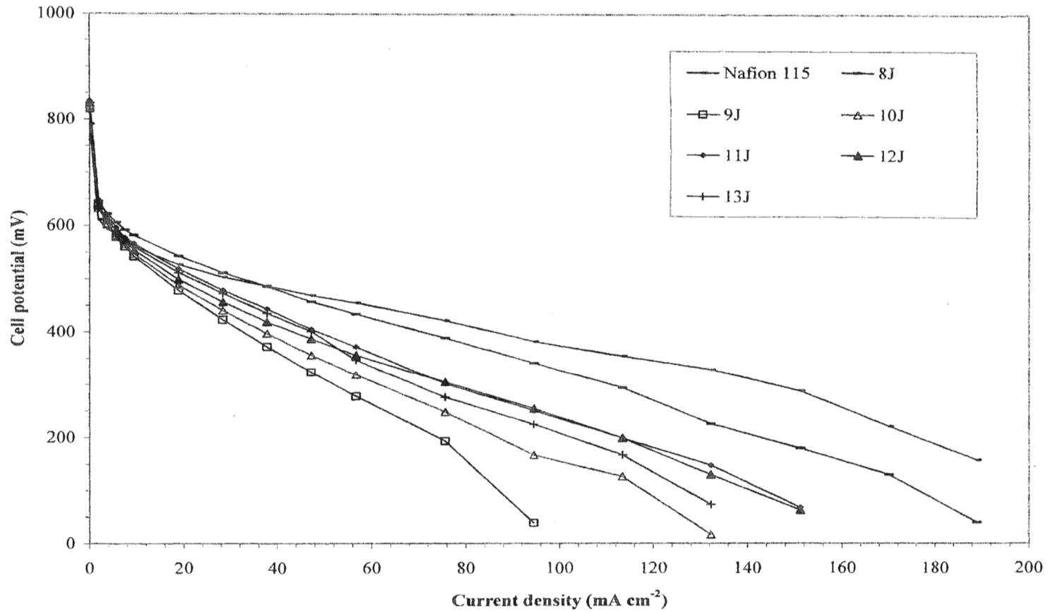
**Figure 4.6.** DMFC performances after running the cell for 3 days, for unmodified and modified Nafion 115 running with air at 60 °C and at ambient pressure.  $f_{air} = 73.1 \text{ mL min}^{-1}$ ,  $C_{MeOH} = 1 \text{ mol L}^{-1}$ .
