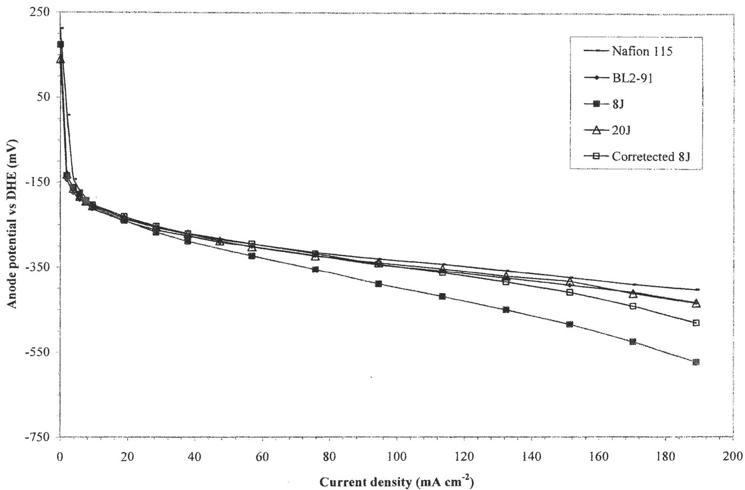
**Figure 5.1.** Anode performances for unmodified and modified Nafion 115 prepared by H<sub>2</sub>O<sub>2</sub> oxidation, running at 60 °C and at ambient pressure.  $f_{Nitrogen} = 25.6 \text{ mL min}^{-1}$ ,  $C_{MeOH} = 1 \text{ mol L}^{-1}$ .
