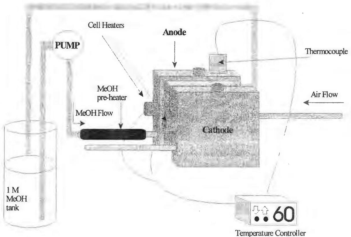
**Figure 1.1.** A schematic diagram of a direct methanol fuel cell system.
