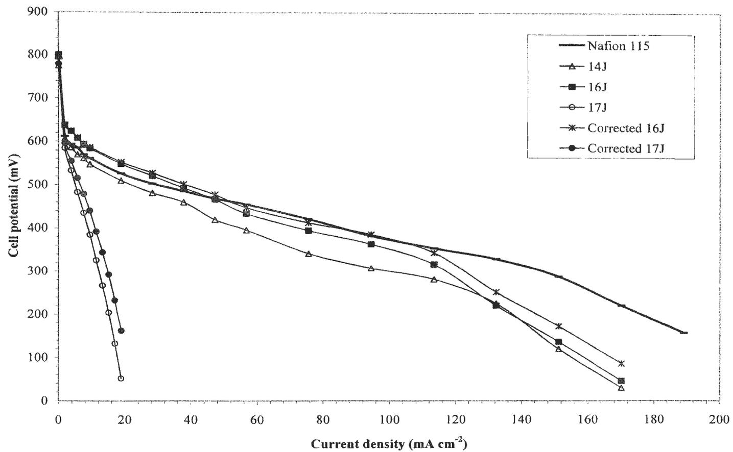
**Figure 4.9.** DMFC polarization curves for Nafion 115 and composite membranes running with air at 60 °C and at ambient pressure.  $f_{air} = 73.1 \text{ mL min}^{-1}$ ,  $C_{MeOH} = 1 \text{ mol L}^{-1}$ .
