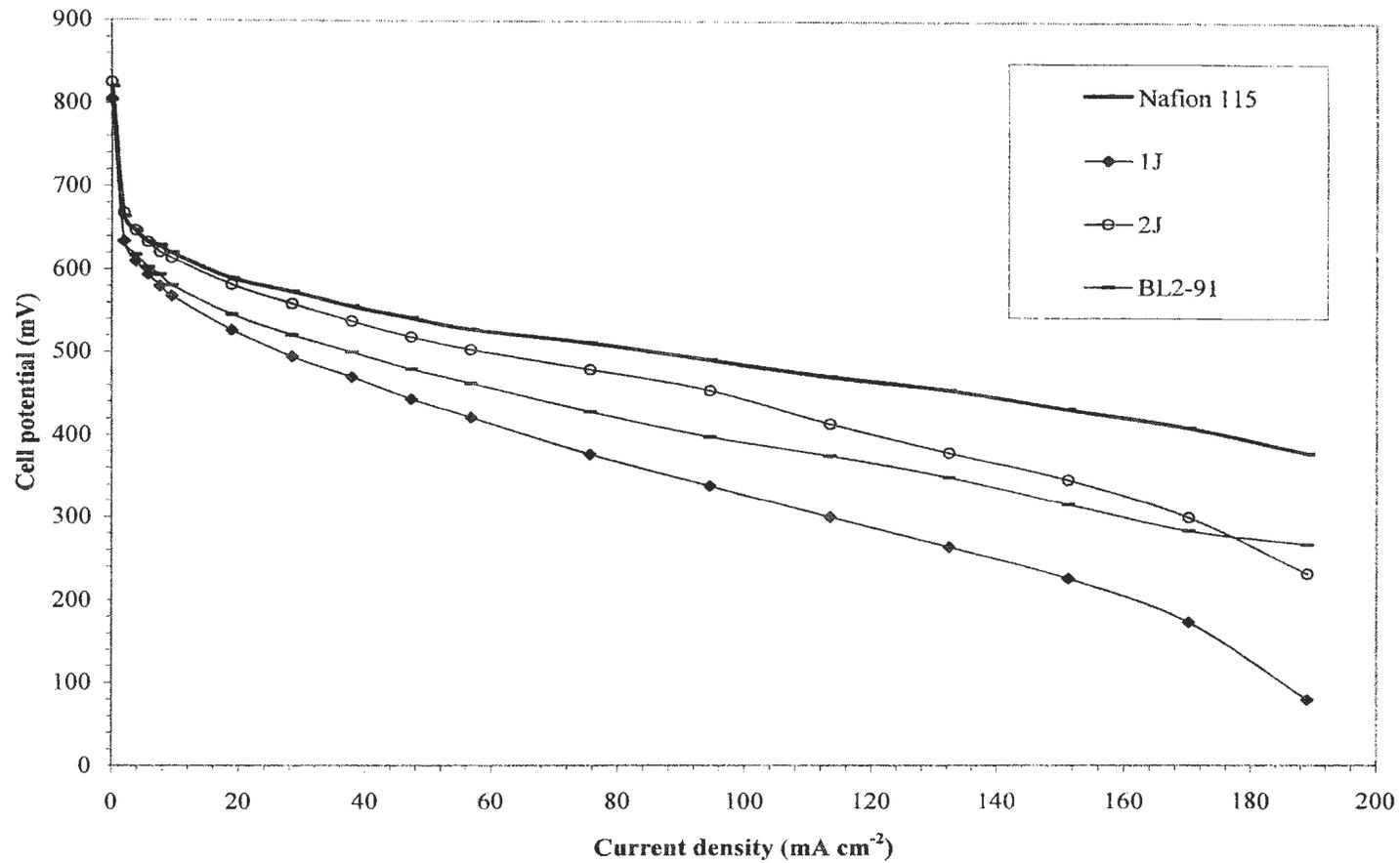
**Figure 4.2.** DMFC performances for unmodified and modified Nafion 115 membranes running with oxygen at 60 °C and at ambient pressure.  $f_{\text{oxygen}} = 12.3 \text{ mL min}^{-1}$ ,  $C_{\text{MeOH}} = 1 \text{ mol L}^{-1}$ .
