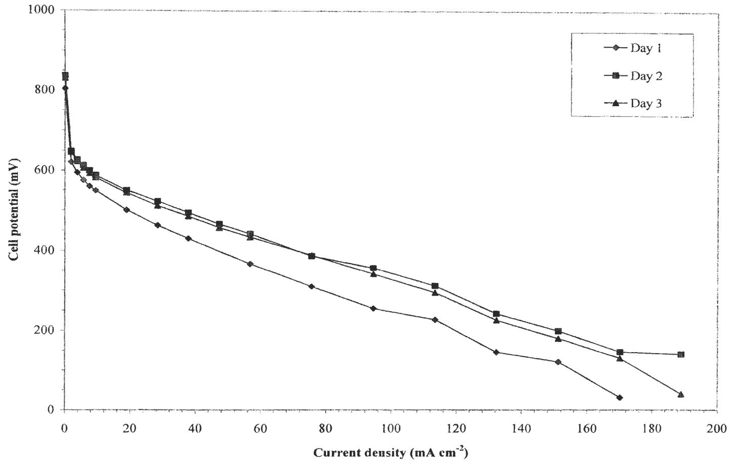
**Figure 4.5.** DMFC performance of 8J composite membrane running for 3 days with air at 60 °C and at ambient pressure.  $f_{air} = 73.1 \text{ mL min}^{-1}$ ,  $C_{MeOH} = 1 \text{ mol L}^{-1}$ .
