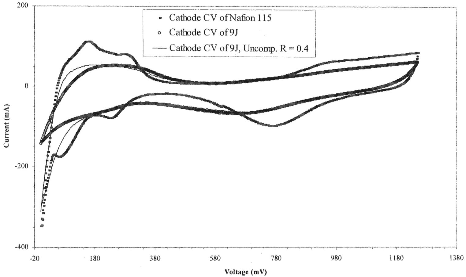
**Figure 5.4.** Cathode CVs for unmodified Nafion 115 and modified 9J membranes treated with  $\text{Fe}^{3+}$  at room temperature and at ambient pressure.  $f_{\text{Hydrogen}} = 18.6 \text{ mL min}^{-1}$ ,  $f_{\text{Nitrogen}} = 25.6 \text{ mL min}^{-1}$ , step height = 2 mV, scan time = 0.1 s.
