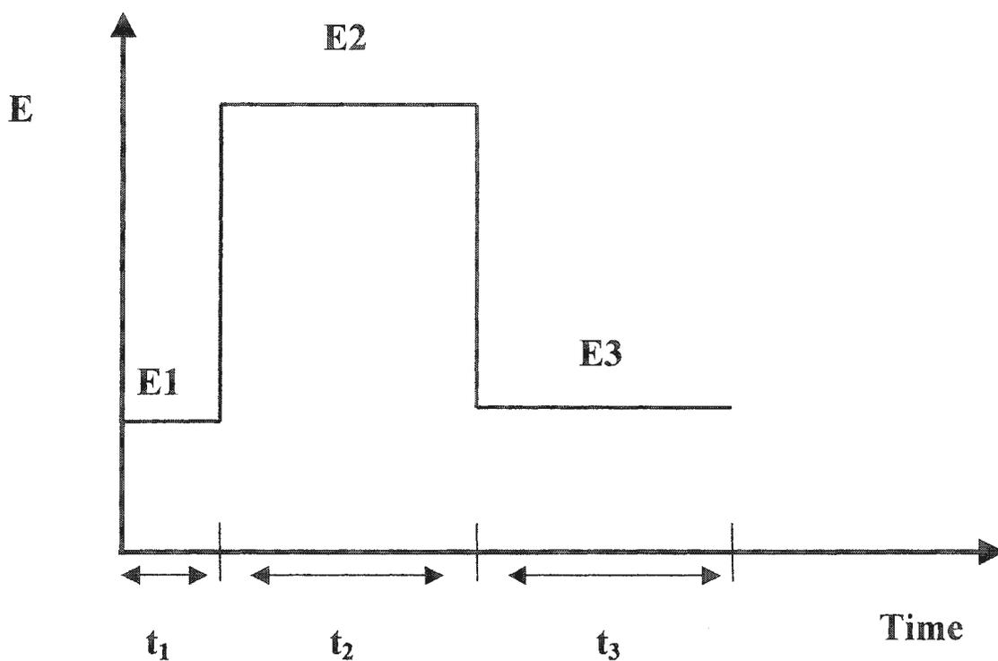
**Figure 3.3.** Chronoamperometric potential time diagram.
