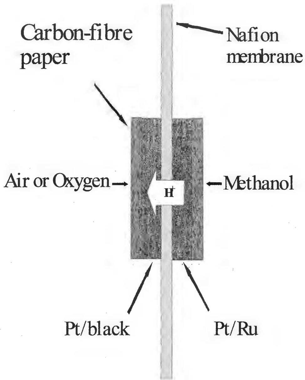
**Figure 1.3.** A schematic diagram of a membrane and electrode assembly (MEA).
