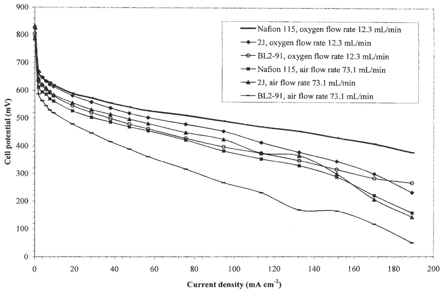
**Figure 4.1.** DMFC performances for unmodified and modified Nafion 115 running with oxygen or air at 60 °C and at ambient pressure.  $C_{MeOH} = 1 \text{ mol L}^{-1}$ .
