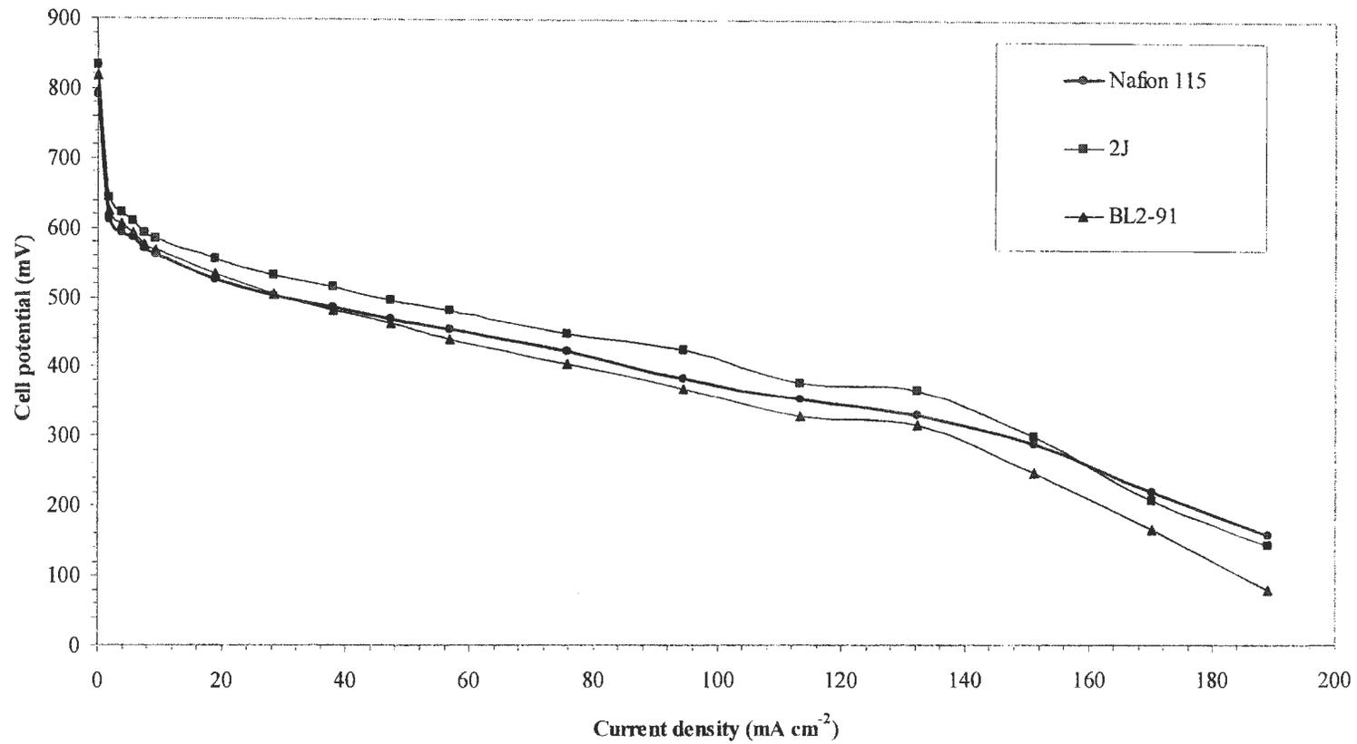
**Figure 4.3.** DMFC performances for unmodified and modified Nafion 115 membranes running with air at 60 °C and at ambient pressure.  $f_{air} = 73.1 \text{ mL min}^{-1}$ ,  $C_{MeOH} = 1 \text{ mol L}^{-1}$ .
