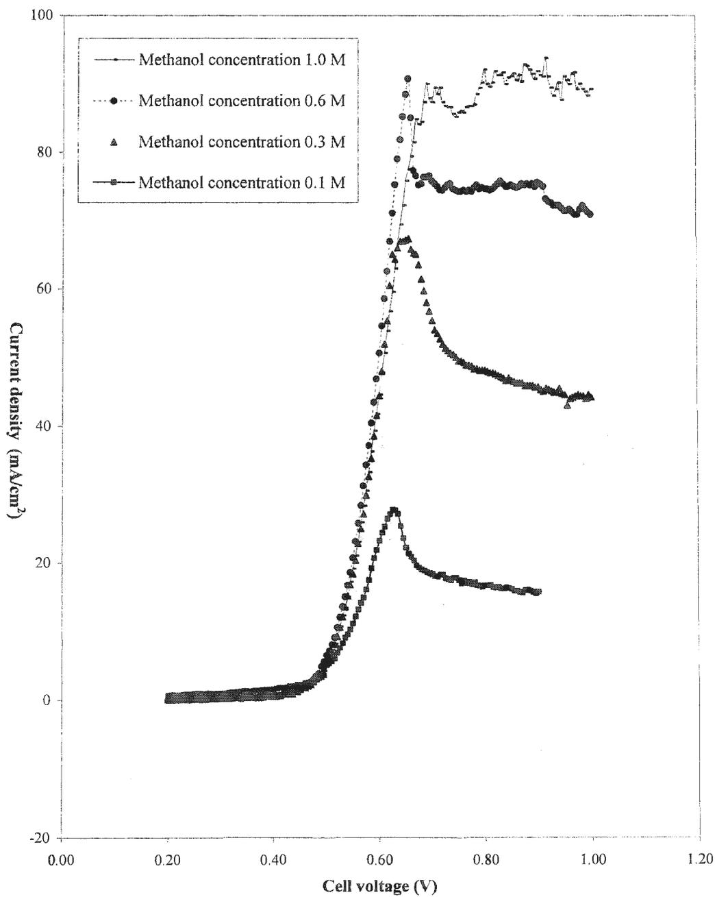
**Figure 3.2.** Voltammetric curves at 50 °C for the oxidation of methanol crossing through Nafion<sup>®</sup> 112 using 0.1, 0.3, 0.6, and 1.0 M methanol solutions, step height = 5 mV, step time = 2.5 s.
