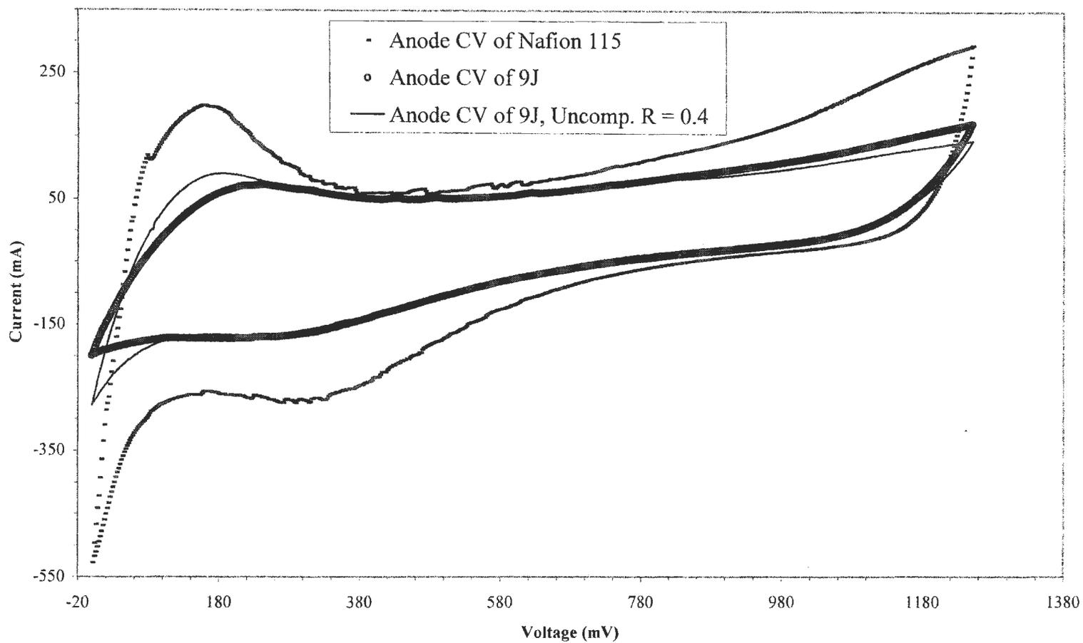
**Figure 5.5.** Anode CVs for unmodified Nafion 115 and modified 9J membranes treated with  $\text{Fe}^{3+}$  at room temperature and at ambient pressure.  $f_{\text{Hydrogen}} = 18.6 \text{ mL min}^{-1}$ ,  $f_{\text{Nitrogen}} = 25.6 \text{ mL min}^{-1}$ , step height = 2 mV, scan time = 0.1 s.
