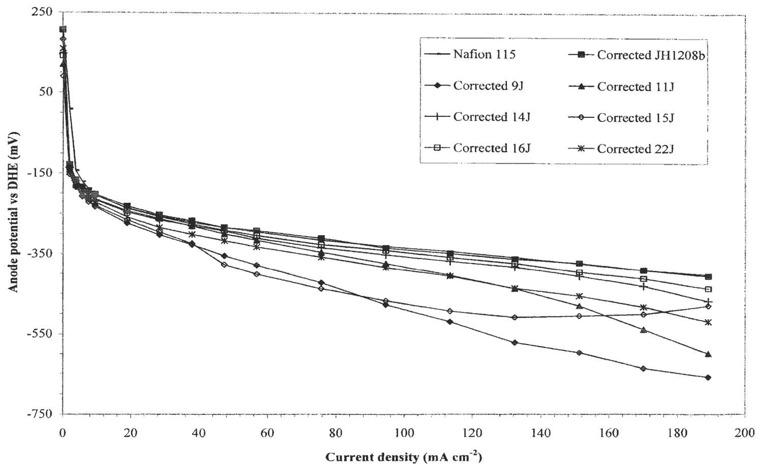
**Figure 5.3.** Resistance corrected DMFC anode performances for unmodified and modified Nafion 115 membranes treated with  $\text{Fe}^{3+}$  at 60 °C and at ambient pressure.  $f_{\text{Nitrogen}} = 25.6 \text{ mL min}^{-1}$ ,  $C_{\text{MeOH}} = 1 \text{ mol L}^{-1}$ .
