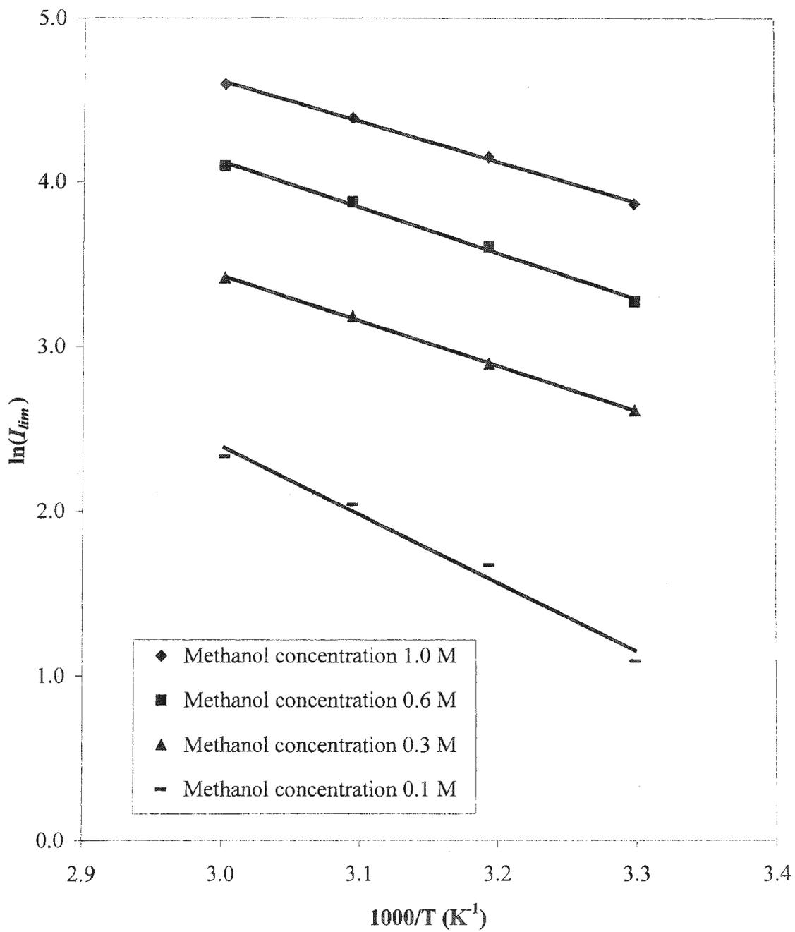
Figure 3.4. Temperature dependence of methanol crossover for Nafion®
