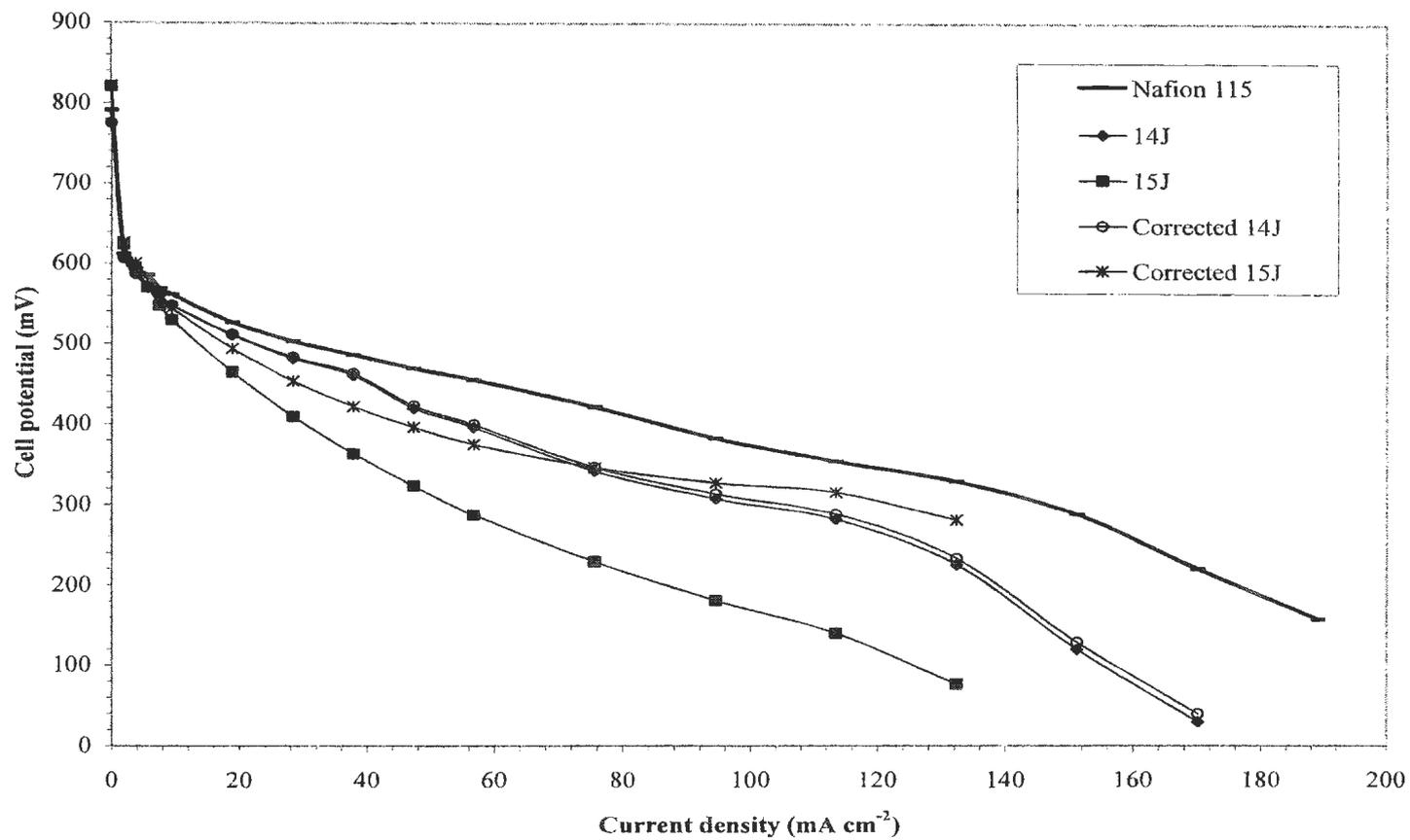
**Figure 4.8.** DMFC polarization curves for Nafion 115, 14J and 15J running with air at 60 °C and at ambient pressure.  $f_{air} = 73.1 \text{ mL min}^{-1}$ ,  $C_{MeOH} = 1 \text{ mol L}^{-1}$ .
