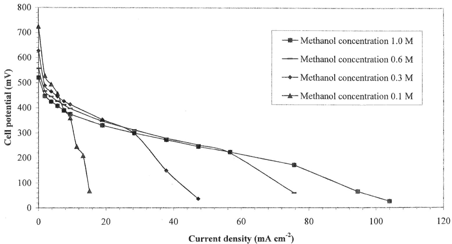
**Figure 3.7.** Polarization curves of a DMFC operated at 60 °C using a Nafion<sup>®</sup> 115 membrane with different methanol concentrations.
