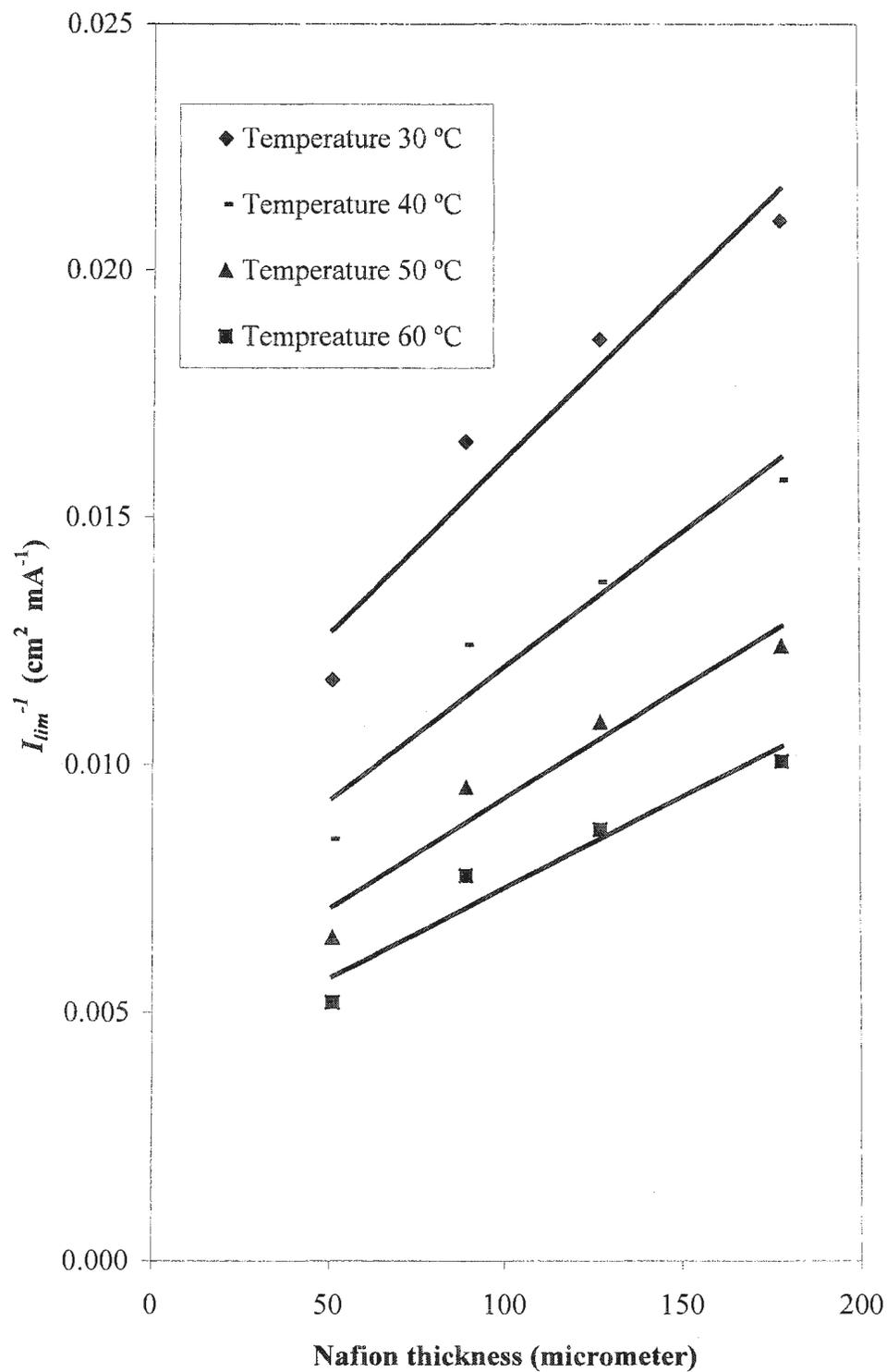
**Figure 3.5.** Thickness dependence of methanol crossover for a series of membranes using  $1 \text{ mol L}^{-1}$  methanol solution at different temperatures.
