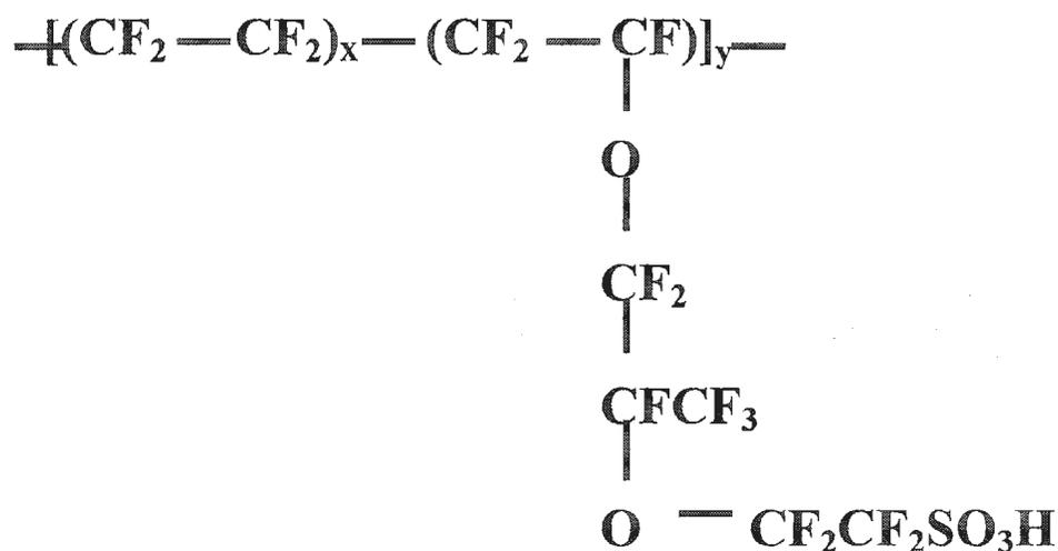
**Figure 1.5.** The general structure of Nafion<sup>®</sup>.
