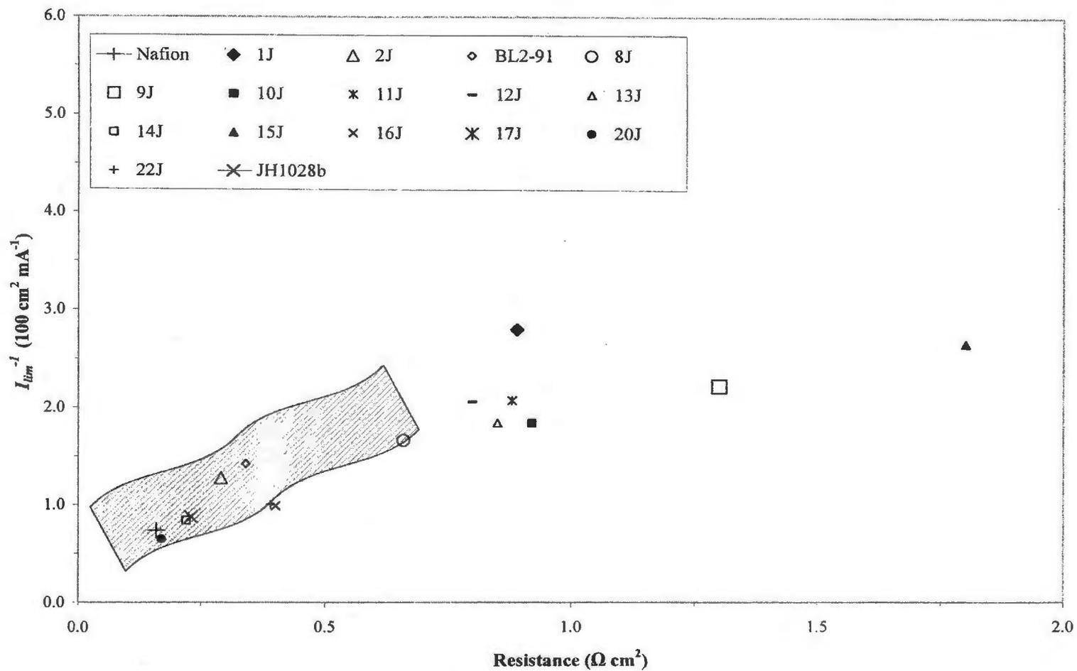
Figure 4.12. Resistance vs.  $I_{lim}^{-1}$  diagram for unmodified and modified Nafion 115 membranes.
