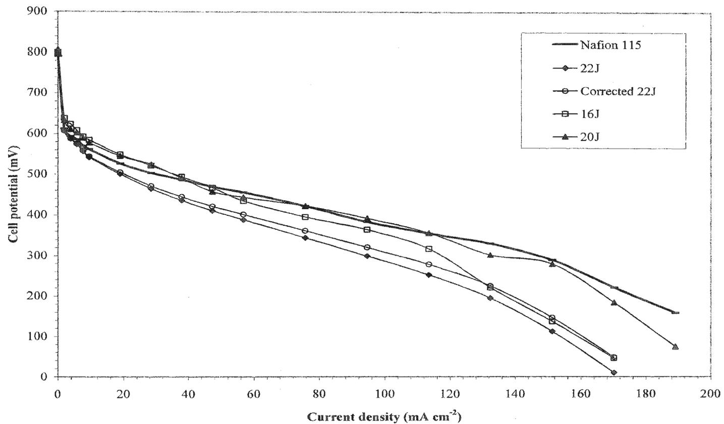
Figure 4.11. DMFC performances for unmodified and modified Nafion 115 running with air at 60 °C and at ambient pressure.  $f_{air} = 73.1 \text{ mL min}^{-1}$ ,  $C_{MeOH} = 1 \text{ mol L}^{-1}$ .
