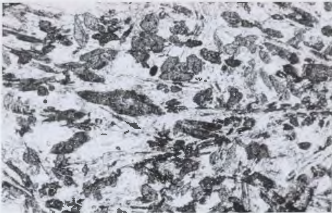
FIGURE 3.2: RJ75-162: Kaersutite microlites in massive flow intergrown with plagioclase laths. Large euhedral crystal at centre is about 0.5 mm across.
