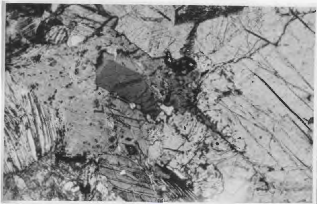
FIGURE 3.6: RJ75-286. Gabbro, showing fresh pyroxene (right), amphibole rimming pyroxene (medium to dark grey, centre), and chloritized biotite (left). Width of field is about 3 mm.
