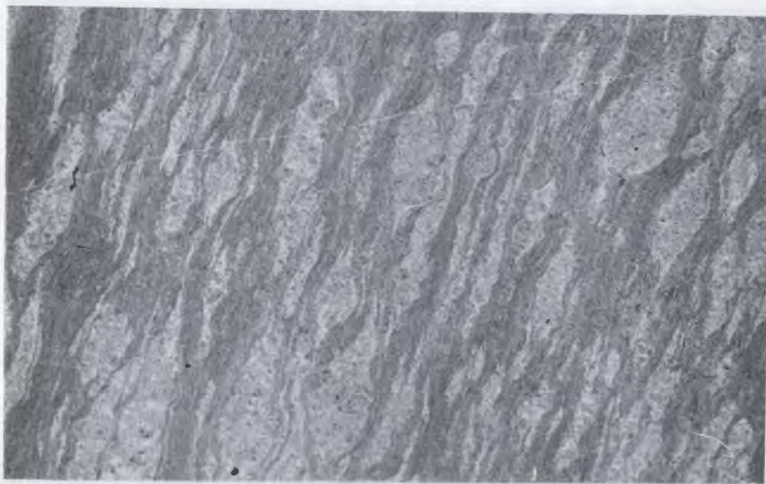
FIGURE 3.25: RJ75-117. Spotted greenschist showing elongated aggregates of epidote, calcite, and albite after plagioclase porphyroclasts, in a matrix of actinolitic hornblende. Width of field is 3.8 cm.
