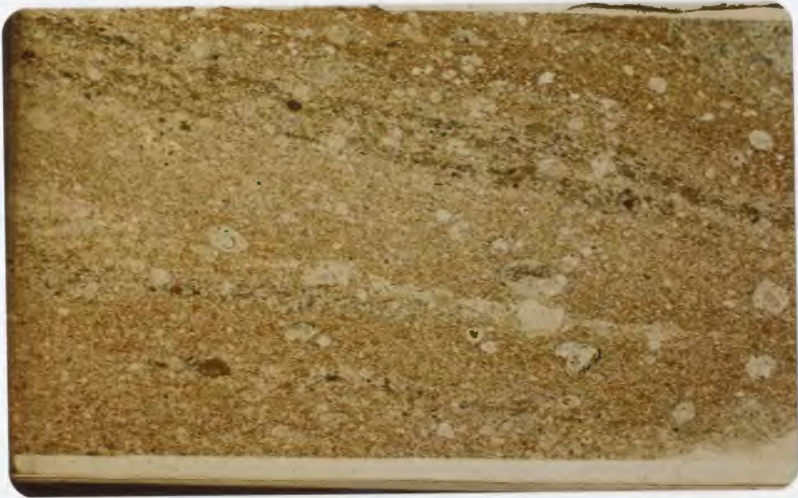
3.36a: RJ75-082. Biotite amphibolite showing disrupted hornblende-rich layers and garnet, feldspar, and hornblende porphyroclasts in a fine-grained biotite- and quartz-rich matrix. Width of field is 3.8 cm.
