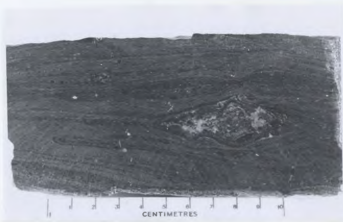
FIGURE 2,23: RJ75-138, biotite amphibolite containing epidote amphibolite inclusions, Three Mountain Summit.
