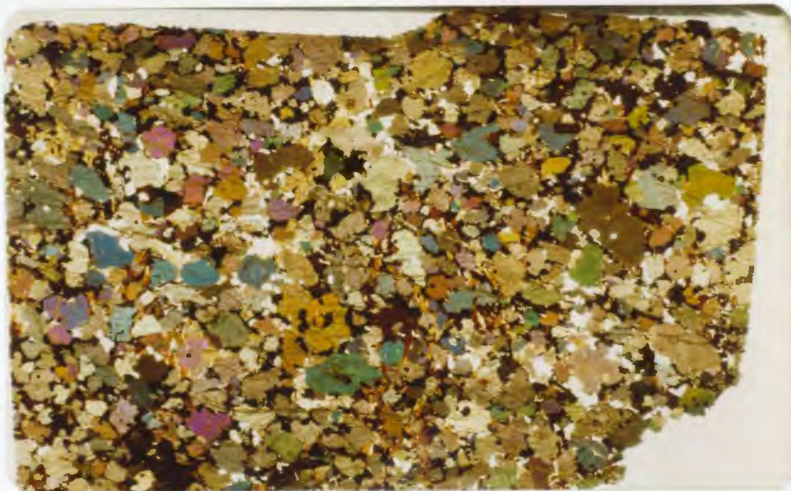
3.54a: RJ76-491: Undeformed jacupirangite with titanaugite (bright colours) and interstitial biotite and kaersutite (brown), ilmenite (black), and apatite (white). (Partly crossed Nicols). Width of field is 3.2 cm.
