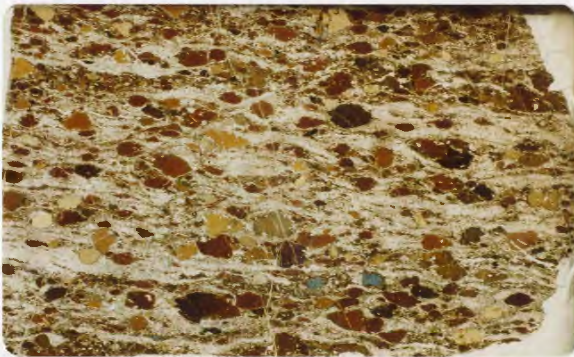
3.54b: RJ76-488. Hornblende gneiss, showing kaersutite augen (brown), relict titanaugite (blue), and interstitial fine-grained albite (grey and white). (Partly crossed Nicols). Width of field is 3.2 cm.
