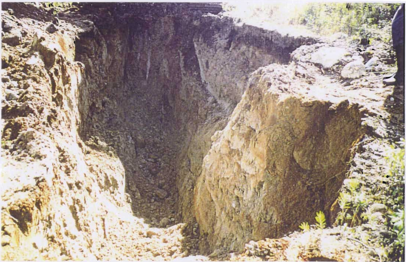
Photograph #1 - Test pit #1 showing non layering of glacial till overburden - Sept. 21, 1993
