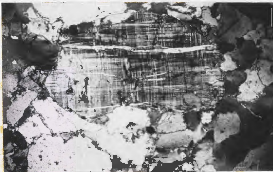
Pl. XXXIII. Photomicrograph of sand grain of unaltered microcline displaying cross-hatched twinning. Fractures are associated with deformation of the sediment. X 38.
