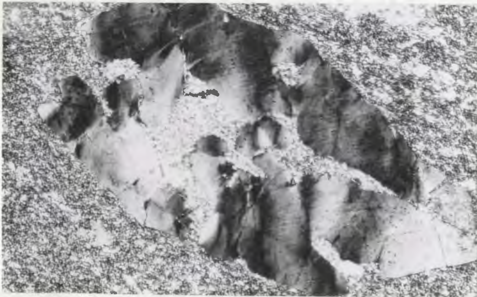
Glide lamellae developed in deformed quartz crystal. MJBb. X-nicols, X65.
