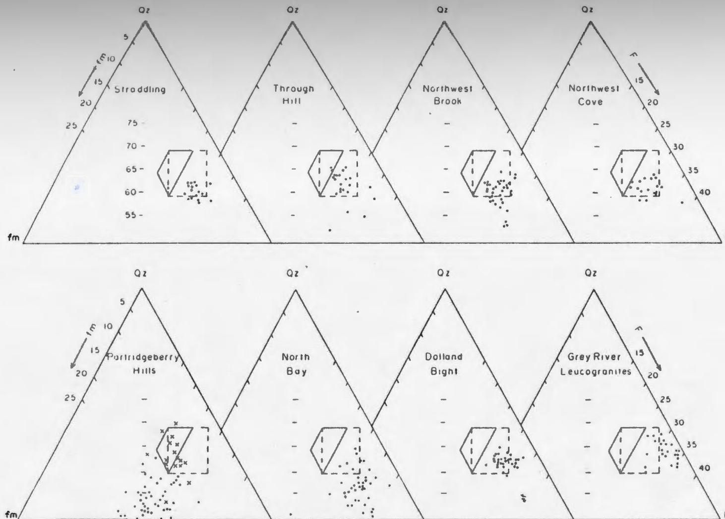
Fig. 7.1. Kohler-Raatz indices for selected South-Central Newfoundland granitoids. Dashed square indicates the field of favourable tin granites of the Bohemian Massif after Sattran and Klominsky (1970). Solid trapezoid outlines the favourable field for tin granites of Eastern Australia after Hesp and Rigby (1977). Qz=silicon in quartz; F=sodium and potassium in feldspar. fm=ferric cations in ferromagnesian minerals.
