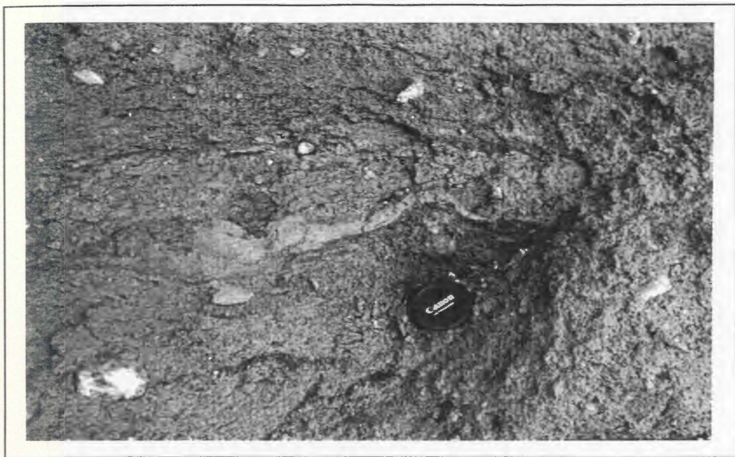
Plate 5.1 - Sinusoidal sand lens within Section A11a draping the underlying clast. The lens is 17 cm wide and 1 cm thick.
