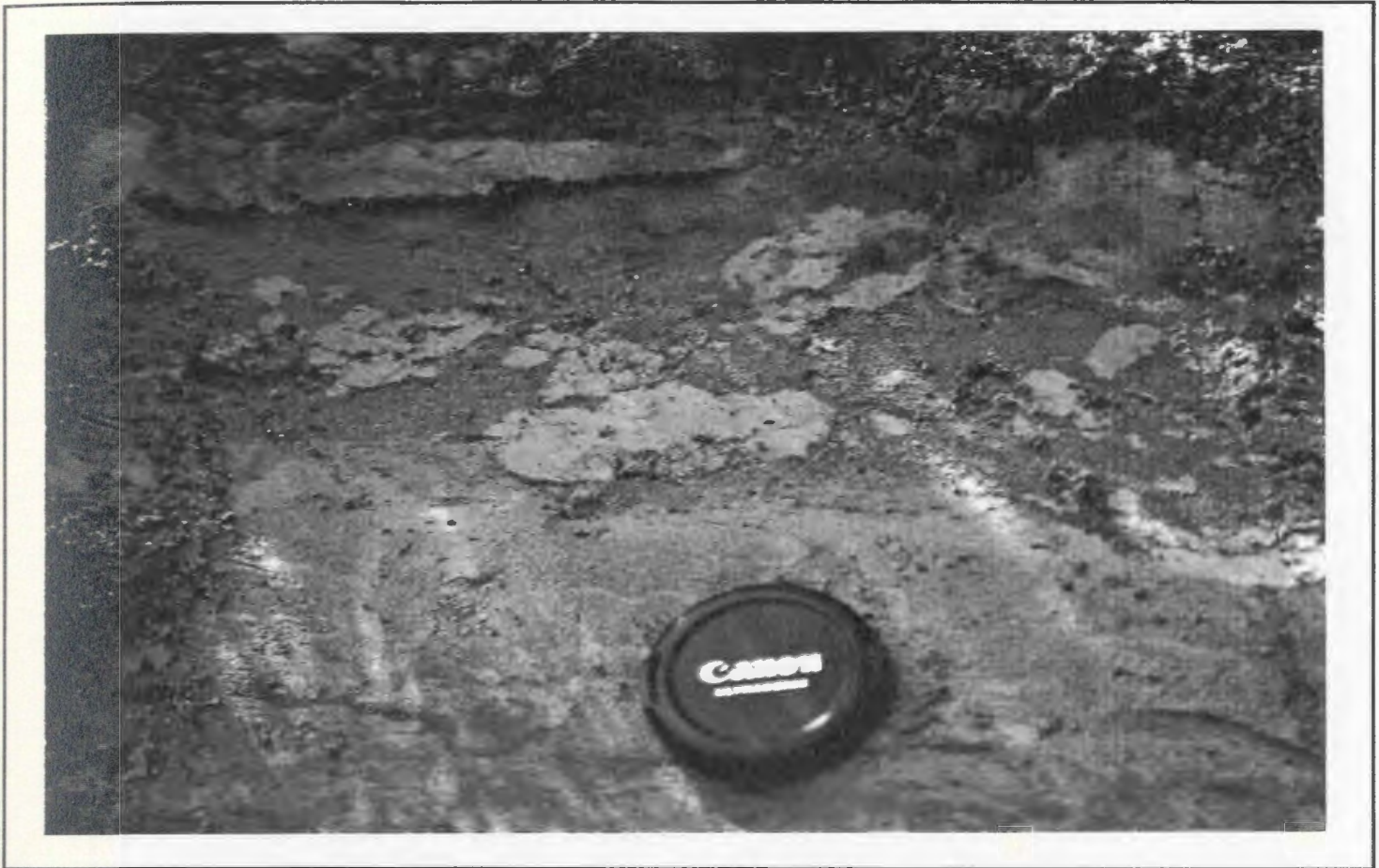
Plate 7.2 - Lenses of medium sand at the top of the clay, silt and sand unit (A18). The lenses are 1.1-0.7 cm wide and 0.7-1.5 cm thick. All the lenses have an irregular shape and sharp contacts with the surrounding coarse sand.
