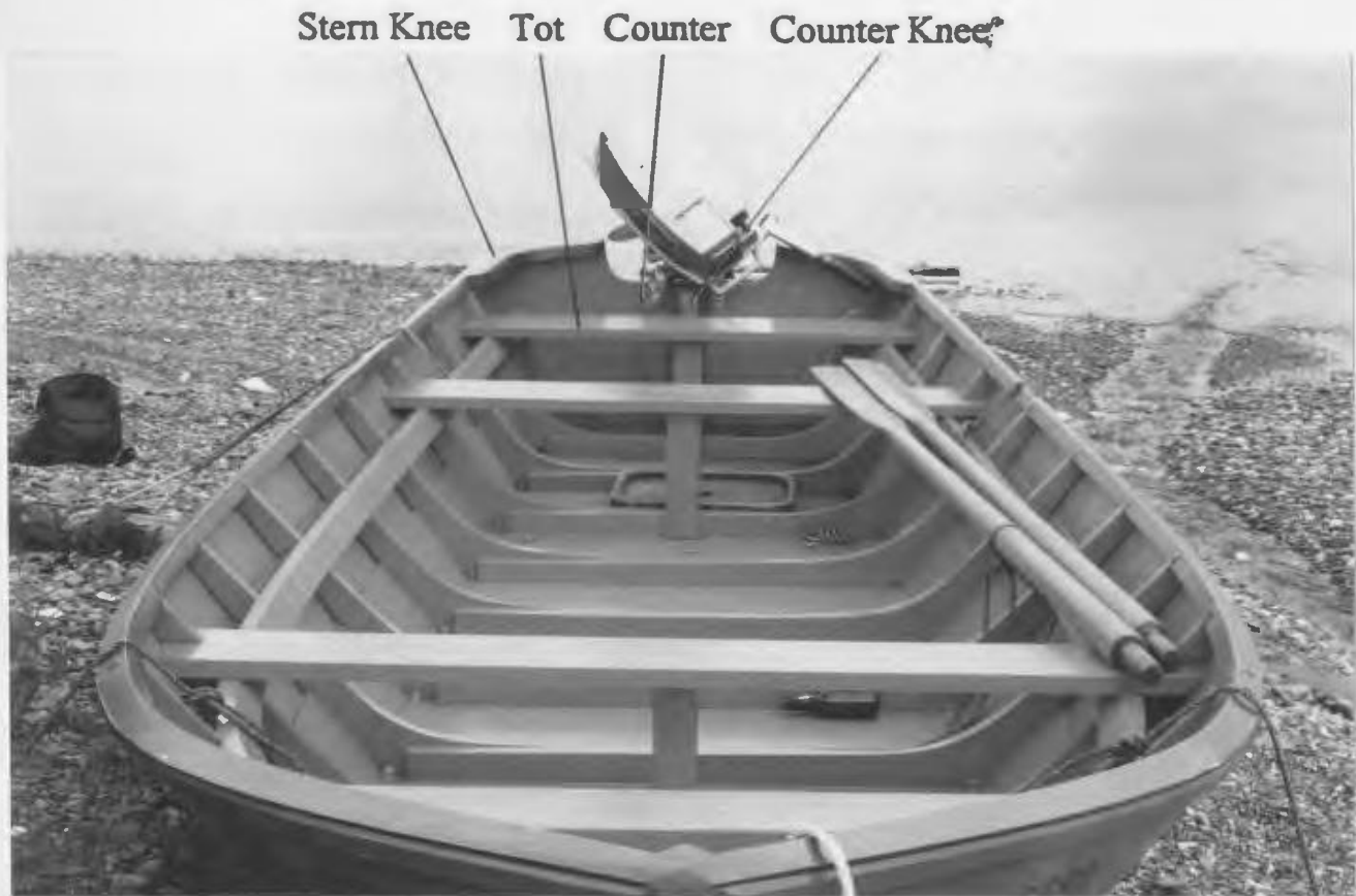
Figure 1.3. Dory built by Freeman Sheppard of York Harbour with parts identified.
