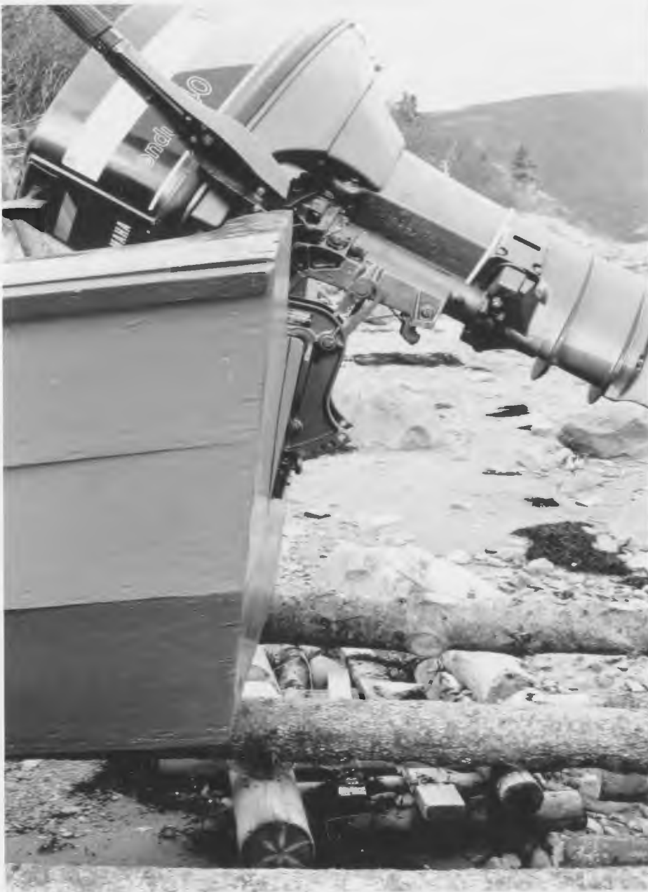
Figure 6.4. Dory built by Freeman Sheppard with counter wedges in place. The counter wedges were used to change the pitch on the counter of the dory without alteration of the existing counter. At the time of this photo in 1994 Freeman Sheppard was experimenting with different wedge sizes. The extra pitch provided by these wedges was to be built into the next dory.
