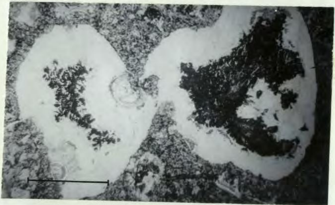
Photomicrograph 8: Chlorite rim and epidote core of vesicle in Calmer Formation basalt. (Plane polarized light; bar scale = .75 mm).
