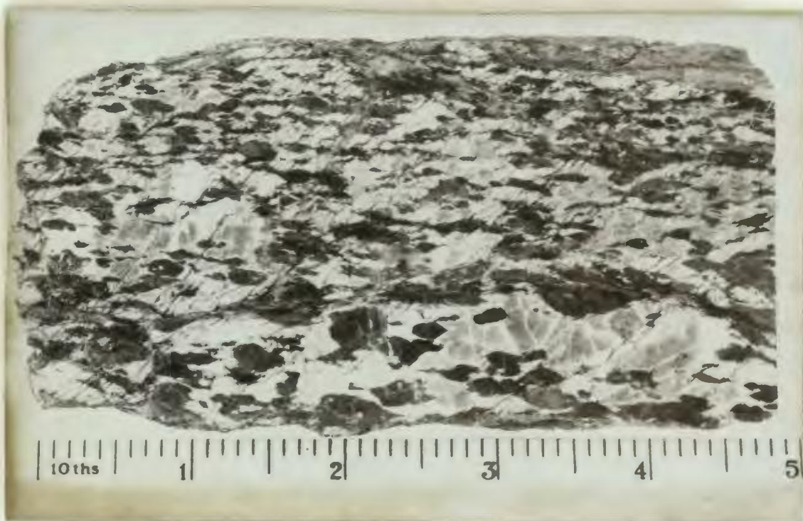
a: "Flaser gabbro" - Strong fabric in gabbro; elongation and augens of crystals - O'Dwyer Mountain slice. Note fractures in rock.
