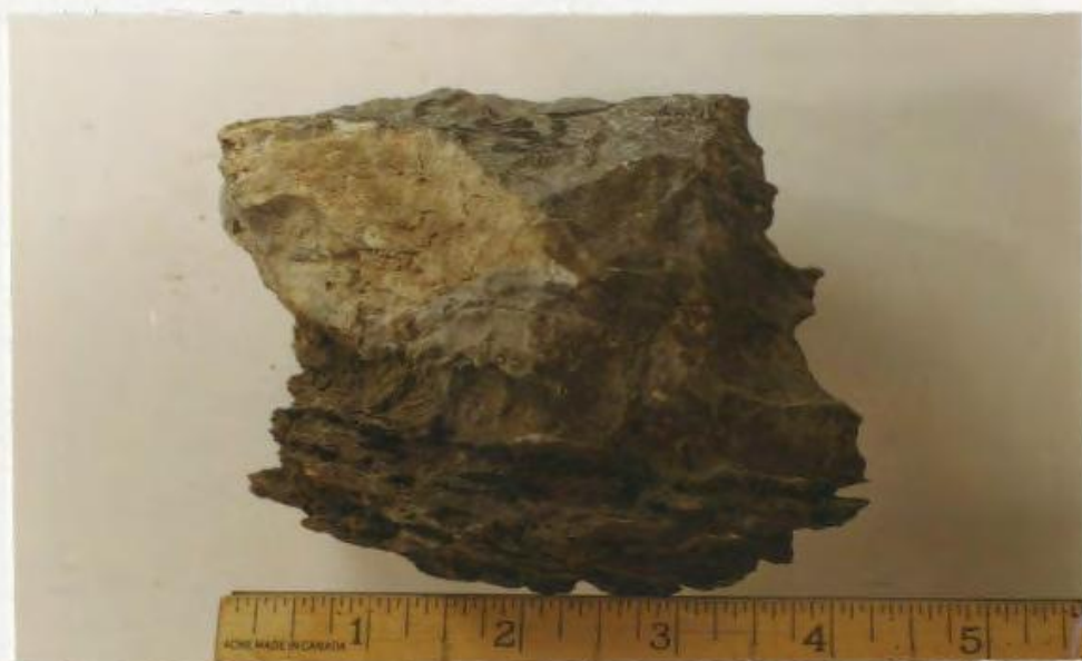
Red sandy siltstone grading into red grey impure limestone. From the middle sequence of the type section.
