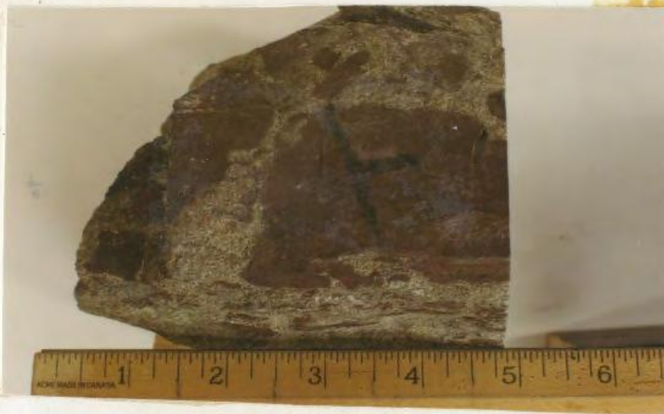
Conglomerate containing mainly red shale fragments set in an arkosic groundmass. From about the 500 foot level, east of North Bay.
