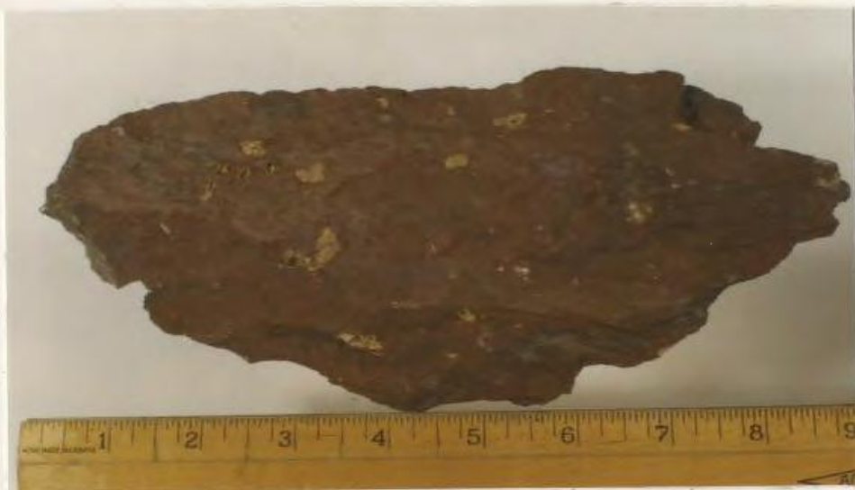
A. Mixed bed of carbonate blebs within red silt. Specimen from the lower part of the type section.
