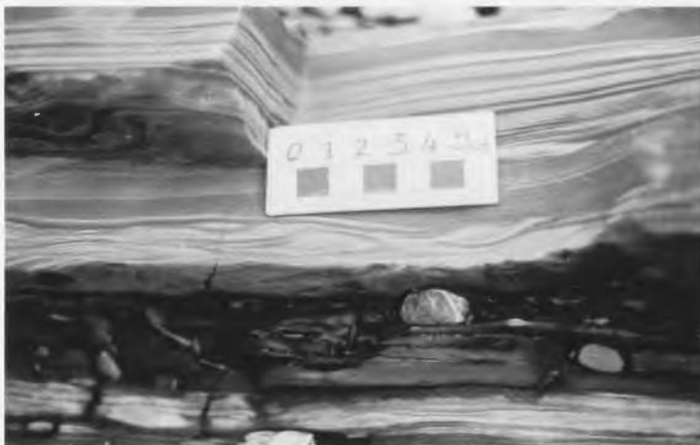
Plate 6: Dolomitic siltstone of the McKenzies formation showing asymmetric ripples. McKenzies Brook waterfall.
