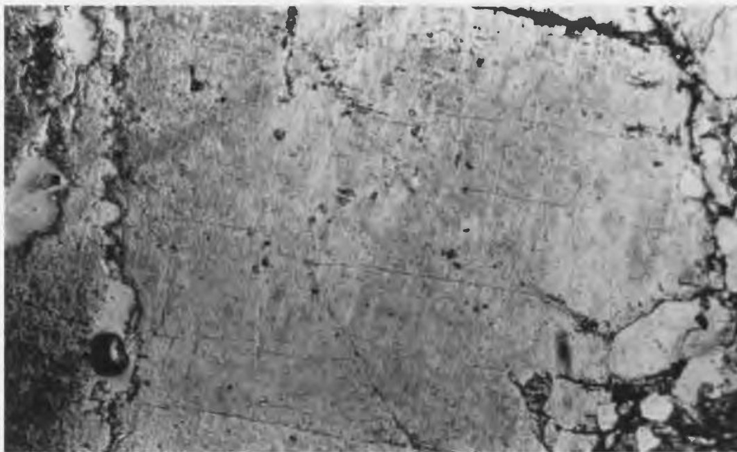
Plate 35: Feldspar in the Sellars formation which has pink appearance in the field is cloudy in thin section, probably with minute inclusions of hematite. Feldspars of this type are plagioclase since they stain pink with amaranth. Plane polarised light. Field of view 3mm.
