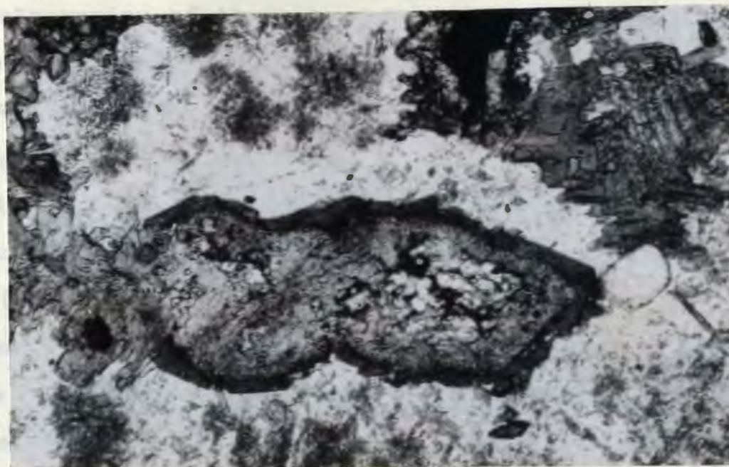
Plate-15: Photomicrograph of a mafic dyke near "Steve's Pond" (northwest), showing a fresh amphibole rim around an earlier altered amphibole. The height of the photograph represents 0.46 millimeters. (M6-23-J)
