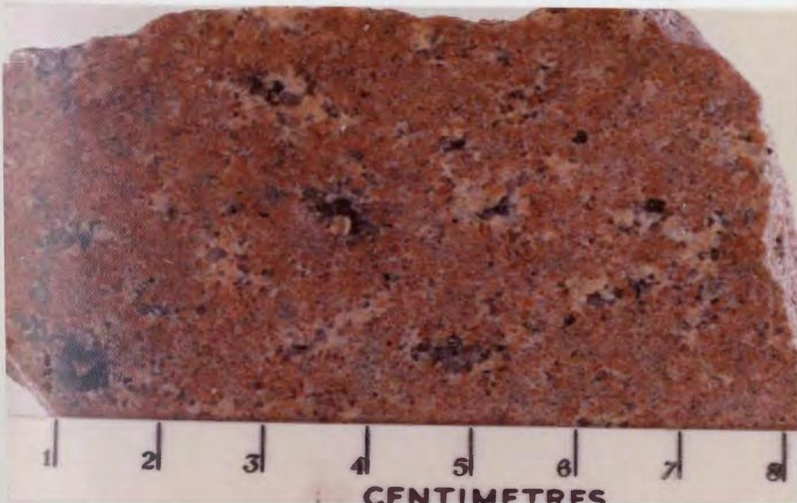
Plate 10: Pegmatitic aplite which contains numerous pegmatitic miarolitic segregations, Ackley City Showing, Sample ACD-22.
