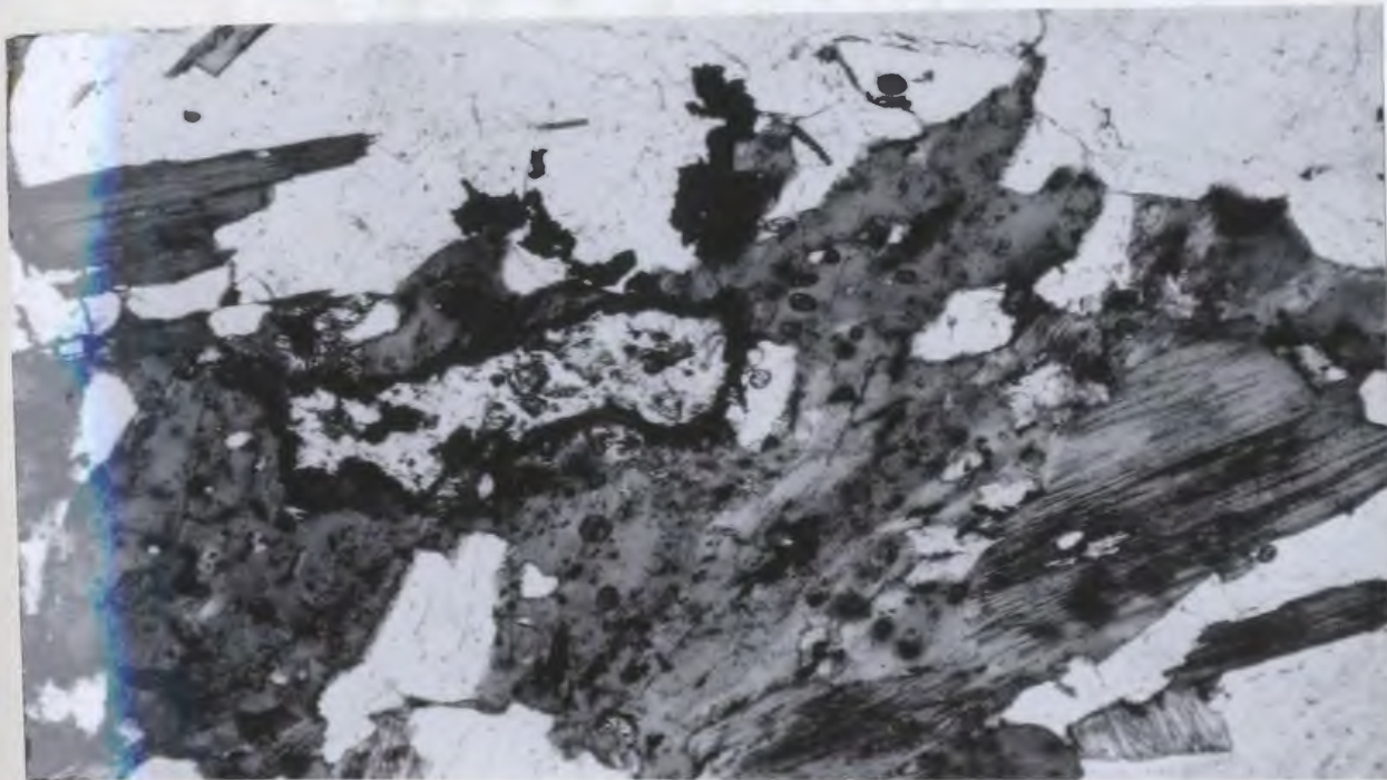
Plate 13: Secondary biotite containing numerous inclusions characterized by radioactive halos, Ackley City Showing, uncrossed nicols, X30, T.S. ACD-5.
