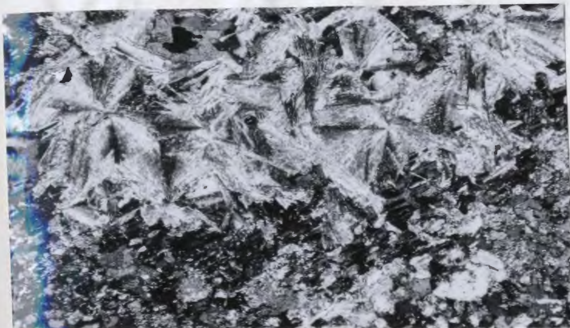
Plate 37: Coarse grained radiating felted masses of sericite completely replacing a plagioclase phenocryst in porphyritic medium grained granite, Belle Island, crossed nicols, X30, T.S. JW-10.
