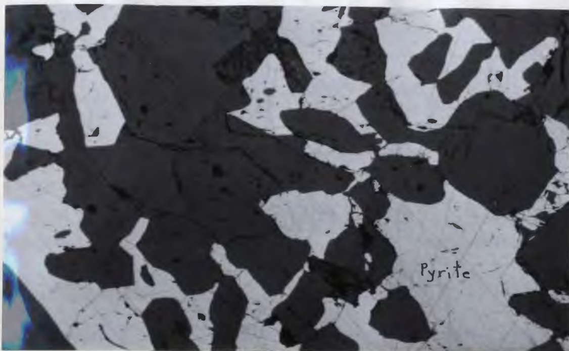
Plate 29: Part of pyrite nodule showing the dendritic nature of the pyrite which occupies quartz sites in the granite, Wylie Hill, reflected light, uncrossed nicols, X60, P.S. WH-249.
