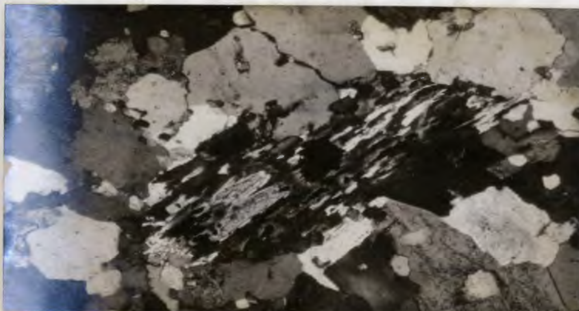
Plate 38: Biotite completely replaced by sericite-calcite-sphene-rutile-pyrite in porphyritic aplite, Belle Island, crossed nicols, X60, T.S. JW-90.
