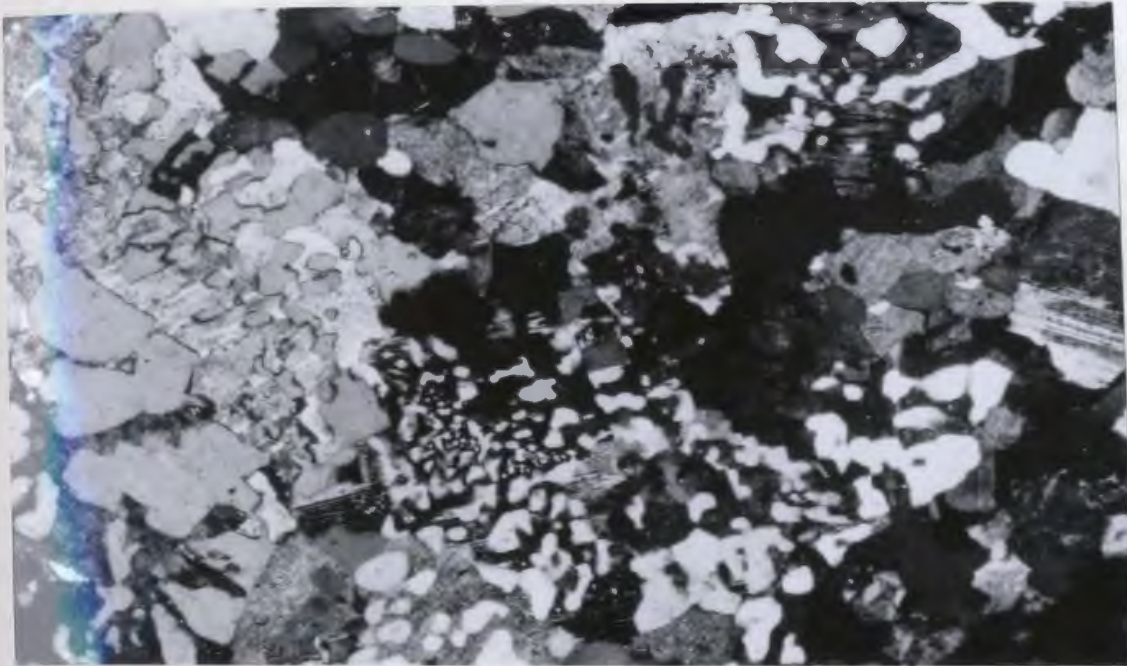
Plate 5: Coarse grained granophyric intergrowth of string perthite and quartz in medium grained granite, Motu, crossed nicols, X30, T.S. JW-99.
