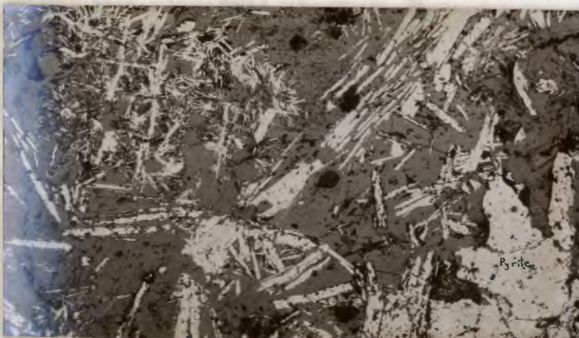
Plate 30: Fine grained platy aggregate of molybdenite disseminated in fine grained, porphyritic granite, Wylie Hill, crossed nicols, X60, P.S. WH-69-7-150.
