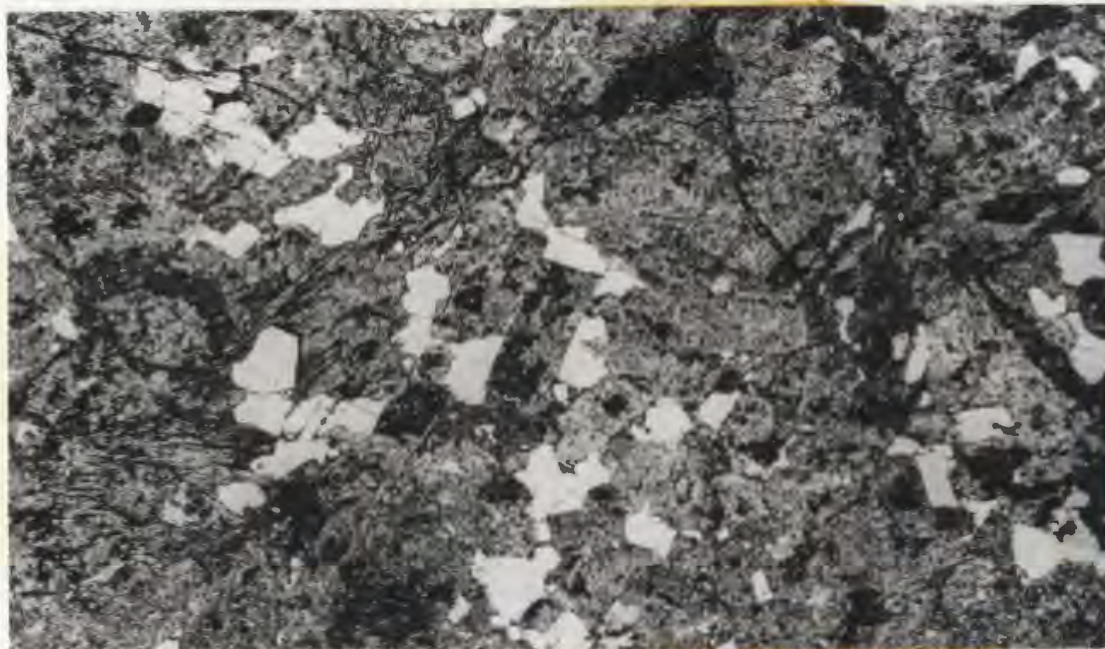
Fig. b: Quartz diorite from the Dolland Quartz Diorite, showing turbid plagioclase grey, hornblende (dark grey) and interstitial quartz (white). Locality 1000 ft. west of Dolland Arm. 2000 ft. west of Dolland Arm. Plane polarised light.
