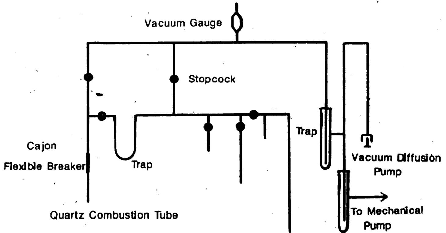
**Figure 2-2:** Gas separation line used to purify
