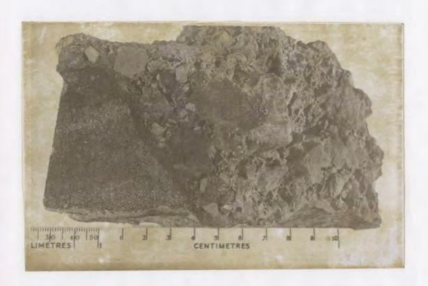
Plate 1: A sulphide float clast from the Sheffield Lake - Indian Pond Area; note Limonite rim and accretion of pebble sized andesite clasts.
