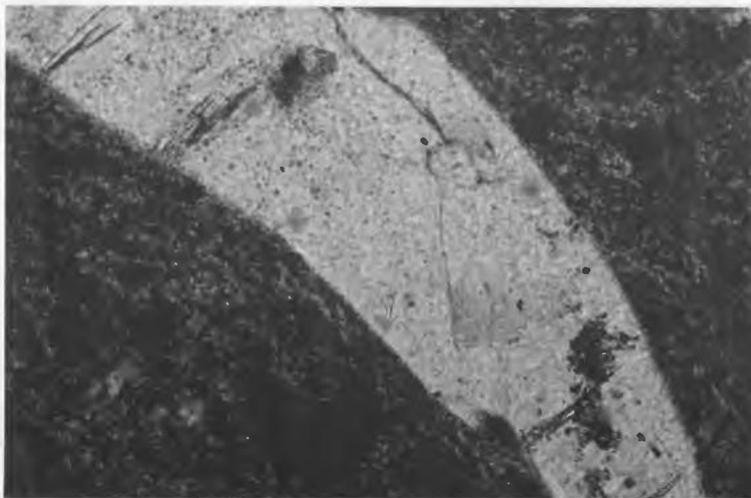
Photomicrograph 56. K-feldspar (darker grey with lower relief) spreading from fractures and partly replacing resorbed albite phenocryst. Crossed nicols; field of view approx. 3mm across. Specimen H120; central zone of welding in unit 23.
