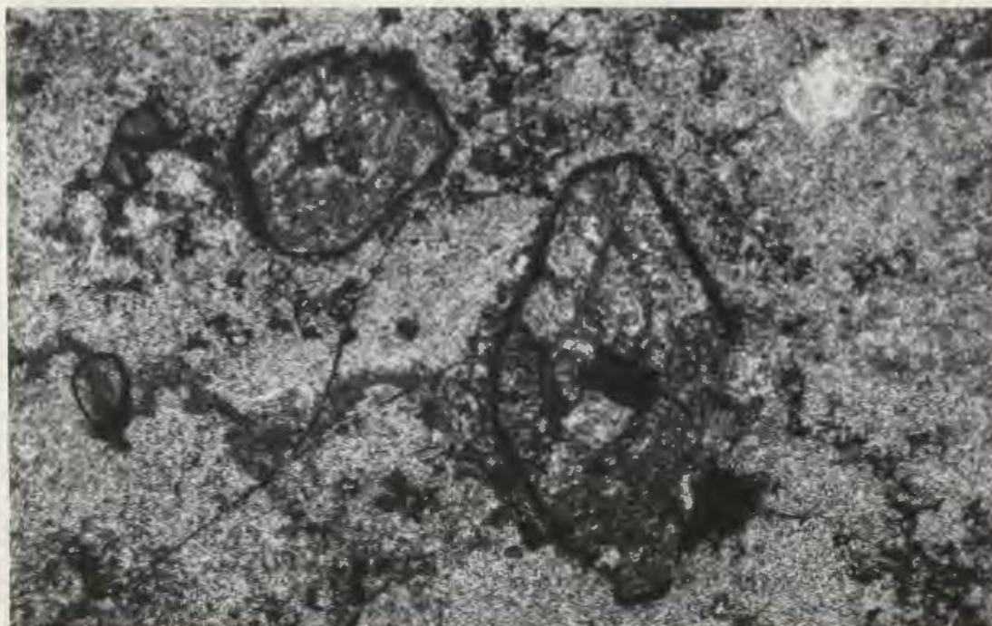
Photomicrograph 40. Subhedral amphiboles in dacite replaced by alkalic feldspar, chlorite, and clay minerals. Note amphibole cross-sections and relict cleavage. Plane-polarized light; field of view approx. 3.8mm across. Analysis GC12.
