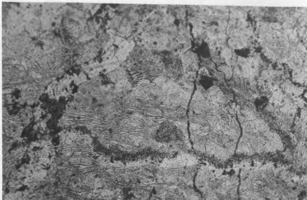
Photomicrograph 61. Veins of albite (pale grey) and epidote (dark grey with high relief) promoting recrystallisation of iron-oxide at their margins. Compare this with devitrification textures described in photomicrographs 27-31. Plane-polarized light; field of view approx. 12mm across. Specimen H110; 3ft (0.9m) above green altered vesicular base of unit 15.
