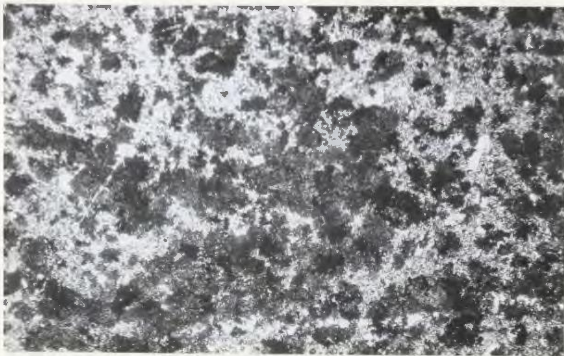
Photomicrograph 52. Intense recrystallisation of dacite to a fine-grained assemblage of "mossy" epidote (pale to dark grey), quartz, and albite (both white). Note relict feldspar phenocryst (right-centre). Plane-polarized light; field of view approx. 6.1mm across. Specimen H162; map ref. 3460,6040.
