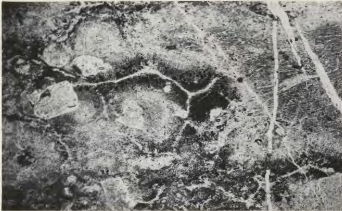
Photomicrograph 29. Same specimen as photomicrograph 27. Thin curvilinear "canals" of minor alkalic feldspar in a quartz base grade outwards into an axiolitic zone rich in iron ore, which in turn is surrounded by a zone practically devoid of opaque material. Plane-polarized light; field of view approx. 12mm across.
