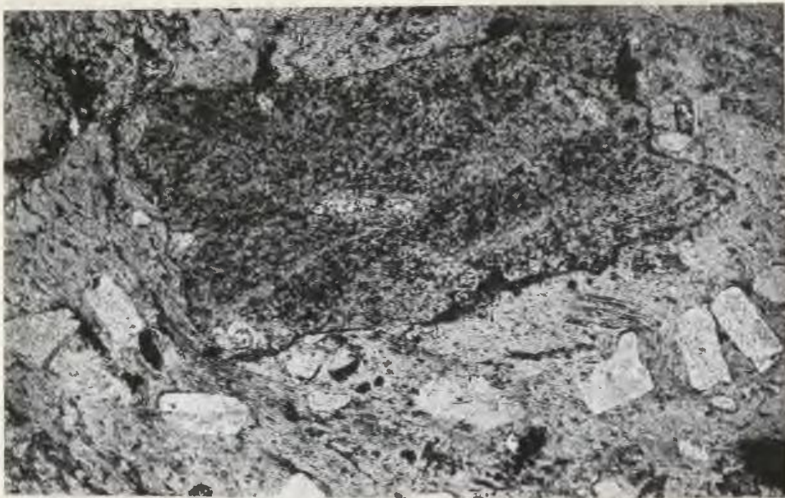
Photomicrograph 33. Incipient development of microspheralitic alkali feldspar and granophyric quartz in devitrified tuff fragment. Plane-polarized light; field of view approx. 30mm across. Specimen H183; top of unit 41.
