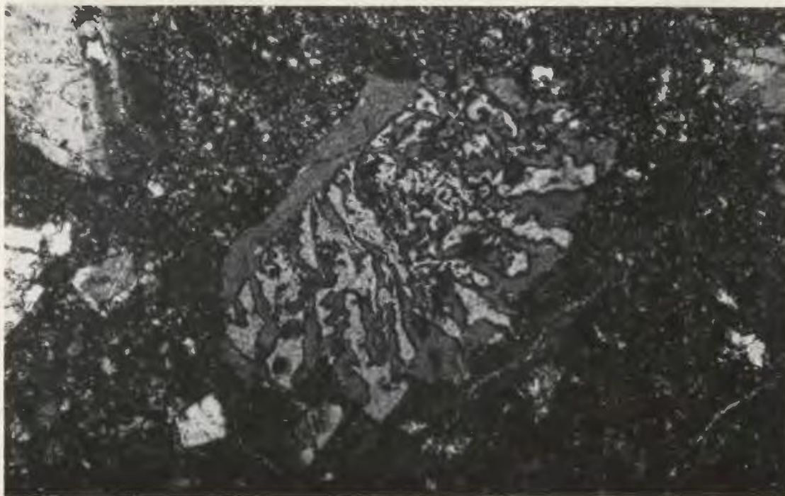
Photomicrograph 1. Granophyre xenolith enclosed in base of unit 3. Crossed nicols; field of view approx. 6.1mm across. Specimen H25.
