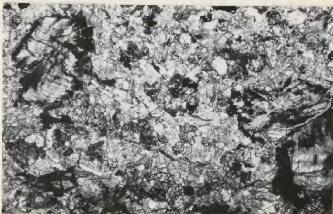
Photomicrograph 48. Olivine diabase containing subhedral olivine phenocrysts (upper right and lower left) replaced by iron-oxide (black), iddingsite (grey), and colourless to pale green serpentine (white) set in a groundmass of clinopyroxene (greyish white with high relief) and clouded albite. The clear white recrystallised areas with low relief are albite. Plane-polarized light; field of view approx. 12mm across. Analysis NX17; cf. fig. 4.
