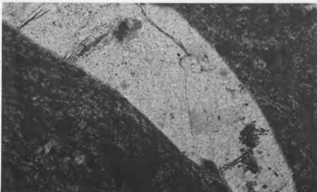
Photomicrograph 56. K-feldspar (darker grey with lower relief) spreading from fractures and partly replacing resorbed albite phenocryst. Crossed nicols; field of view approx. 3mm across. Specimen H120; central zone of welding in unit 23.
