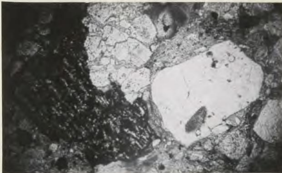
Photomicrograph 9. Partially resorbed quartz and oxidised biotite phenocrysts in sillar. Plane-polarized light; field of view approx. 7.5mm across. Base of unit 6; analyses GC38 and NX1.
