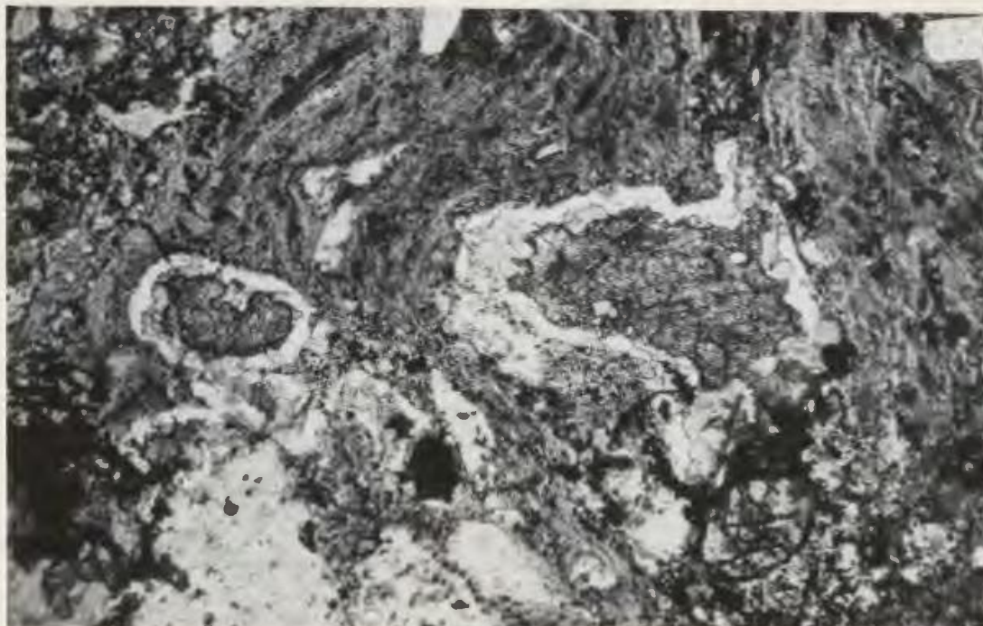
Photomicrograph 22. Same specimen as photomicrograph 20. Welding wraps around lithophysal cavities infilled with quartz (white), bladed crystals of yellow pleochroic epidote (dark grey with high relief), and minor chlorite (pale grey with lower relief). Note clinopyroxene microphenocryst (lower left). Light-coloured area at upper left is an irregular vein of albite. Plane-polarized light; field of view approx. 7.5mm across.
