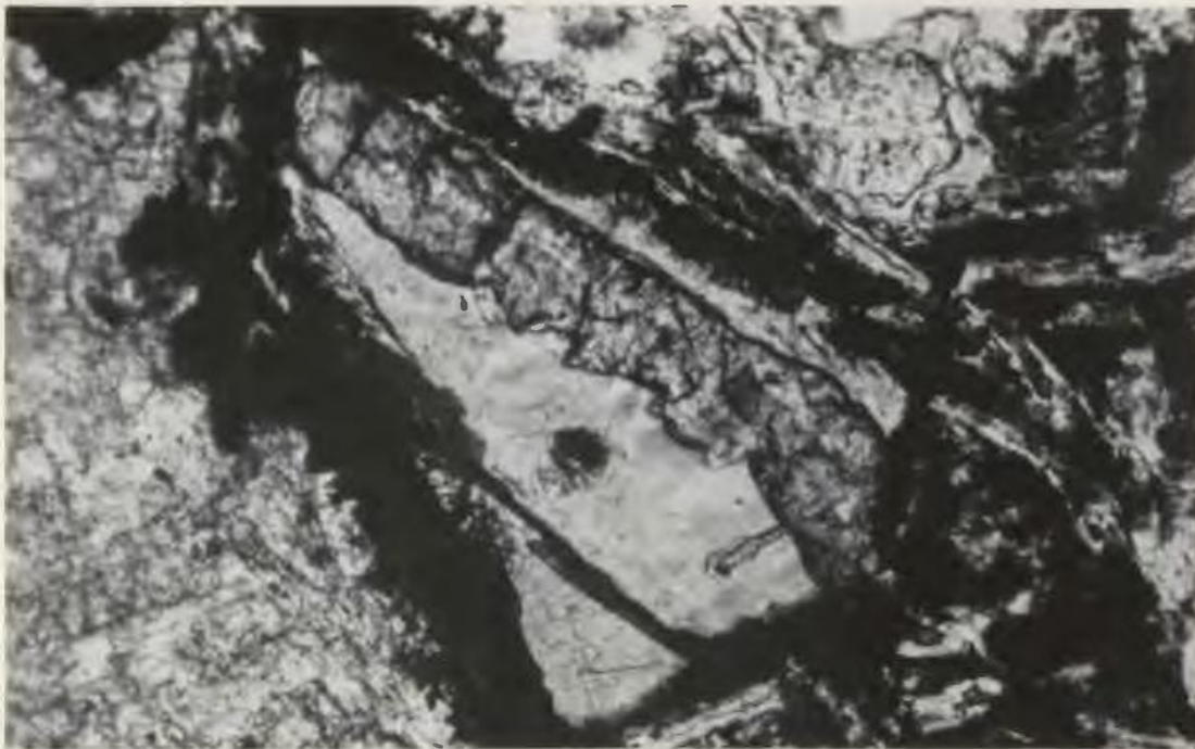
Photomicrograph 41. Groundmass olivine in mafic lava flow exhibiting a core of fresh olivine (high relief) partly replaced by yellow pleochroic serpentine (pale grey) rimmed by iron-oxide (black). Plane-polarized light; field of view approx. 1.5mm across. Analysis NX12; cf. fig. 4.
