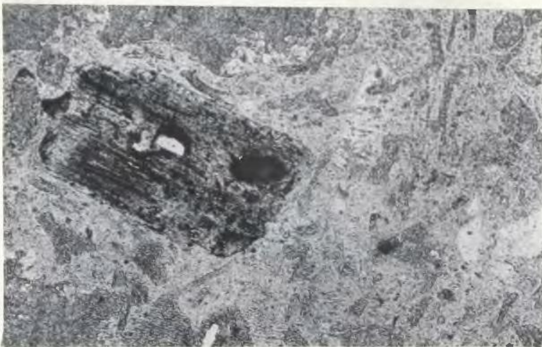
Photomicrograph 49. Green biotite phenocryst in sericitised and bleached welded tuff. Plane-polarized light; field of view approx. 6.1mm across. Specimen H82; map ref. 3410,5735.
