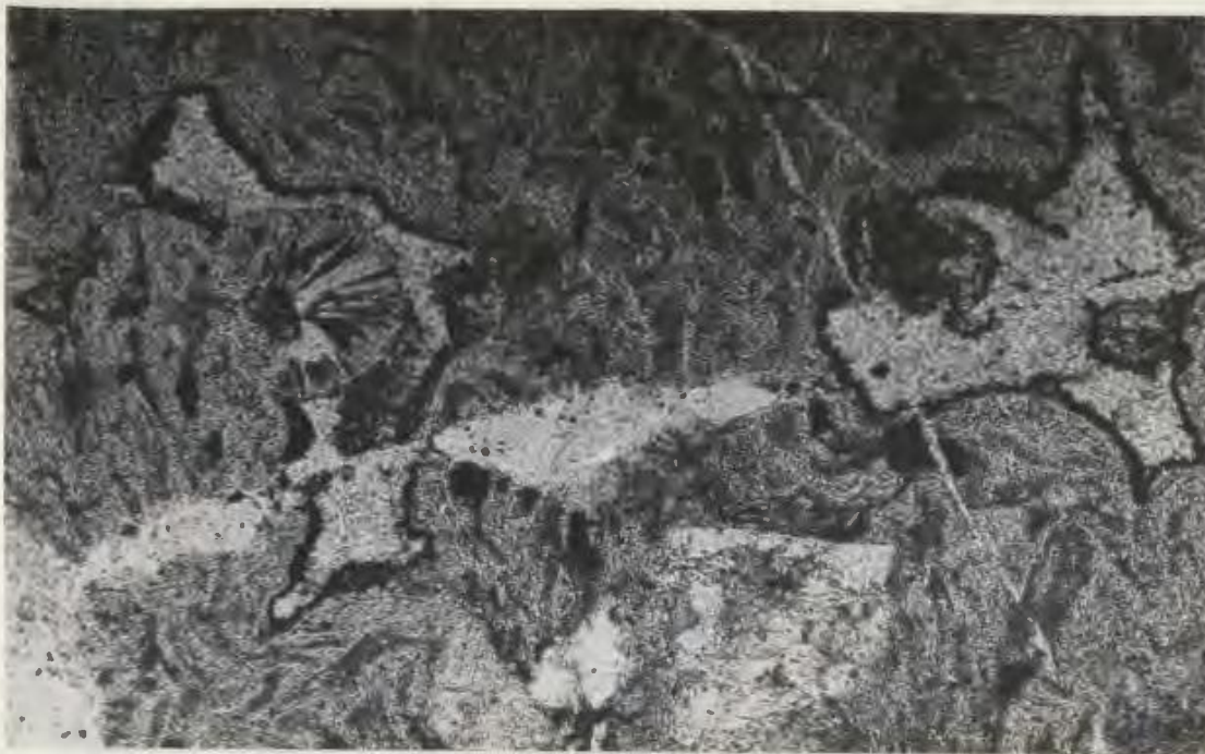
Photomicrograph 5. Altered, densely welded crystal-vitric tuff enclosing devitrified platy shards, possibly of accidental origin. Plane-polarized light; field of view approx. 7.5mm across. Specimen H93; 18ft (5.5m) above base of unit 11.
