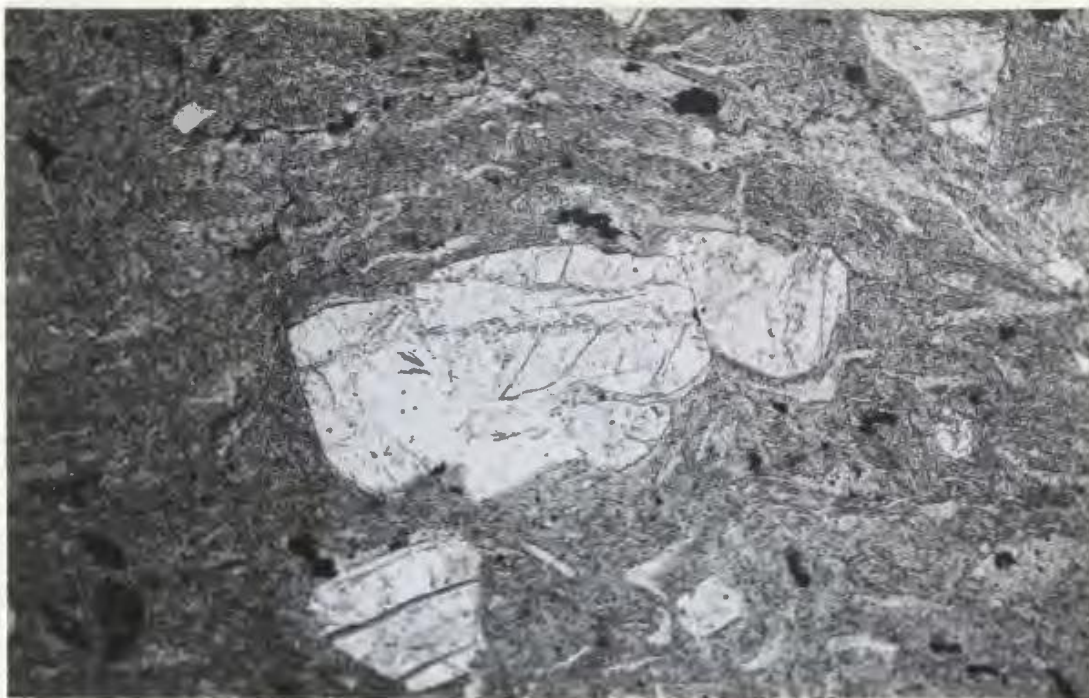
Photomicrograph 53. Incipient welding in sericitised crystal-lithic tuff. Anhedronal phenocrysts are albite. Plane-polarized light; field of view approx. 6.1mm across. Specimen H173; top of unit 40; analysis GC43.
