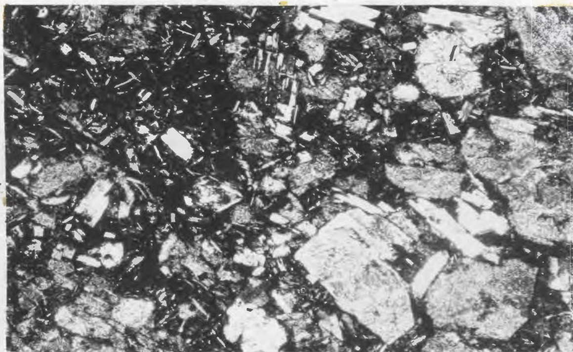
Plate 28. Saussuritized and fresh plagioclase phenocrysts, microphenocrysts and microlites in a cryptocrystalline groundmass, from the PILLOW-ANDESITE Member, Cutwell Arm area, (x38), plane polarized light.
