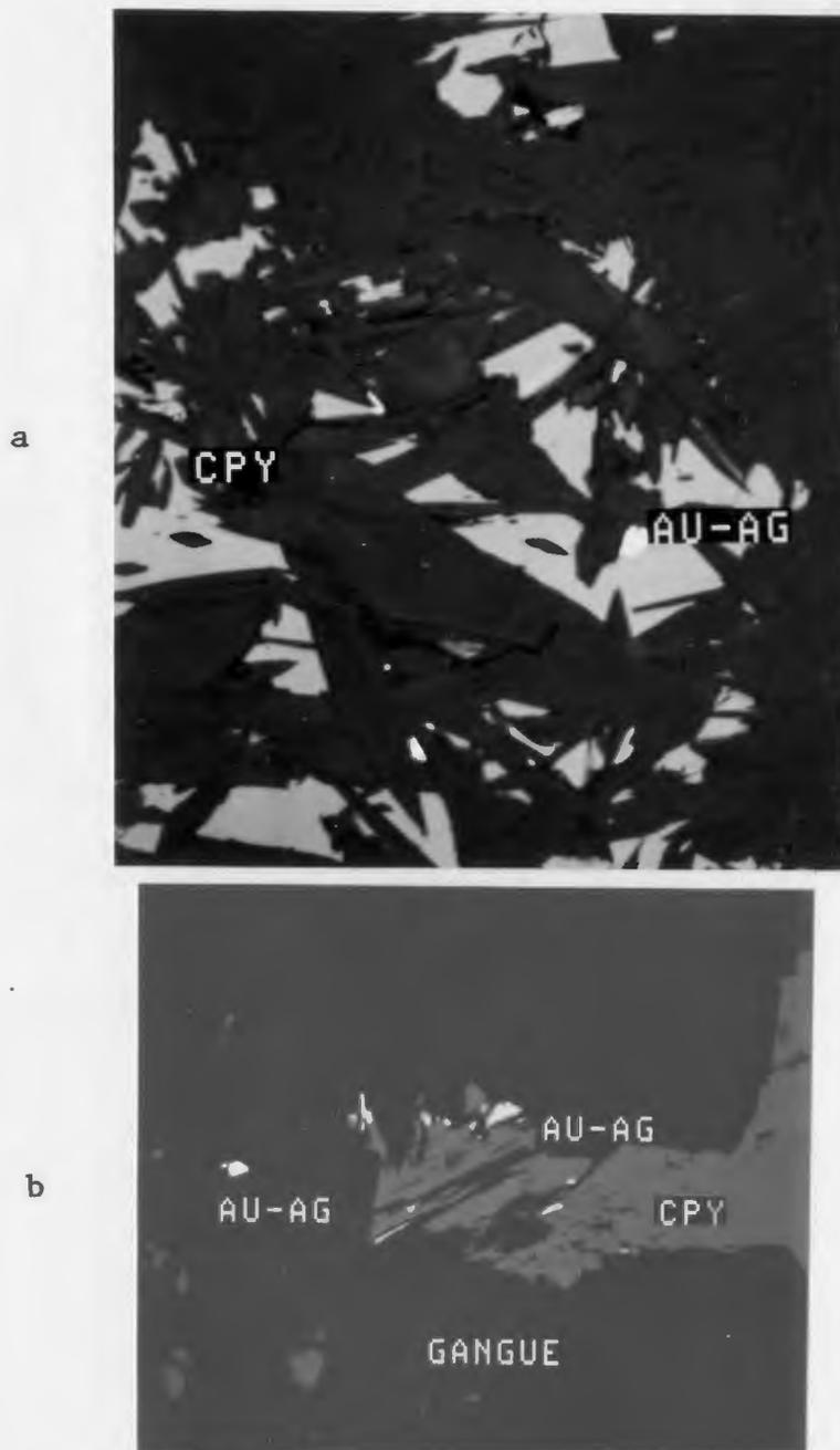
**Figure 3-13:** SEM photomicrographs of electrum grains, Burton's Pond
