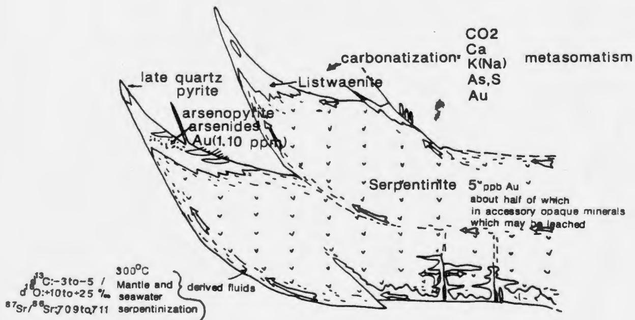
**Figure 1-4:** The listwaenite model of gold mineralization
