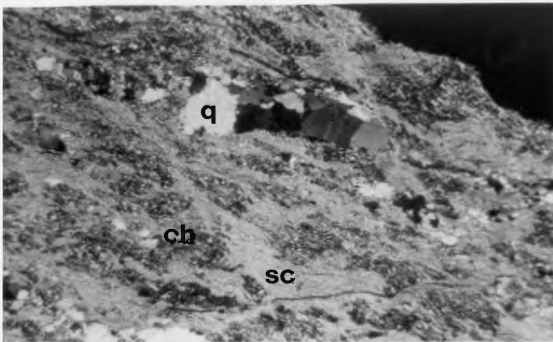
**Figure 3-18:** Photomicrograph of chlorite-sericite alteration, Gull Pond
