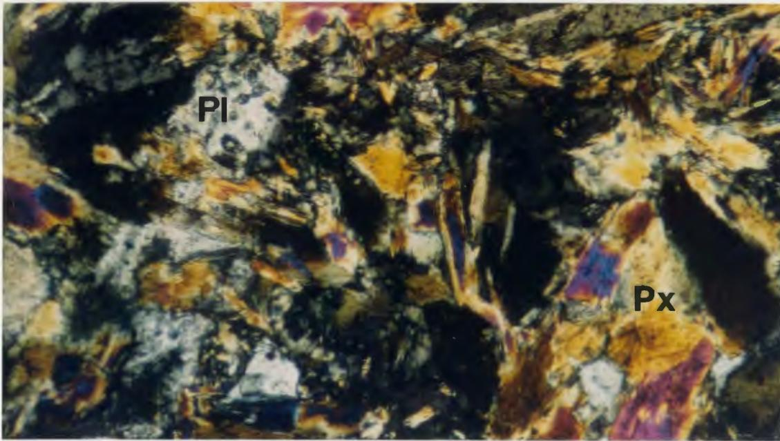
**Figure 2-6:** Photomicrograph of diabase texture Sample 21, XP, Subophitic diabase, note uralitized pyroxene laths (Px) enclosed by plagioclase (Pl). Photo width 3.3 mm. Abbreviations for this and following figures: PL-plane light, XP-cross polars, RL-reflected light.
