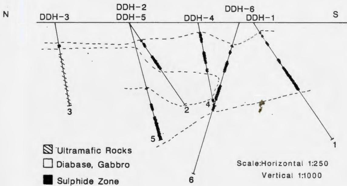
**Figure 3-6:** Subsurface geology of the Burtons Pond showing
