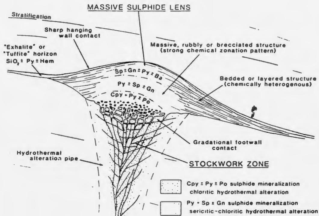
**Figure 1-3:** Essential characteristics of an idealized massive sulphide deposit
