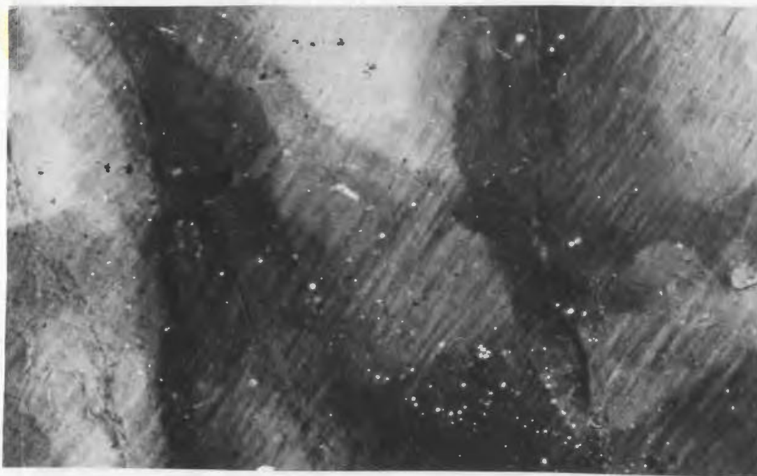
4a. Deformation lamellae in quartz. (X 120)
