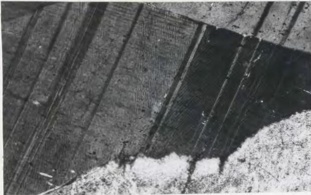
15b. Microantiperthite (or dislocation features?) in plagioclase grain from sills. (X 100)
