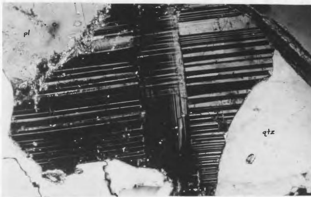
4b. Deformation lamellae parallel to kink boundary in plagioclase feldspar. (X 60)
