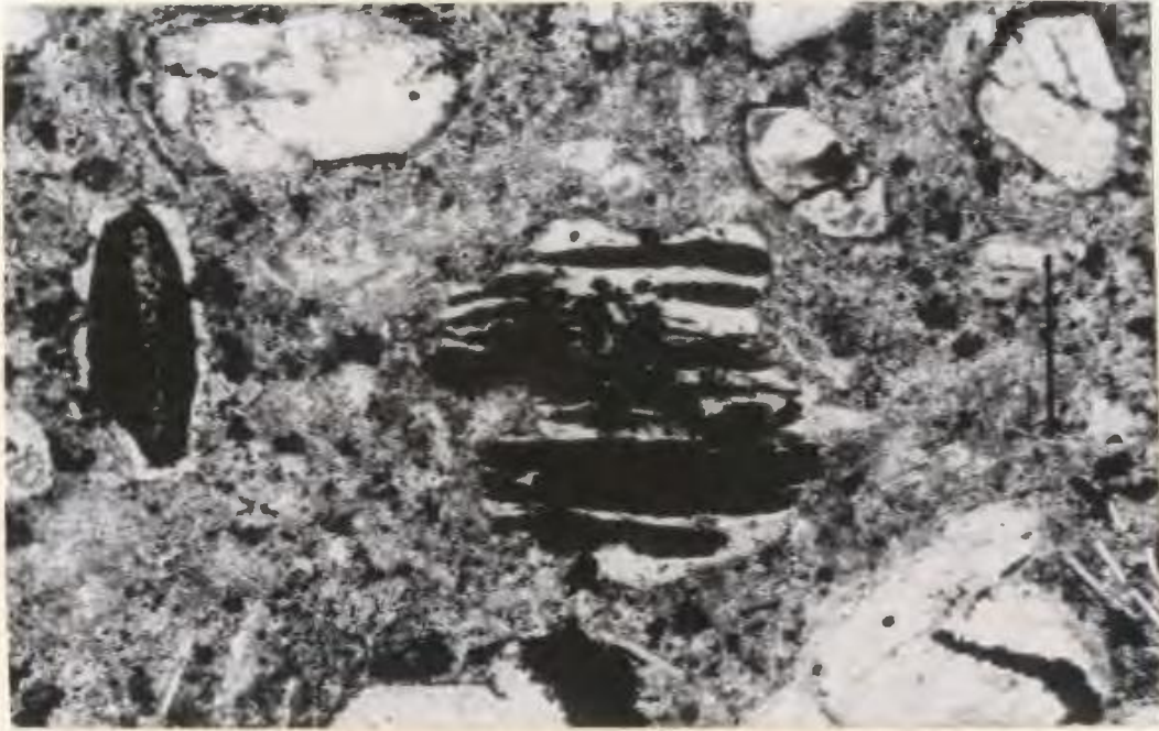
Figure 4.24 Photomicrograph of a second generation mica megacryst which contains abundant opaque oxides along the (001) cleavage. Plane light. Scale bar is 0.5 mm long.
