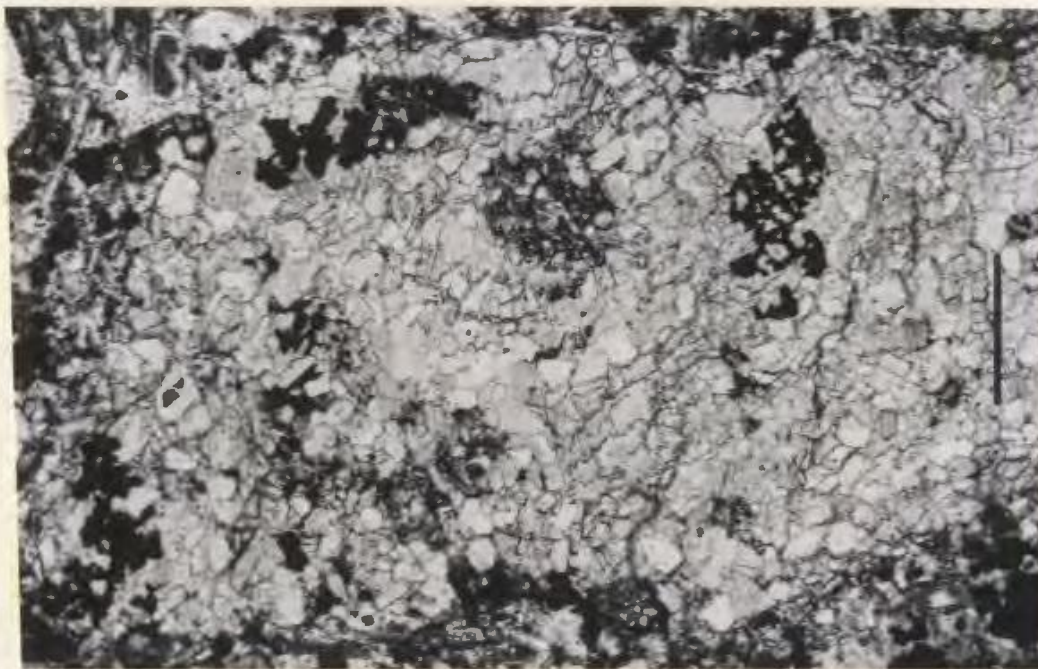
Figure 4.16 Photomicrograph of a poikilitic opaque oxide crystal in an opaque - olivine glimmerite. Plane light. Scale bar is 0.5 mm long.
