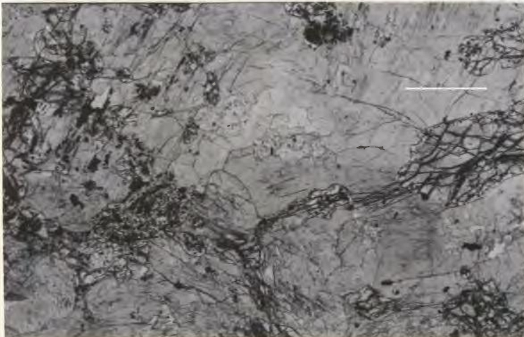
Figure 4.1 Photomicrograph of large poikilitic hornblende crystals which enclose embayed olivine and augite crystals. Note the opaque oxides along cleavage traces in the amphibole. Plane light. Scale bar is 0.5 mm long.
