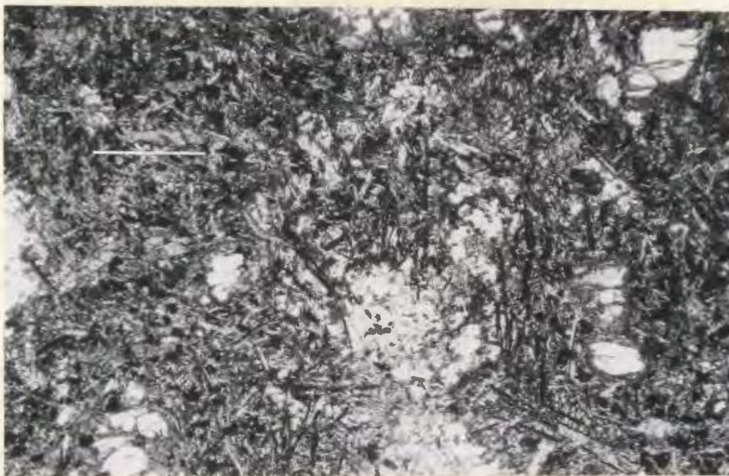
Figure 4.6 Photomicrograph showing the matrix of a carbonate-rich monchiquite composed of acicular to bladed opaque oxide growths with biotite and opaque oxides. Plane light. Scale bar is 0.5 mm long.
