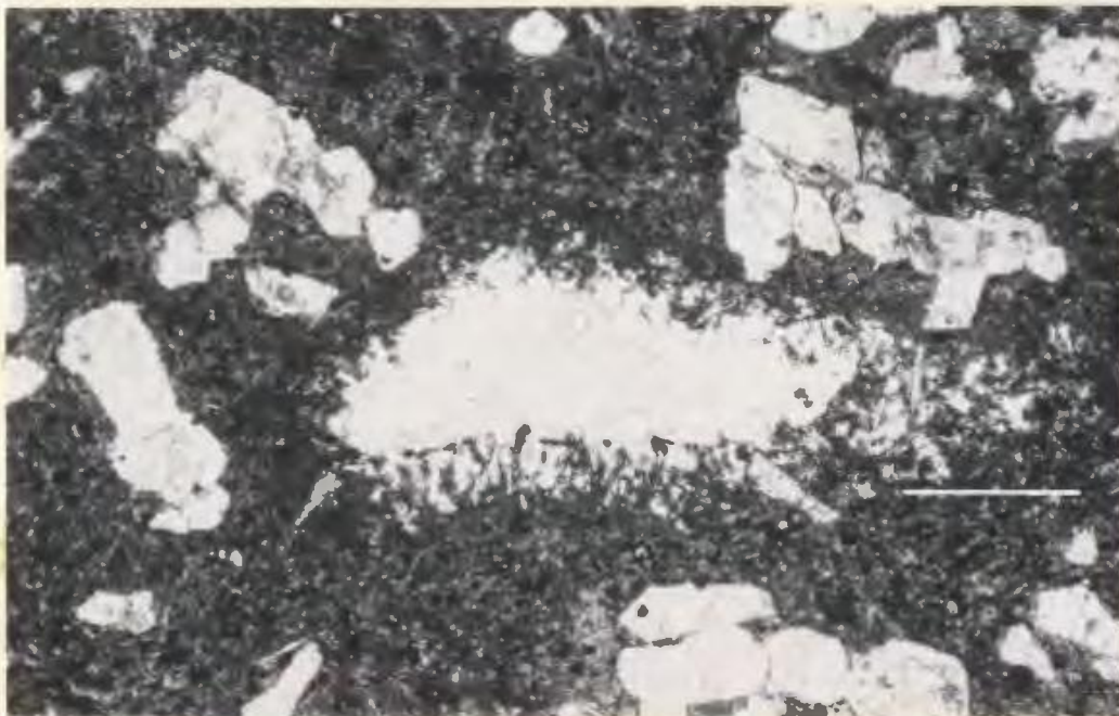
Figure 4.7 Photomicrograph showing the diffuse boundry of a carbonate-rich ocelli. This diffuse boundary is caused by the projection of augite and biotite across the ocelli wall. Plane light. Scale bar is 0.5 mm long.
