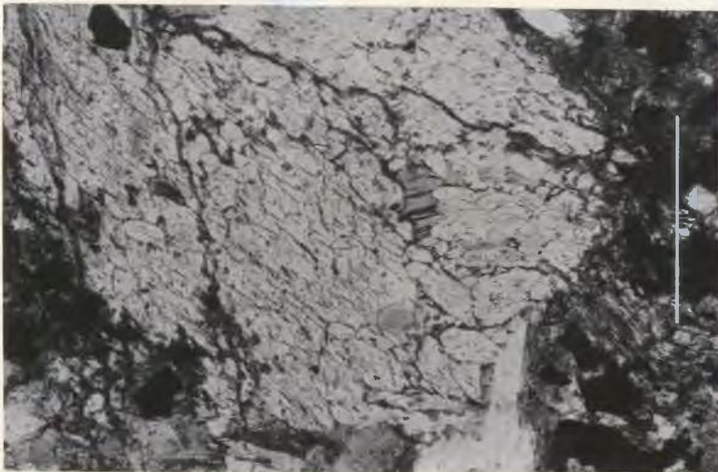
Figure 4.15 Photomicrograph of an amphibole - biotite - opaque oxide glimmerite with nonpleochroic amphibole (richterite?). Plane light. Scale bar is 0.25 mm long.
