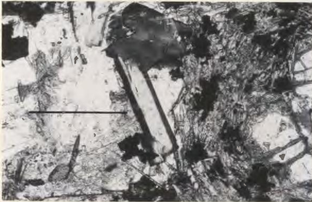
Figure 4.5 Photomicrograph showing a poikilitic tabular plate of biotite which encloses acicular needles of augite. Note the rim of dark mica around a lath of biotite just below the tabular crystal. Plane light. Scale bar is 0.25 mm long.
