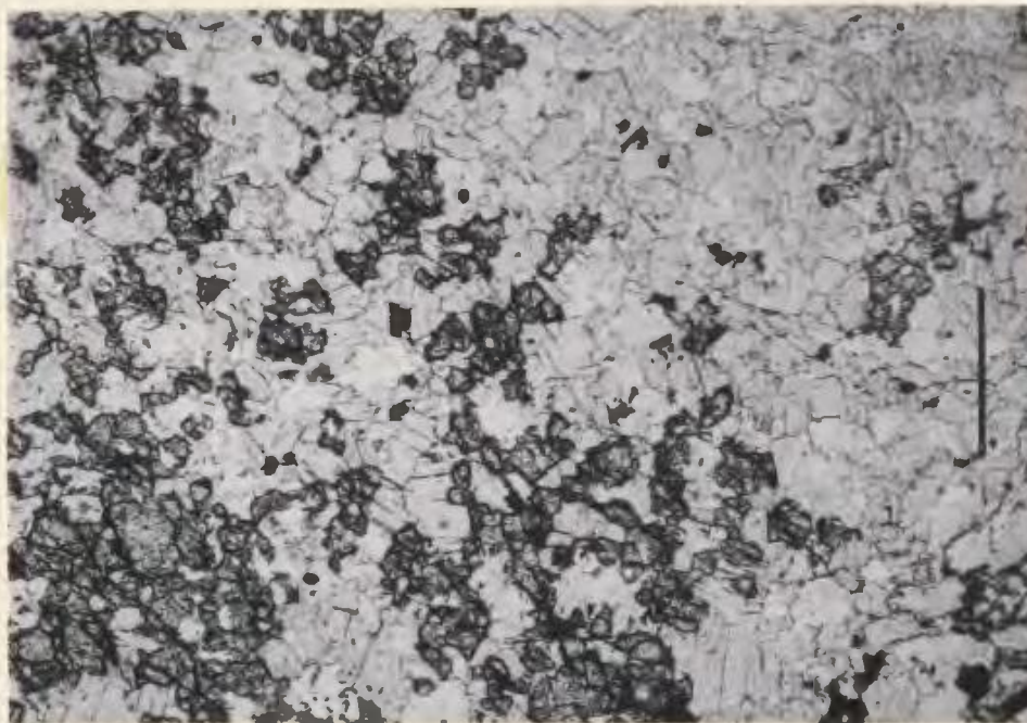
Figure 4.12 Photomicrograph showing granular olivine crystals in an olivine opaque oxide glimmerite. Note the decussate texture displayed by the mica crystals. Plane light. Scale bar is 0.5 mm long.
