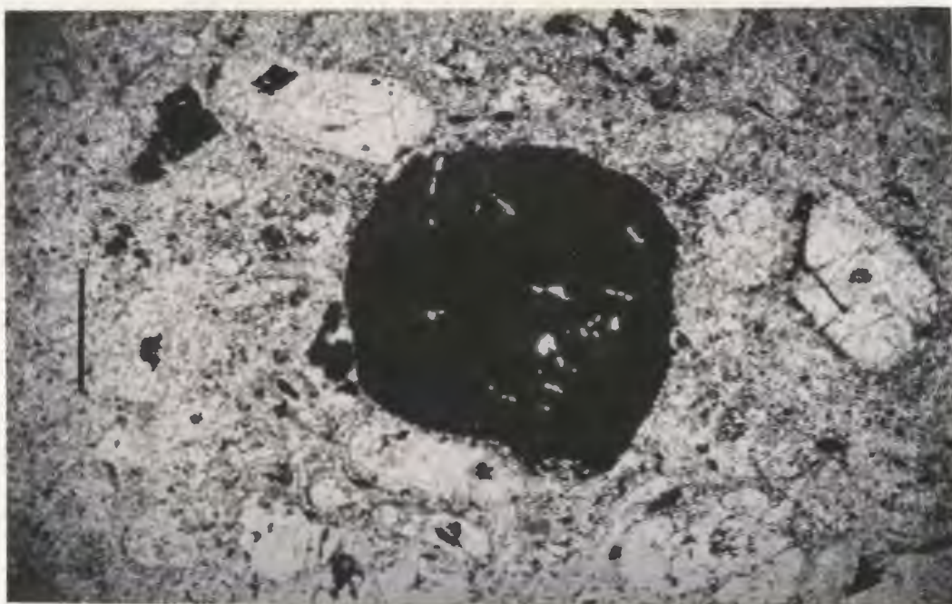
Figure 4.20 Photomicrograph of a first generation perovskite megacryst. Note the rounded grain boundary and the inclusions of carbonate. Plane light. Scale bar is 1 mm long.
