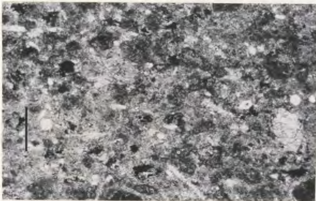
Figure 4.37 Photomicrograph of aegirine occurring as static growths within a dolomitic carbonatite (beforsite). Plane light. Scale bar is 0.5 mm long.
