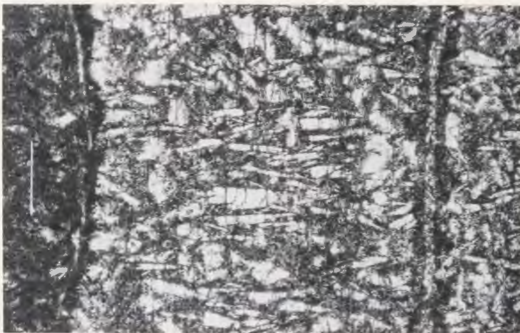
Figure 4.38 Photomicrograph of melilite which occurs as a band of perpendicular growth. Plane light. Scale bar is 0.5 mm long.
