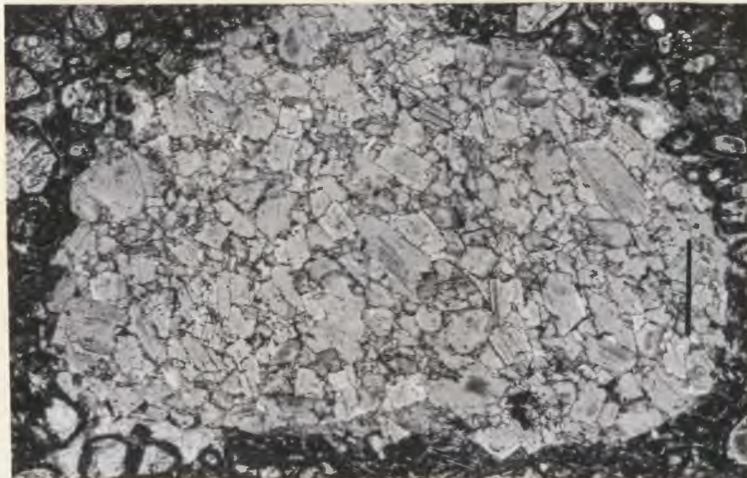
Figure 4.10 Photomicrograph of a glimmerite nodule (Group V mica) within kimberlite. The nodule is subrounded and contains interstitial granular diopside. Plane light. Scale bar is 0.5 mm long.
