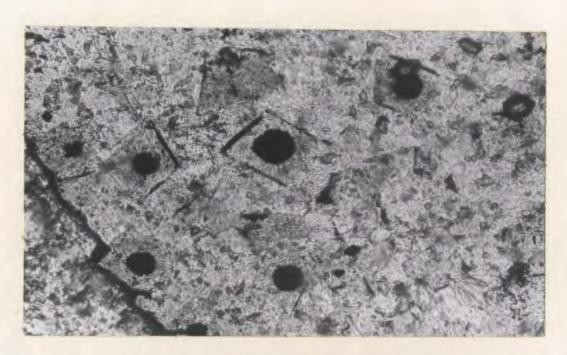
Figure 36: Rhomb-shaped pseudomorphs of some unknown gangue mineral after magnetite-2. The circular opaque mineral in the centre of the pseudomorphs is possibly mineral "X". Transmitted plane polarized light, X150.
