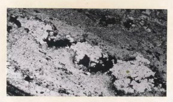
Figure 25: "Pinch and swell" structure shown by quartz (pitted white) in chloritic cordierite rock. The "necks" are filled with sulphides (black). Transmitted plane polarized light, X45.
