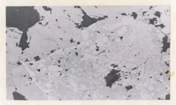
Figure 49: Remnant segments of large pyrite-2 crystal (grayish white) that was replaced by chalcopyrite and pyrrhotite (light gray). Reflected plane polarized light, X125.
