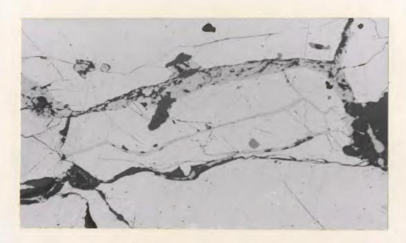
Figure 38: Pyrite-2 (grayish white) fractured by cataclastic deformation. The fractures are filled with chalcopyrite (light gray). Reflected plane polarized light, X125.
