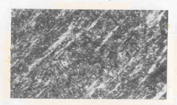
Photomicrograph of quartz-sericite phyllite showing the main schistosity S<sub>1</sub>, which was crenulated by a later deformation that gave rise to the strain-slip schistosity S<sub>2</sub> (running northeast). Transmitted light, Crossed nicols, X60.
