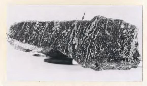
Figure 29: Ribboned ore showing "ribbons" of sulphide (white) and gangue (medium and dark gray). Arrow indicates the direction of foliation which runs parallel to the ribbons'. Length of specimen, 6 inches.
