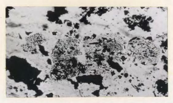
Figure 33: Some unknown mineral pseudomorphous after magnetite-2 (rhomb-shaped). The thin opaque lamellae are of ilmenite. Transmitted plane polarized light, X45.
