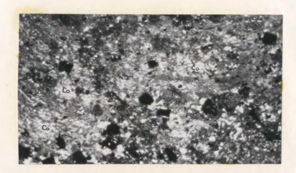
Figure 12: Crenulated patches and poorly defined bands of cordierite (Co) in cordierite-bearing silicic tuff. The banding is clearer on the western margin of the microphotograph.
