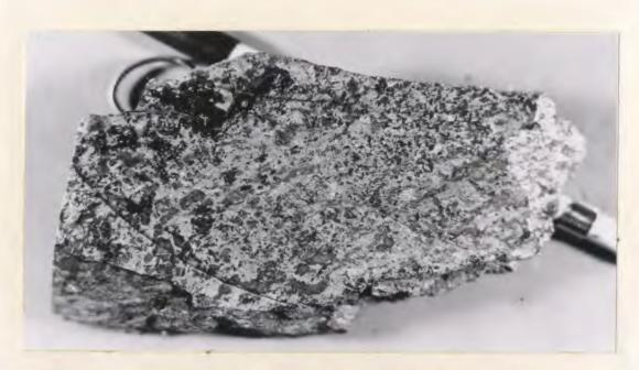
Figure 28: Massive ore showing preferred orientation (running almost northeast). Dark and medium gray is gangue; grayish white is chalcopyrite and pyrrhotite. Length of specimen 4 inches.
