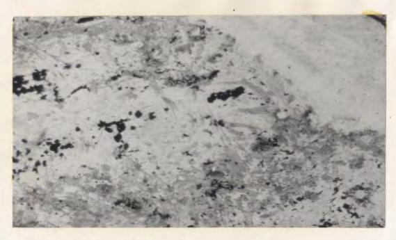
Figure 27: Anthophyllite fibers (medium gray) occurring subpoikilitically within cordierite grains (grayish white). Transmitted plane polarized light, X25.
