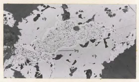
Figure 41: Pyrite-4 (pitted surface) surrounded by a thin rim of pyrite-2(?) (py). The whole grain occurs in a groundmass of chalcopyrite (cp). Reflected plane polarized light, X250.
