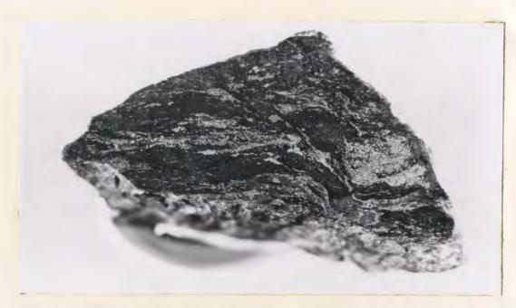
Figure 30: Ore-bearing chloritic cordierite rock showing moderately bent lenticular units of sulphides (white). Specimen about natural size.
