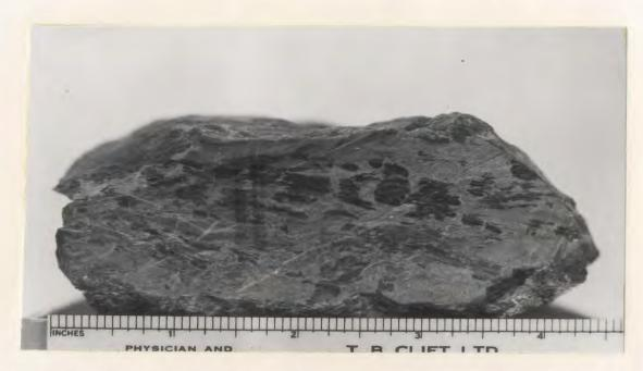
Figure 20: Cordierite-bearing silicic tuff. The discontinuous and slightly crenulated units (dark gray) consist of cordierite.
