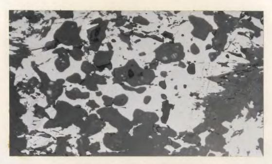
Figure 42: Pyrrhotite (white) filling intergranular spaces among quartz grains (dark gray). Reflected plane polarized light, X125.
