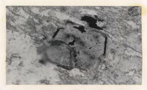
Figure 32: Magnetite-2, almost completely replaced by some unknown gangue mineral, showing its overgrowth on the northwest-trending S<sub>1</sub> schistosity. The unreplaced lamellae (black) are probably of ilmenite. Transmitted plane polarized light, X60.
