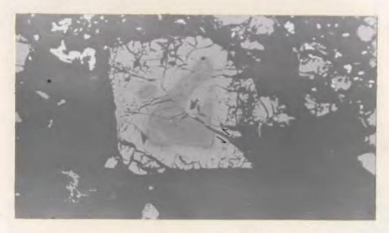
Figure 37: Disrupted grain of magnetite-2 (light gray) containing islands of mineral "X" (medium gray). Arrows indicate the direction of relative movement during disruption. Reflected plane polarized light, X200.
