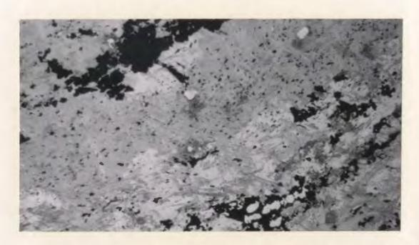
Figure 24: Cordierite-anthophyllite rock showing the growth of anthophyllite fibers (light gray, southeastern part) across northeast-trending ilmenite-hematite trails, the latter are the probable representatives of S<sub>1</sub>. Note that the bands of sulphides run parallel to these trails. Transmitted plane polarized light, X20.
