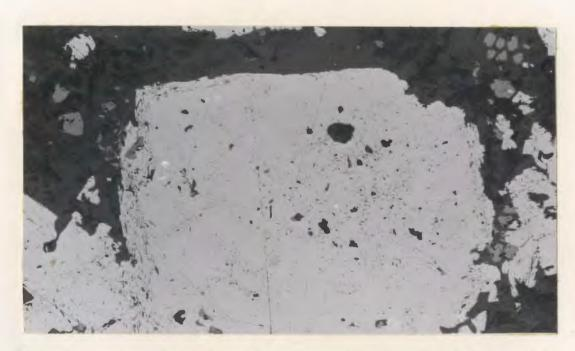
igure 40: A square-shaped grain of pyrite-2. Pyrite-3, which grew through the replacement of anthophyllite, occurs along the left and right margins of this grain. Reflected plane polarized light, X200.
