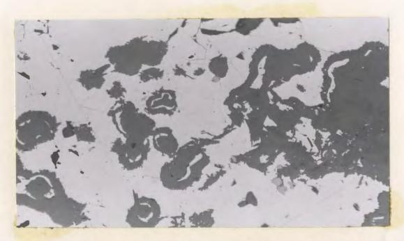
Figure 46: Mutual boundaries (?) texture between sulphides (chalcopyrite, pyrrhotite) and silicates (dark gray) in a sample that occurs within 3 feet of the contact of a post-ore diabase dyke.
