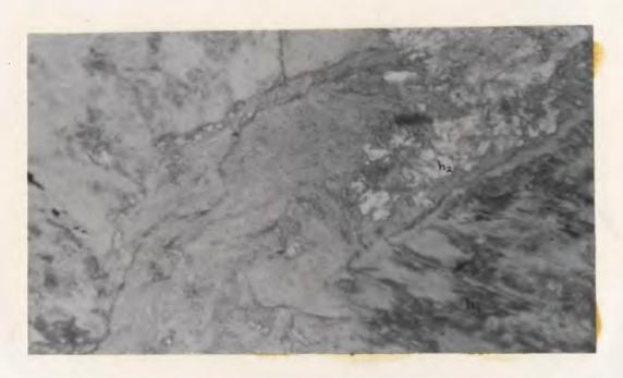
Figure 13: Greenstone showing whispy anhedral units of hornblende-1 (h<sub>1</sub>) that define S<sub>1</sub> in the rock, and subhedral grains of hornblende-2 (h<sub>2</sub>) that overgrew S<sub>1</sub>. Transmitted plane polarized light, X15.
