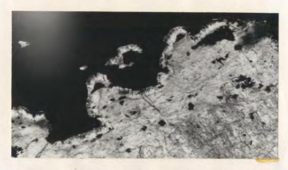
Figure 18: Reaction-rim chlorite (chlorite-3) occurring at the contact of chloritized cordierite (grayish white) and sulphide (black). Transmitted plane polarized light, X45.
