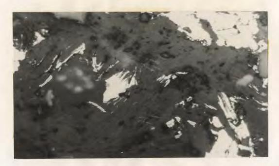
Figure 17: Crenulated acicules of chlorite-2 replaced by chalcopyrite (white). Reflected plane polarized light, X250.
