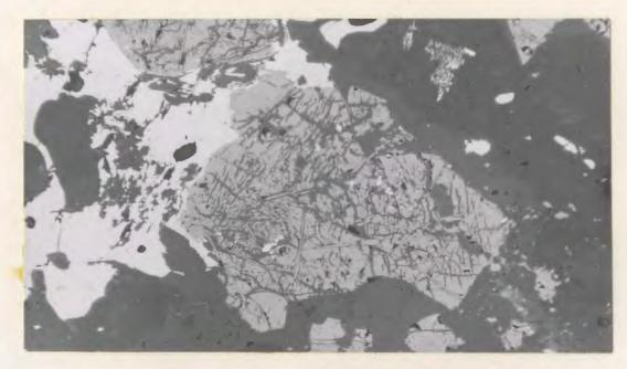
Figure 34: Ilmenite lamellae occurring in magnetite-2 (medium gray). The latter is partly replaced by gangue. Reflected plane polarized light, X125.
