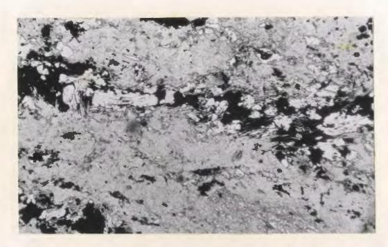
Figure 16: Crenulated acicules of chlorite-2 associated with sulphide bands (black). The chlorite acicules occur around the large patch of massive chlorite, which has a west-northwesterly elongation (lower part of the picture). Transmitted plane polarized light, X15.
