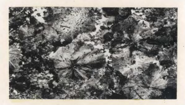
Figure 23: Spherulitic felsite dyke. The almost circular spherulites consist of feather-like units, the latter showing a micrographic texture. Transmitted light, Crossed nicols, X15.
