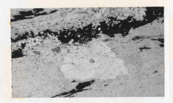
Figure 11: Growth of cordierite (C<sub>0</sub>) over ilmenite-hematite trails (medium-gray specks) that probably represent S<sub>1</sub> within the ore zone. In the northwest corner of the microphotograph the elongated streaks of sulphide run parallel to the adjacent ilmenite-hematite trails. Transmitted plane polarized light, X25.
