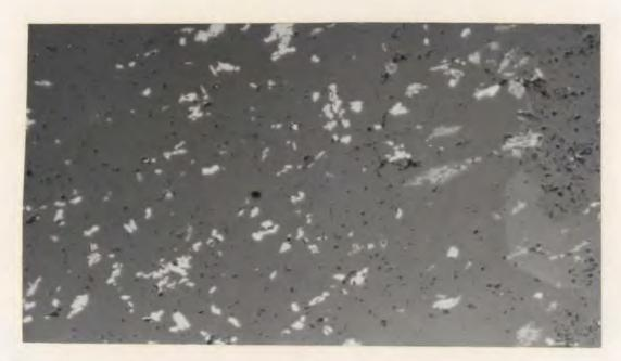
Figure 35: Very weakly defined trails of ilmenite-hematite (white) trending almost northeast. These are the probable representatives of S<sub>1</sub> within the ore zone. Reflected plane polarized light, X125.
