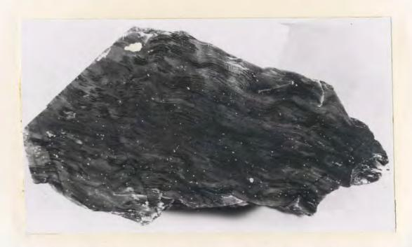
Figure 19: Crenulated silicic tuff. The darker laminae are richer in chlorite. White specks are pyrite. Length of specimen, 6 inches.
