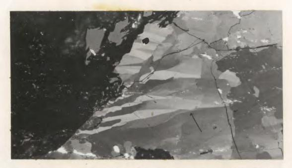
Figure 48: Deformation lamellae (grays of various shades) in pyrrhotite that have almost an east-west trend. The grain boundaries of pyrrhotite grains run roughly towards north-northeast. Arrow indicates the crossing of pyrrhotite grain boundary by the lamellae. Reflected light, crossed nicols, X125.
