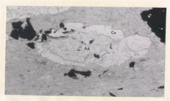
Figure 26: Andalusite (Ad) showing a corroded outline and occurring within cordierite (Co). Transmitted plane polarized light, X50.
