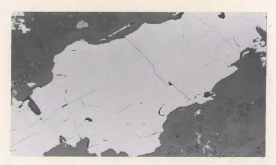
Figure 47: Exolved (?) spindles of chalcopyrite (trending northeast) in pyrrhotite. Reflected plane polarized light, X125.
