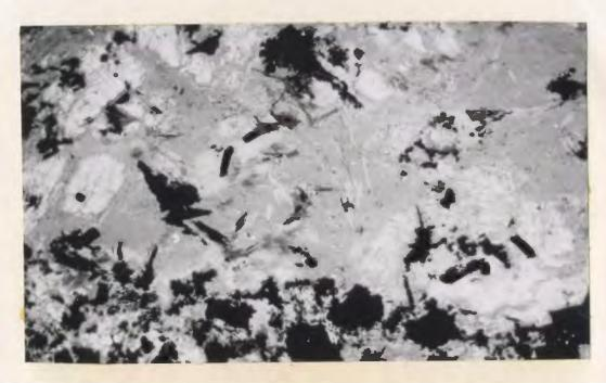
Figure 15: Chloritic cordierite rock showing the partly altered cordierite patches (grayish white) in a groundmass of massive chlorite (medium gray). Note that the sulphides (black) replace only chloritized parts of the cordierite grains. Transmitted plane polarized light, X15.
