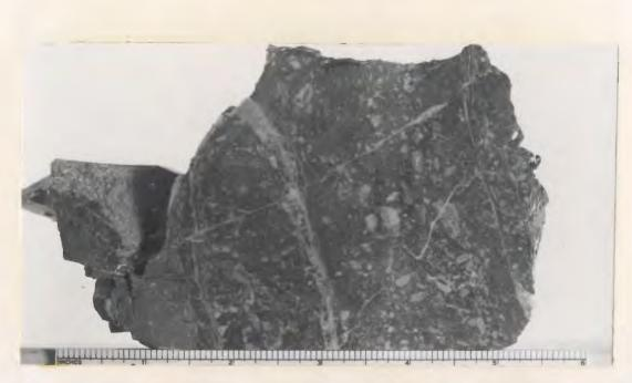
Figure 22: Lapilli tuff (?). Angular fragments of calcite and volcanic (?) rock occurring in a predominantly chloritic groundmass. The irregular veins are of calcite.
