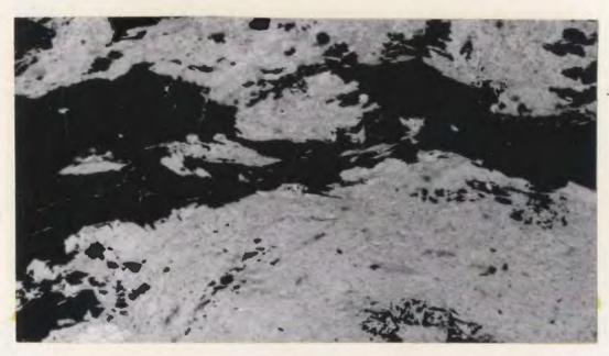
Figure 43: Massive chlorite (light gray) foliated parallel to the elongated streaks of sulphides (black). Transmitted plane polarized light, X45.
