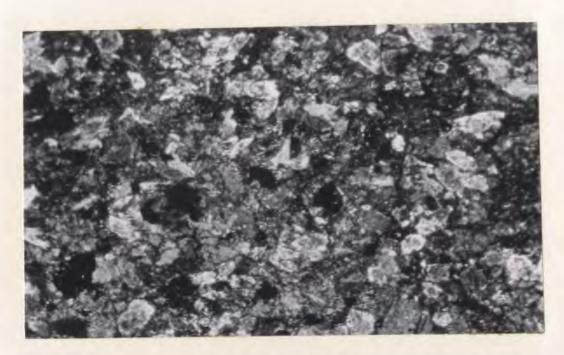
Figure 14: Non-amygdaloidal metabasalt containing laths of hornblende-2 (grayish white) and altered plagioclase (somewhat pitted) with diffused outlines. Transmitted plane polarized light, X15.
