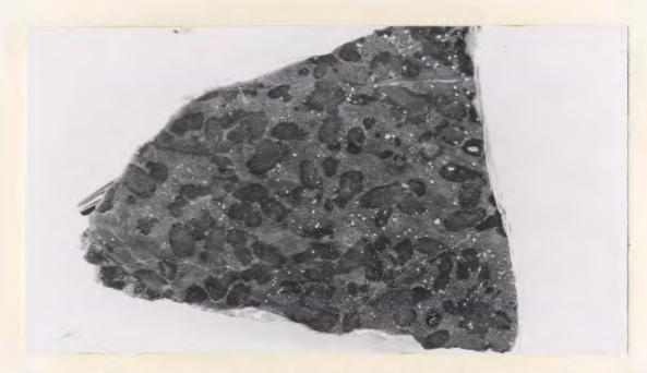
Figure 21: Cordierite-spotted silicic tuff. The randomly oriented cordierite porphyroblasts (dark gray) occur in a quartz-rich groundmass (medium gray). Length of specimen, 5 inches.
