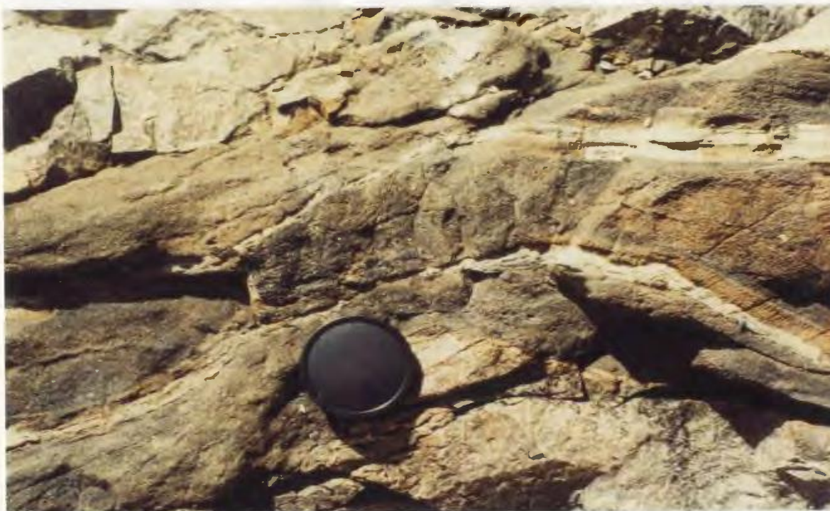
Figure 2-10: Multiple intrusion in kimberlitic dyke. The carbonate-rich selvage to the later intrusion is taken to be evidence for a volatile-rich precursory fluid. Mica is concentrated in the latest intrusion head, showing it to be volatile enriched.
