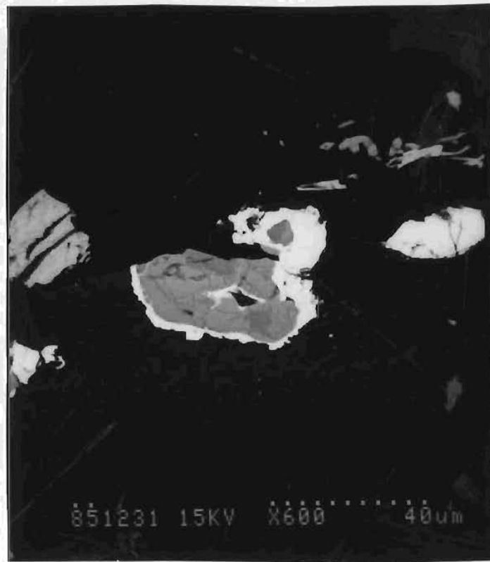
Figure 4-11: A SEM back scatter image of a zircon crystal (grey) with a pitchblende core and rim (white), from a fluorite vein. Pitchblende also occurs as individual grains (white) associated with flakes of molybdenite (med. grey).
