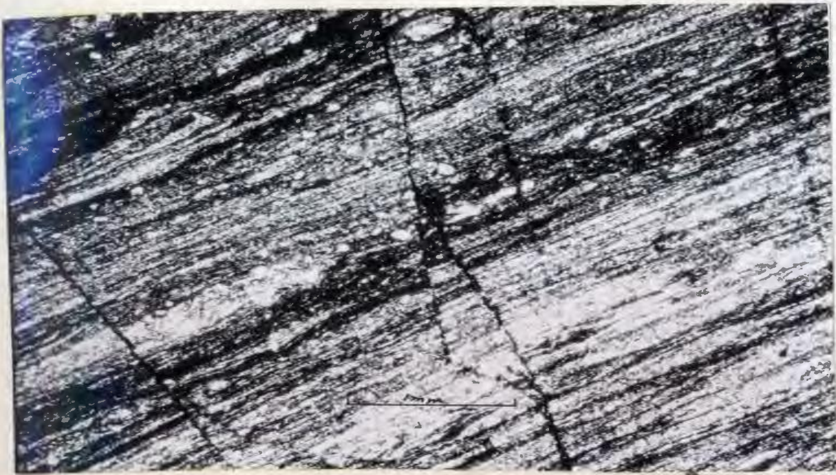
Plate 18. Mylonitic granite with small porphyroclasts of feldspar in a fine-grained to microcrystalline matrix of recrystallized quartz and feldspar.
