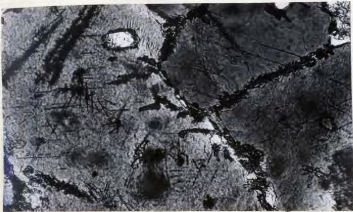
Plate 14. Sagenitic texture shown by rutile in flakes of biotite.
