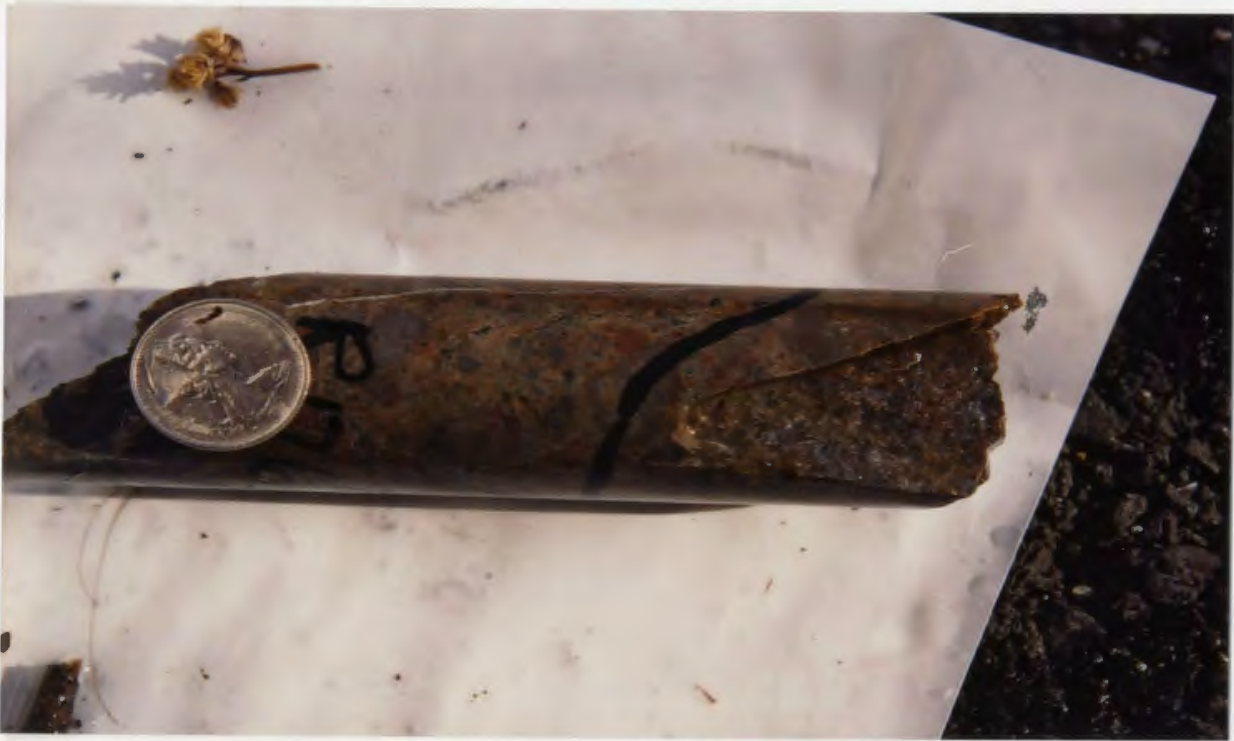
Plate 7: Drill core sample of rhyolite crystal, lapilli tuff comprising quartz and K-feldspar crystal fragments and rhyolite lapilli in an aphanitic ash groundmass.
