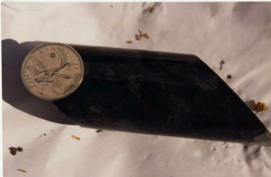
Plate 1: Lapilli tuff, sample from drill core. This is the lowermost unit in the DF-zone stratigraphy, and has a significant mafic component.
