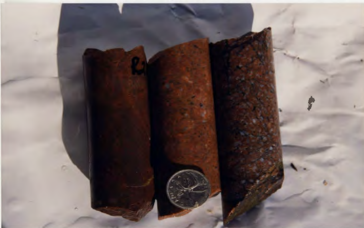
Plate 12: Drill core specimens of the Hart Lake Granite illustrating the transition from granophyric through fine grained to medium grained (from left to right) moving progressively away from the contact with the Byers Brook Formation.
