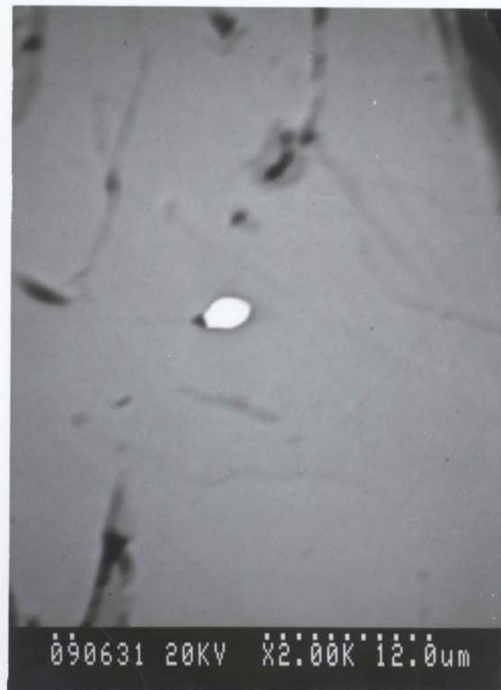
Figure 8.11 Scanning electron photomicrographs of gold with its host minerals. (a) Anhedral gold occurs at the boundary between a silicate xenolith and the pyrrhotite (TL13-98A). (b) An oval inclusion of gold occurring in pentlandite (TL13-63A).
