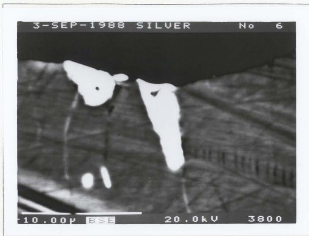
Figure 7.3 Scanning electron photomicrograph of the precious metal minerals and their host minerals in Sample 91-ZC-15. (a) froodite, (b) gold, and (c) silver
