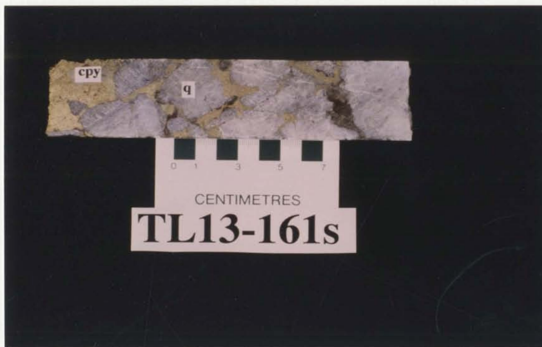
Figure 8.3 Photographs of the drill cores and hand specimens illustrating the ore textures at Thayer Lindsley Mine. (a) and (b): Typical Thayer Lindsley ores, massive pyrrhotite with disseminated chalcopyrite. (c): Sharp contact between massive pyrrhotite and massive chalcopyrite. (d): Melange ore. (e) and (f): Streaky chalcopyrite veins in massive pyrrhotite ores. (g) and (h): Silicate xenoliths in massive sulphide ores. Mineral zoning is displayed around the xenolith. Away from the xenoliths mineral assemblages change from massive chalcopyrite, through chalcopyrite and pentlandite, to massive pyrrhotite. (i): Typical Sublayer rocks. (j): Typical Sublayer ores. (k): Chalcopyrite and quartz vein at the orebody margin of the 4B Ore Zone
