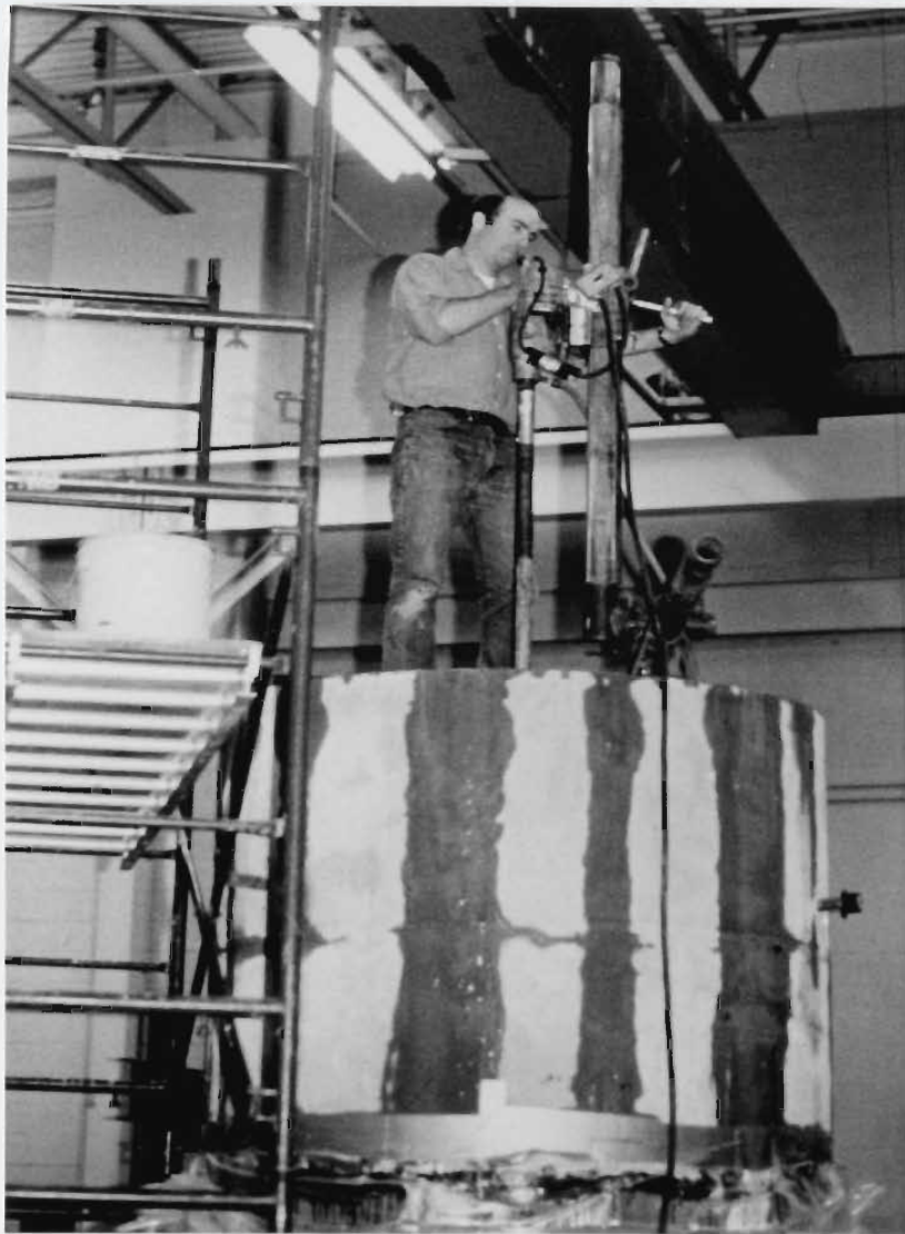
Figure E5 Drilling wellbore in concrete cylinder
